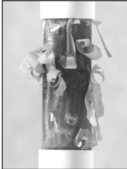
Fig 2. Specimen of E110 cladding that exhibited severe breakaway oxidation after 1400 seconds at 1000°C.
