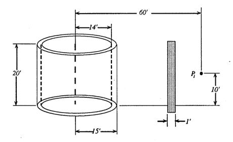
The calculation for dose rate from the cylinder to point  $P_1$  includes buildup based on the Taylor method. See Appendix A for results of the analysis.
