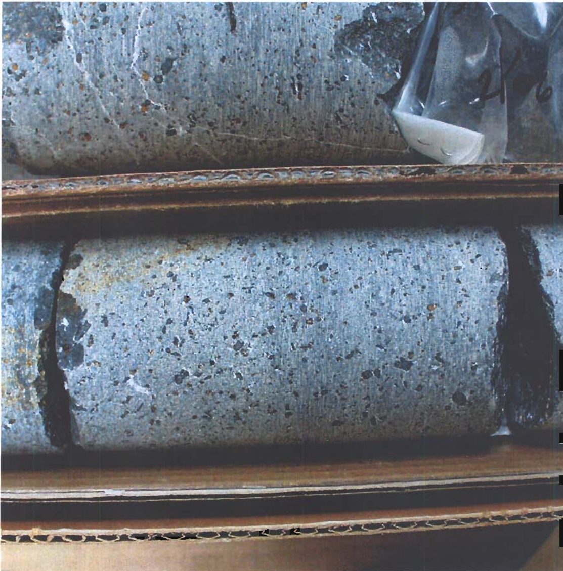
Figure 6. Photograph of core of hornblende-olivine basalt of anomaly G. Diameter of core is 2.25 inches. Dark gray crystals are amphibole, rust-colored crystals are altered olivine.
