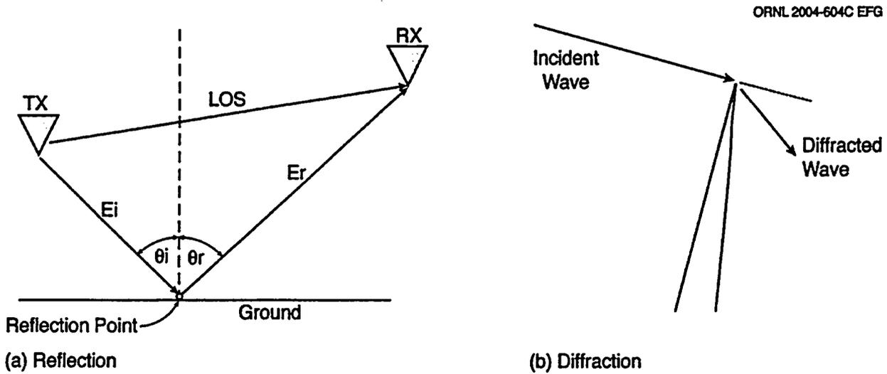
Figure 4.1. Reflection and diffraction.
