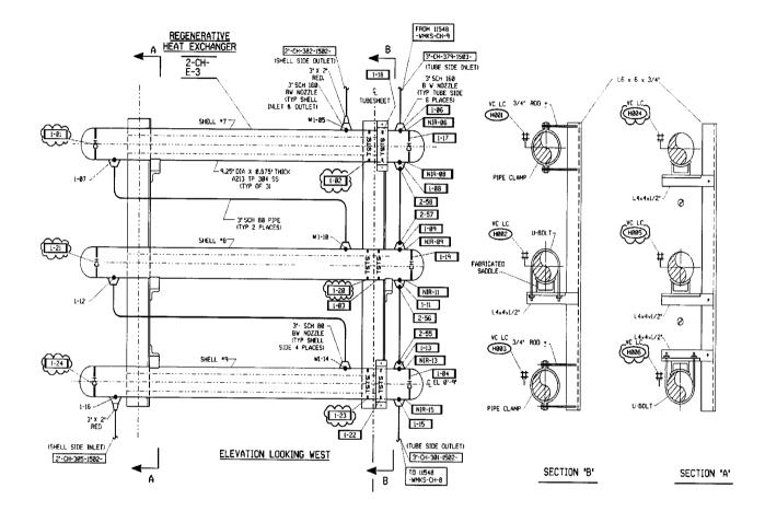
Figure 3 Regenerative Heat Exchanger
