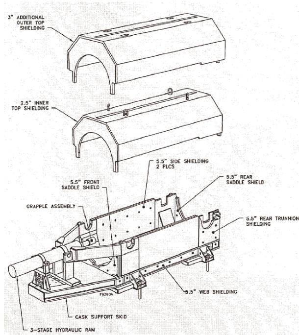
**Figure 2** - Supplemental Shielding on Transfer Trailer
