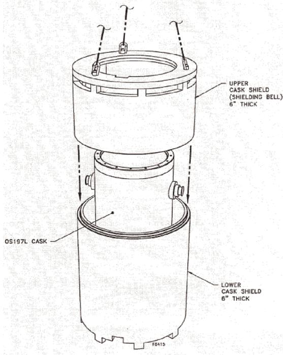
**Figure 1** - Supplemental Shielding in Decontamination Area
