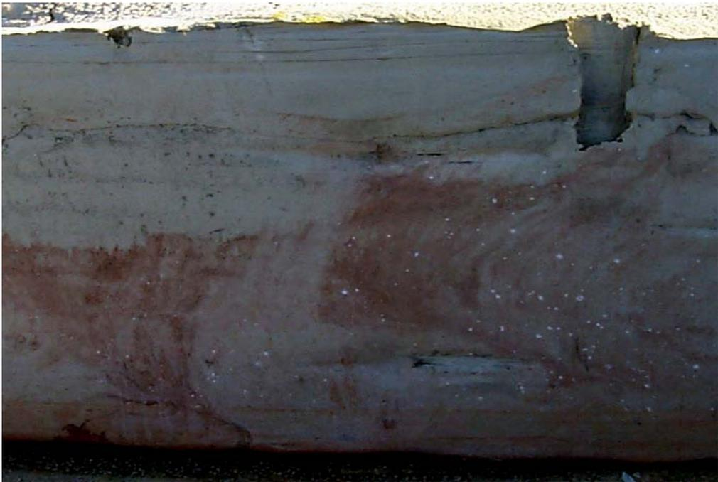
Figure RAI-17-A-2. Vertical mixing near the tank wall.
