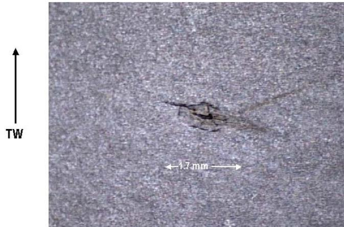
**Figure 1 Small Flaw in Plate Material**
