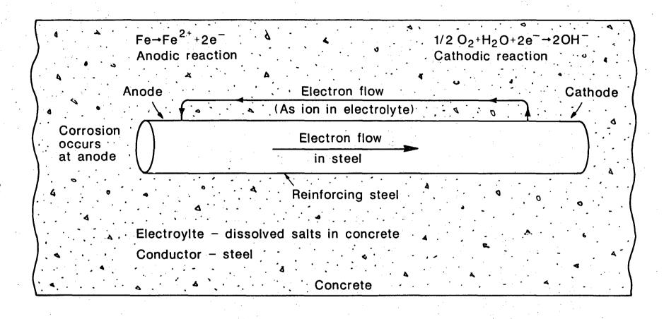
Figure 6. Schematic of corrosion of steel reinforcement in concrete.
