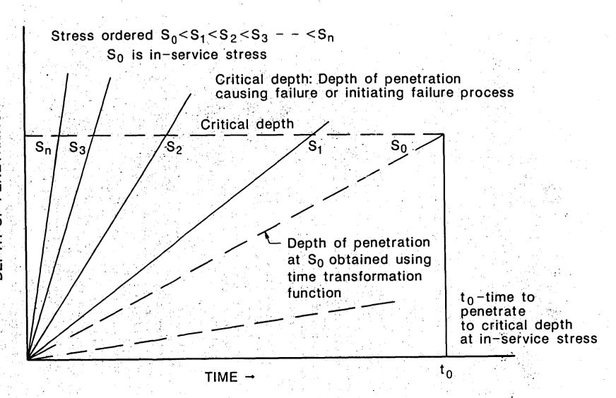
Figure 15. Method for predicting the advance of threshold concentration of aggressive solution concrete at in-service stresses,  $S_{\rm o}$ , based on elevated stresses,  $S_{\rm m}$ .
