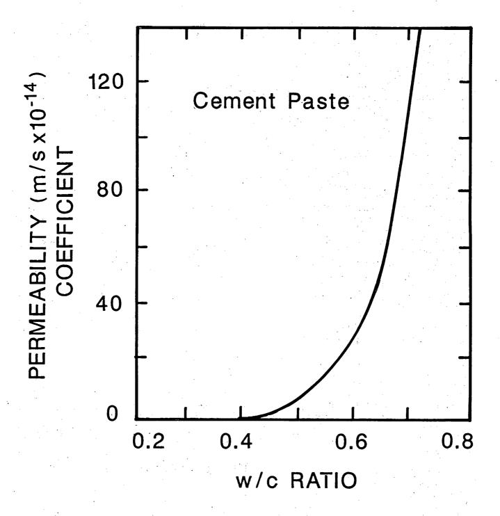
Figure 4. Effect of water-to-cement (w/c) ratio on permeability of hardened cement paste (19).
