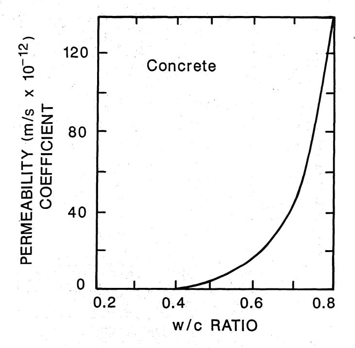
Figure 3. Effect of water-to-cement (w/c) ratio on permeability of concrete (14).
