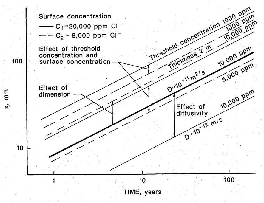
Figure 9. Calculated induction period. Effects of concrete cover, threshold concentration, threshold concentration of chloride ions, concentration of chloride ions, and concrete permeability on calculated induction period (37).
