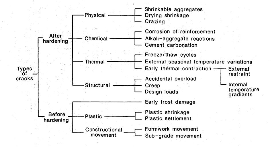
Figure 5. Major causes of cracks in concrete (22).
