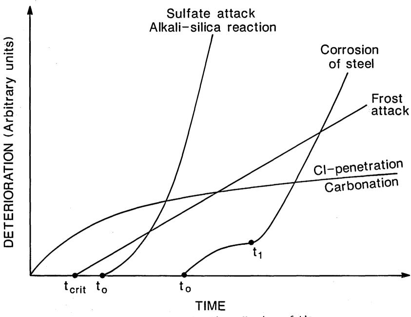
Figure 12. Typical rates of deterioration. Meanings of t's are given in table 5.
