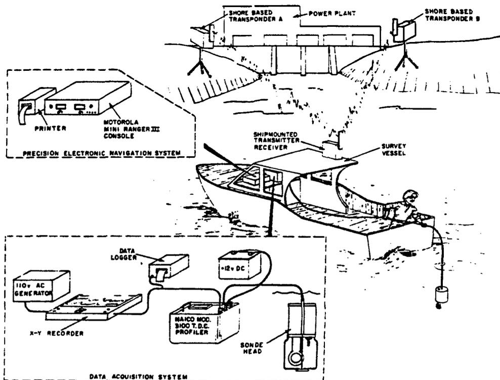
Fig. 2 Instrumentation set up for field surveys.
