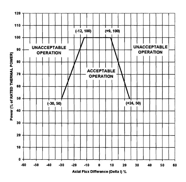
Figure 3 Axial Flux Difference Limits as a Function of Rated Thermal Power for RAOC
