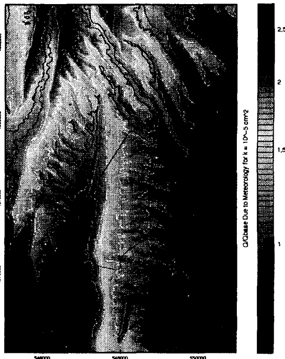
Figure 5: Ratio of infiltration to base-case infiltration due to variation of meteorological factors, assuming uniform coverage of semi-infinite low-permeability alluvium.
