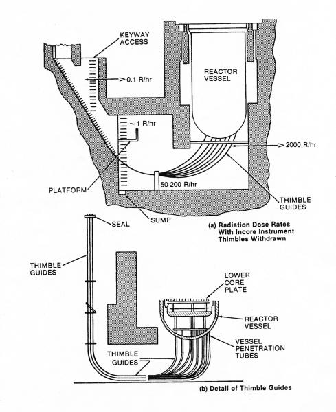
Figure B-1 Pressurized Water Reactor Cavity
