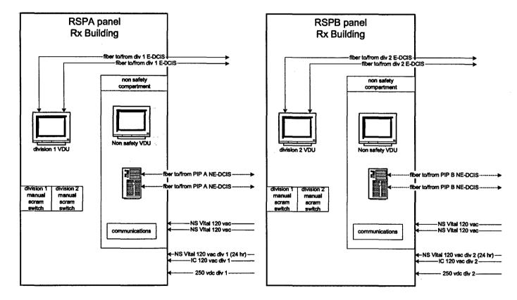
Figure ZZ ESBWR DCIS Remote Shutdown Panels
