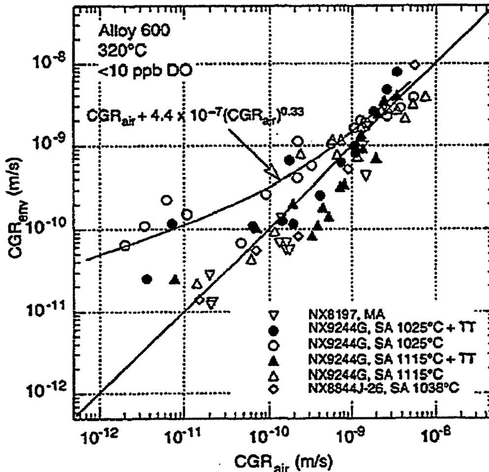
Figure 6-1 Fatigue Crack Growth Model Development for Water Environment
