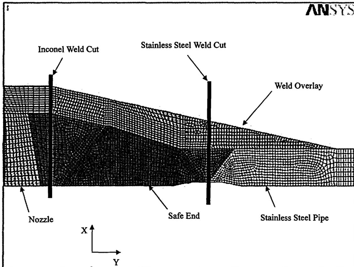
**Figure 5-3 Limiting Sections of Safety Nozzle Weld Overlay (Stress Paths for Figure 5-4 through 5-7)**
