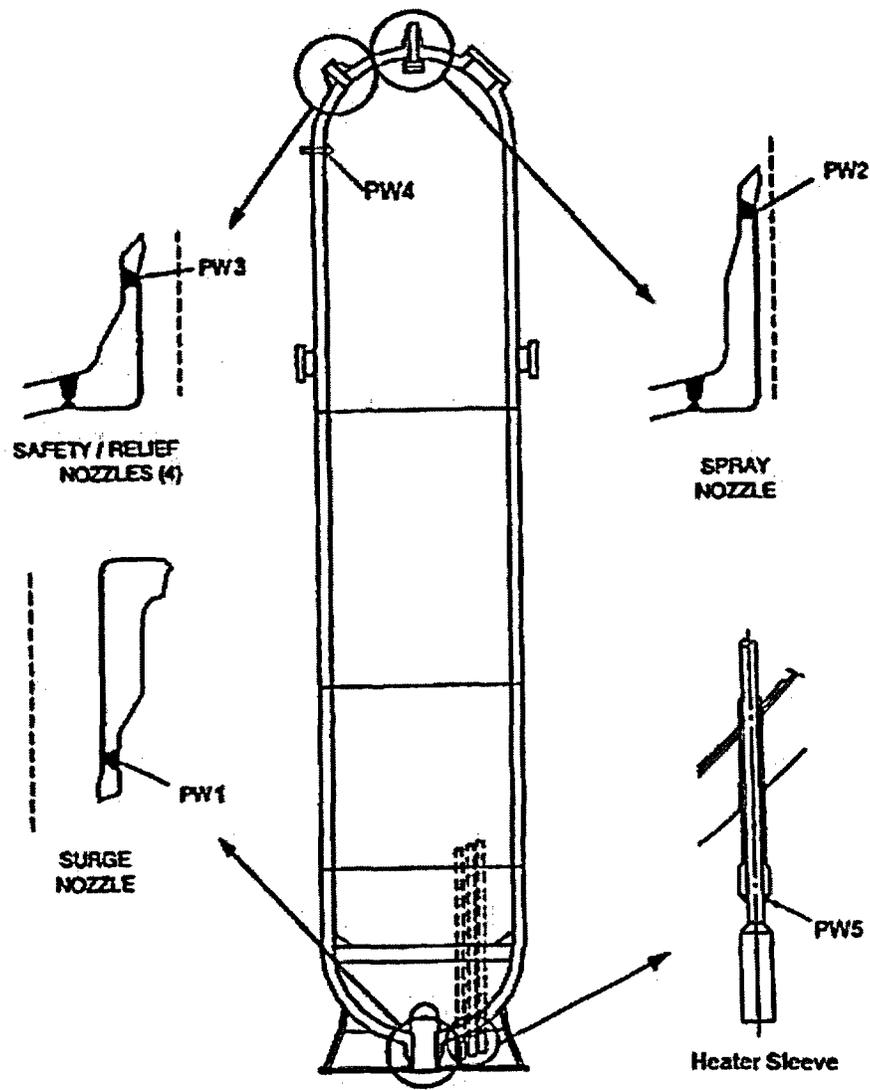
Figure 2-1 Westinghouse Pressurizer Configuration
