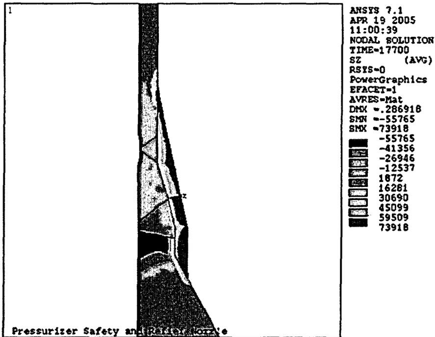
Figure 5-9 Hoop Residual Stress Contour Plot at Ambient Conditions
