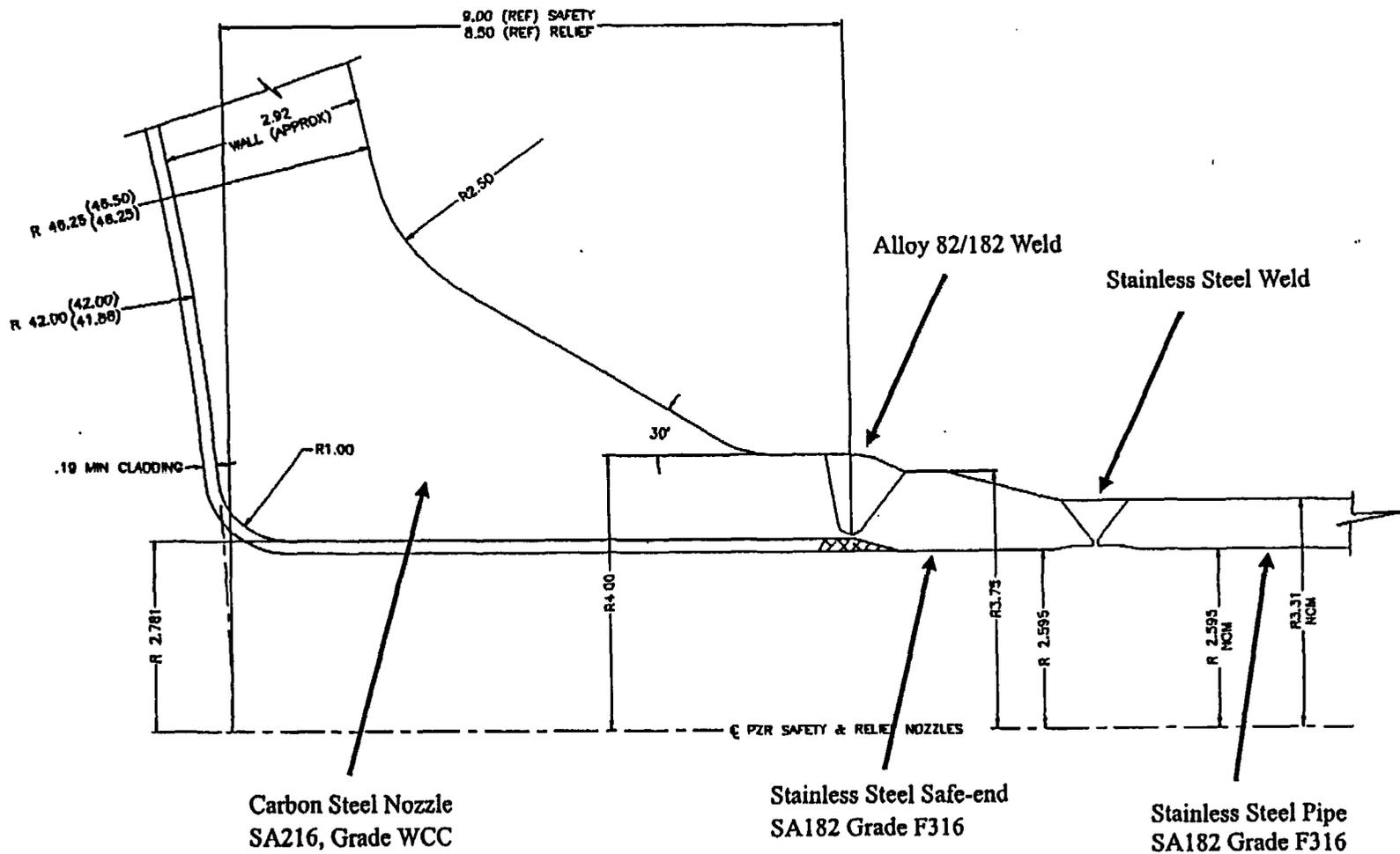
**Pressurizer Safety Nozzle Geometry for the Cast Head Configuration**
