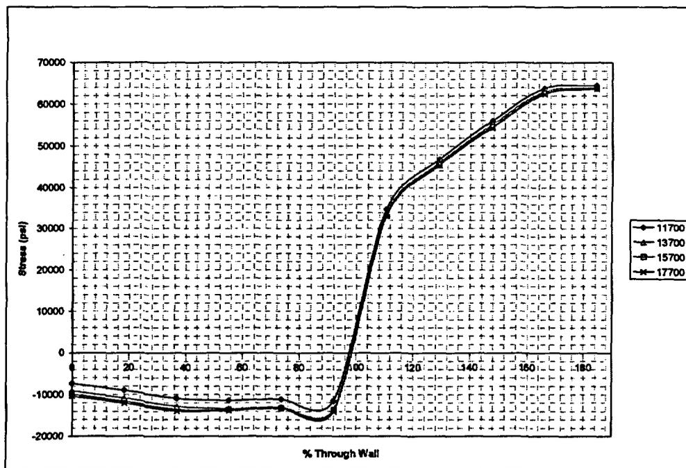
Figure 5-7\* Hoop Through-Wall Residual Stress Distribution at Stainless Steel Weld Location
