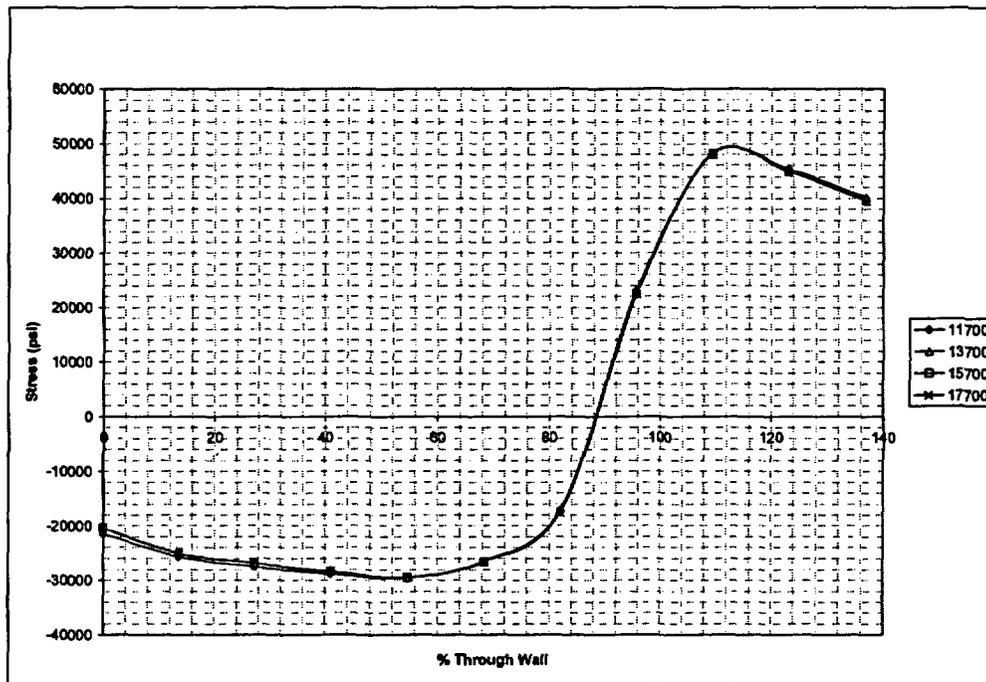
Figure 5-4\* Axial Through-Wall Residual Stress Distribution at Alloy 82/182 Weld Location
