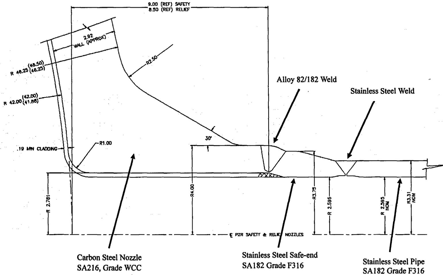
Figure 2-2 Pressurizer Safety Nozzle Geometry for the Cast Head Configuration
