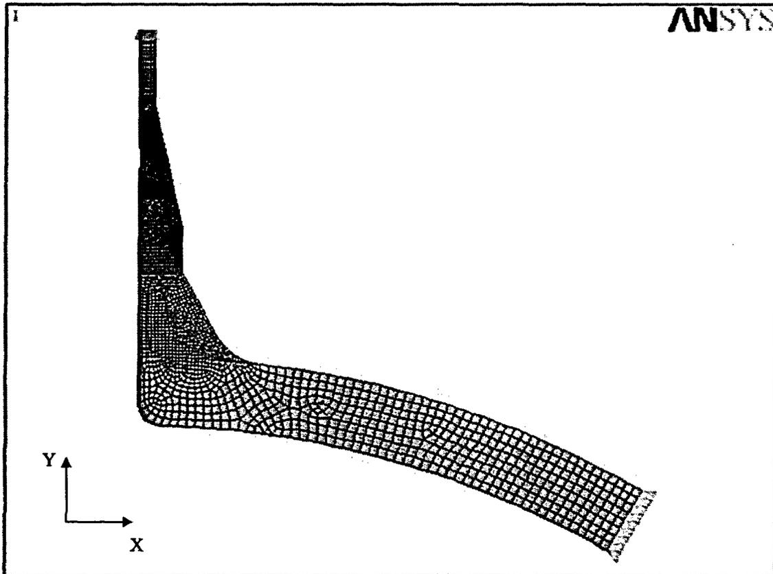
**Figure 5-1 Axisymmetric Finite Element Model Used for Safety Nozzle Weld Overlay Analysis**
