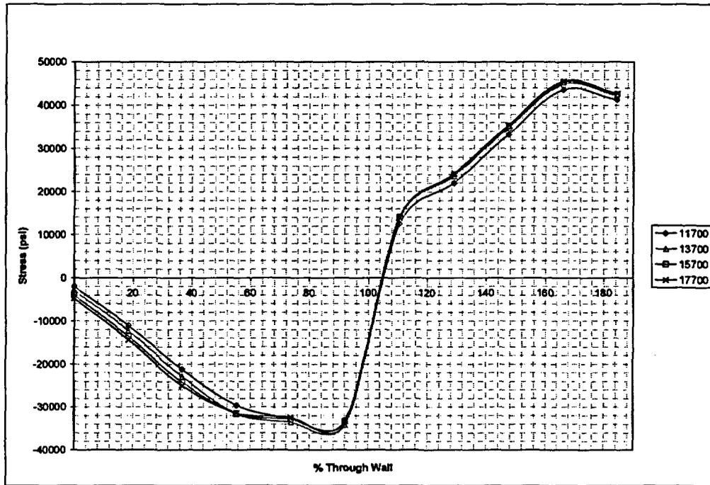
Figure 5-6\* Axial Through-Wall Residual Stress Distribution at Stainless Steel Weld Location
