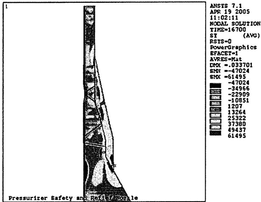
Figure 5-10 Axial Residual Stress Contour Plot at Operational Conditions
