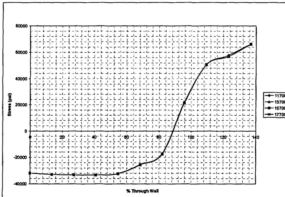
Figure 5-5\* Hoop-Through Wall Residual Stress Distribution at Alloy 82/182 Weld Location
