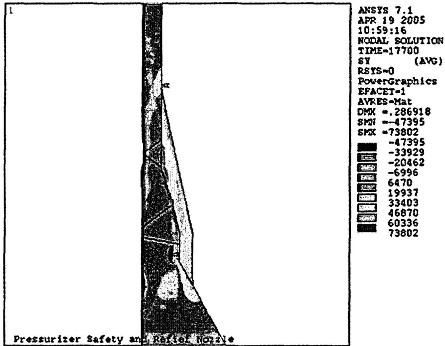
Figure 5-8 Axial Residual Stress Contour Plot at Ambient Conditions
