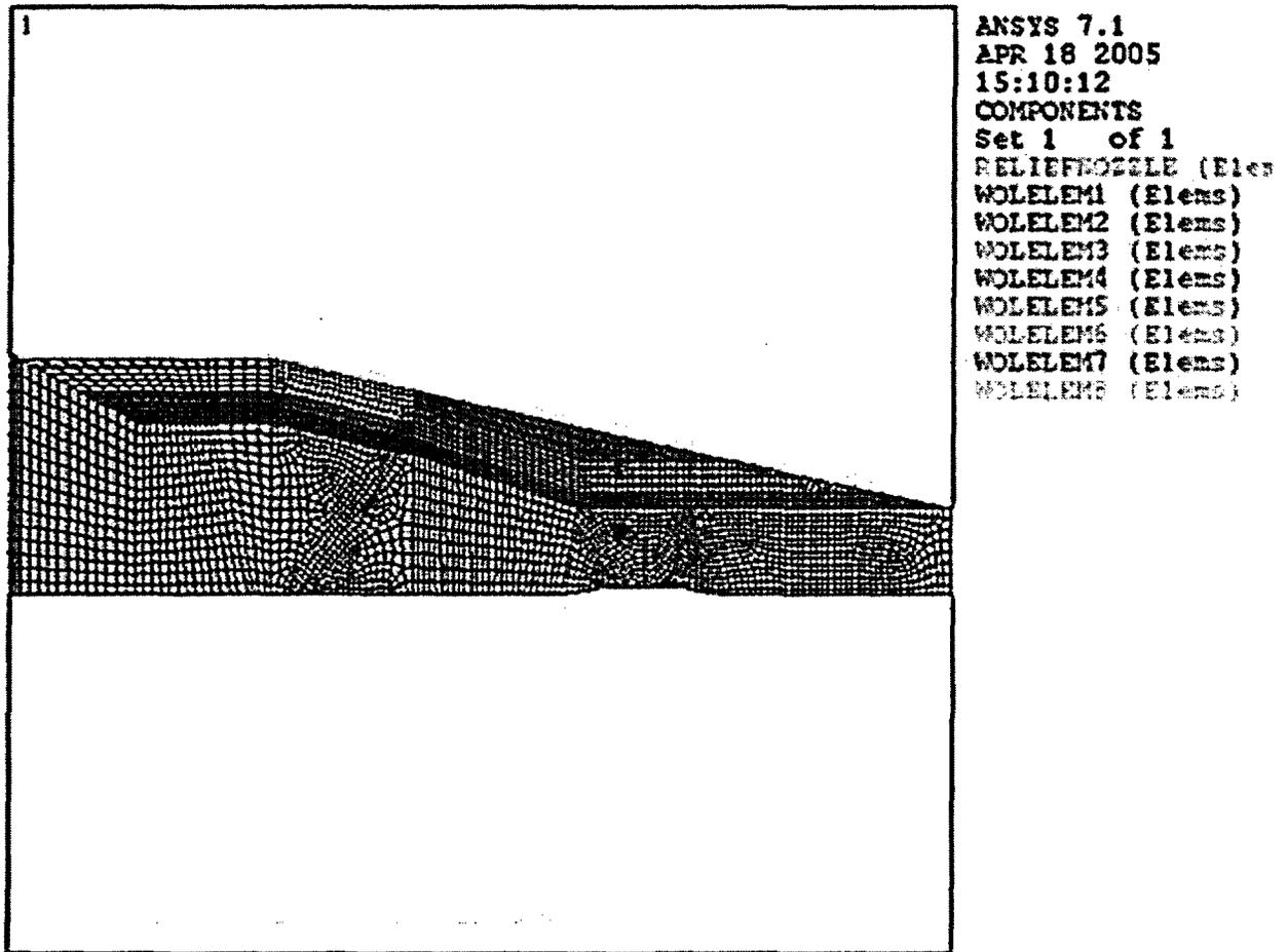
**Figure 5-2 Model of Weld Overlay Segments for the Safety Nozzle Weld Overlay Stress Analysis**
