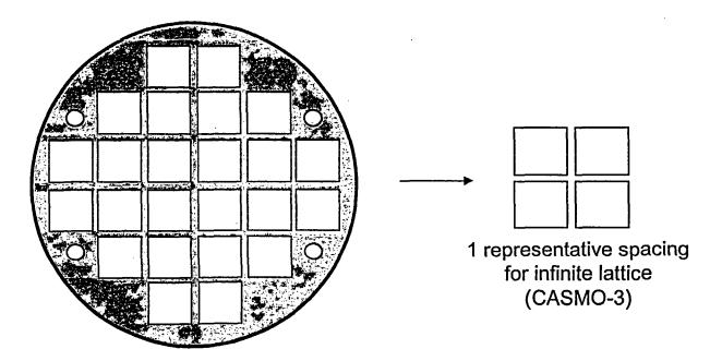
3 different fuel assembly spacings (KENO V.a)
