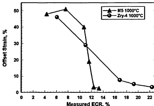
Fig. 1. Deformation versus oxidation at 1000°C for unirradiated M5 and Zircaloy cladding.
