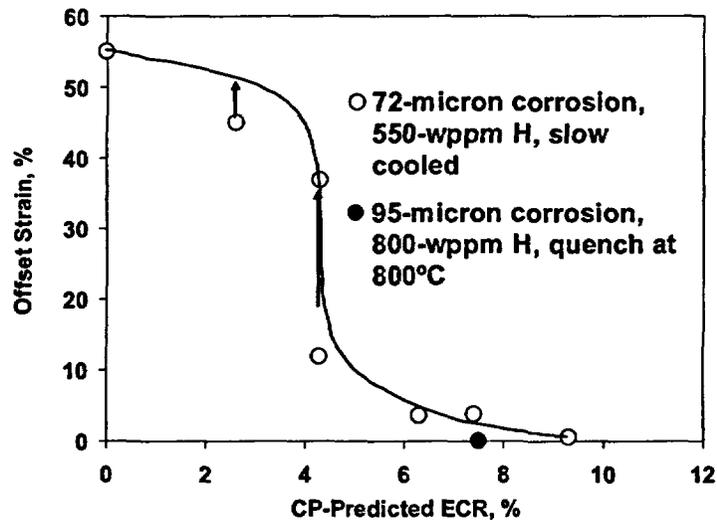
Fig. 4. Deformation versus oxidation at 1200°C for irradiated 15x15 Zircaloy (rough surface). CP-predicted oxidation is the same as measured oxidation at this temperature.
