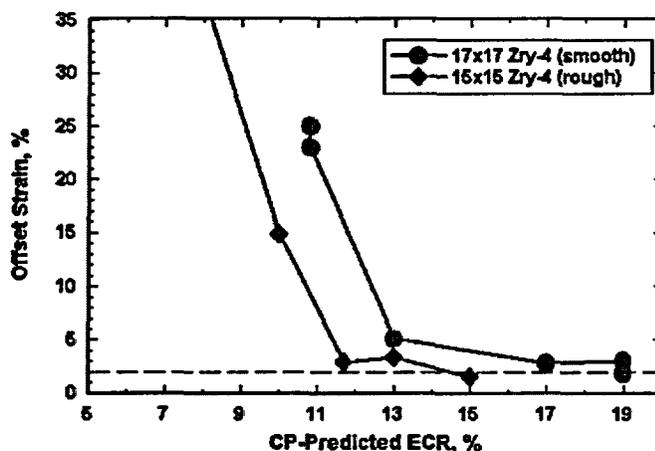
Fig. 2. Deformation versus oxidation at 1200°C for unirradiated Zircaloy (CP-Predicted same as Measured at this temperature).
