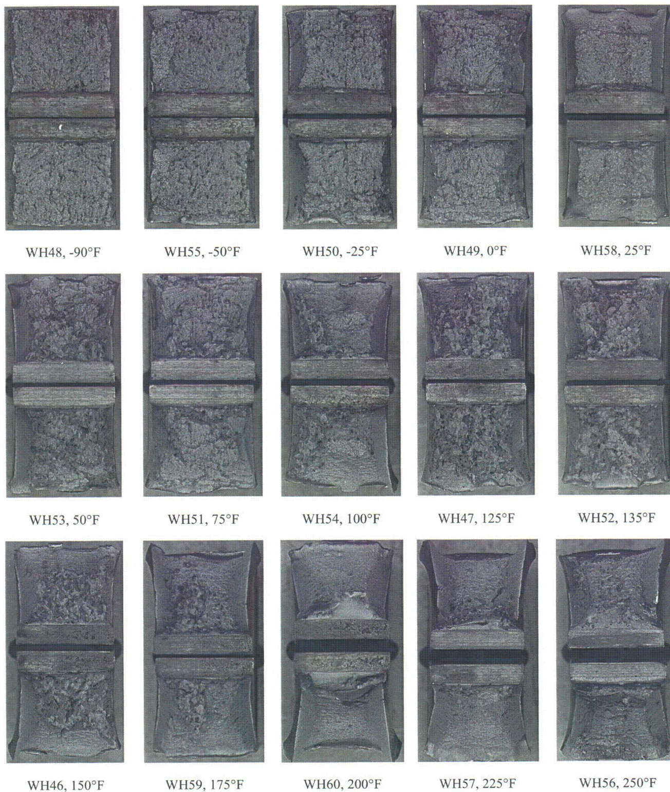
Figure 5-16 Charpy Impact Specimen Fracture Surfaces for Beaver Valley Unit 2 Reactor Vessel Heat Affected Zone Material
