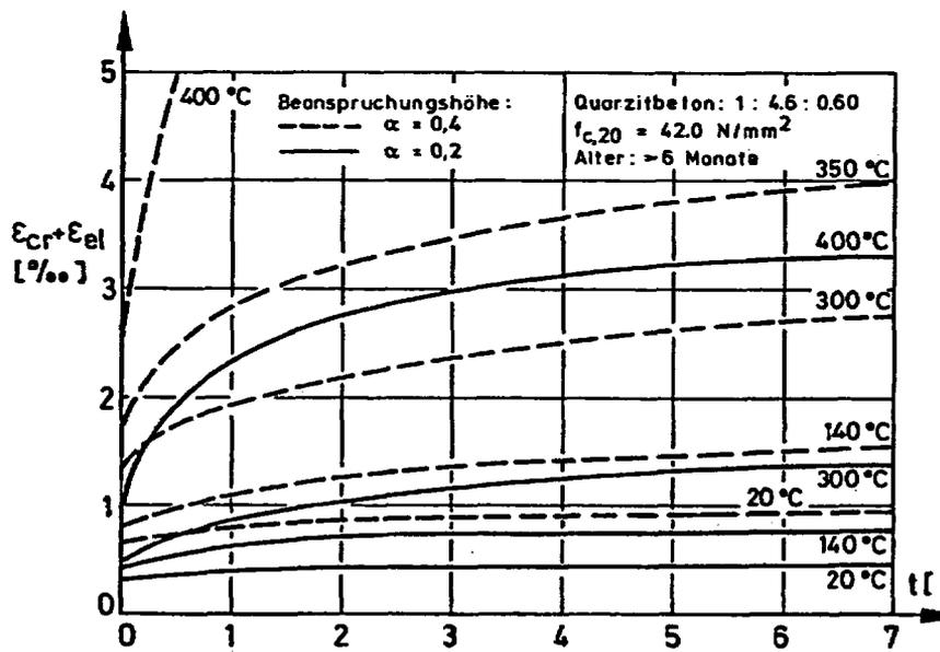
**Figure 52** Influence of load level and temperature on the creep of normal concrete. *Source:* H. Gross, "On High Temperature Creep of Concrete," Paper H6/5 in *Proc. 2nd International Conference on Structural Mechanics in Reactor Technology*, Elsevier Science Publishers, North-Holland, The Netherlands, 1973.
