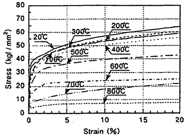
**Figure 8** Stress-strain relationships of reinforcing bars at elevated temperature. *Source:* M. Takeuchi et al., "Material Properties of Concrete and Steel Bars at Elevated Temperatures," *12th International Conference on Structural Mechanics in Reactor Technology*, Paper H04/4, pp. 133-138, Elsevier Science Publishers, North-Holland, The Netherlands, 1993.
