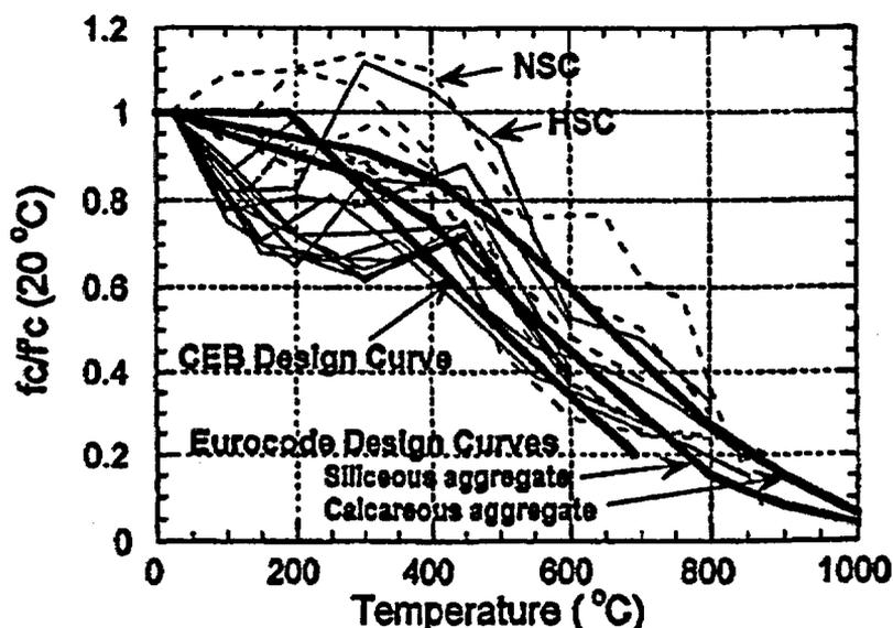
Figure 105 Comparison of unstressed NSC and HSC results with the CEB and Eurocode Design curves. Source: G. L. T. Phan, *Fire Performance of High-Strength Concrete: A Report of the State-of-the-Art*, NISTIR 5934, National Institute of Standards and Technology, Gaithersburg, Maryland, 1996.
