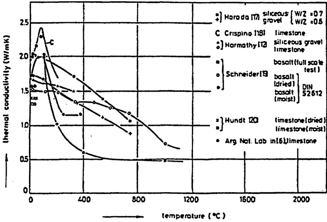
Figure 86 Thermal conductivity of ordinary concretes with different aggregates. Source: U. Schneider, C. Diererichs, and C. Ehm, "Effect of Temperature on Steel and Concrete for PCRV's," *Nuclear Engineering and Design* 67, 245-258 (1981).
