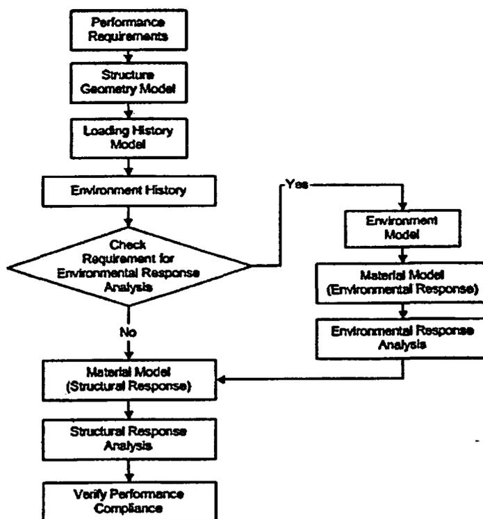
**Figure 120** Design process flow diagram. *Source:* B. Bresler and R. H. Iding, "Effects of Normal and Extreme Environment on Reinforced Concrete Structures," Paper SP 55-11 in *Douglas McHenry Symposium on Concrete and Concrete Structures*, SP 55, American Concrete Institute, Farmington Hills, Michigan, April 1970.
