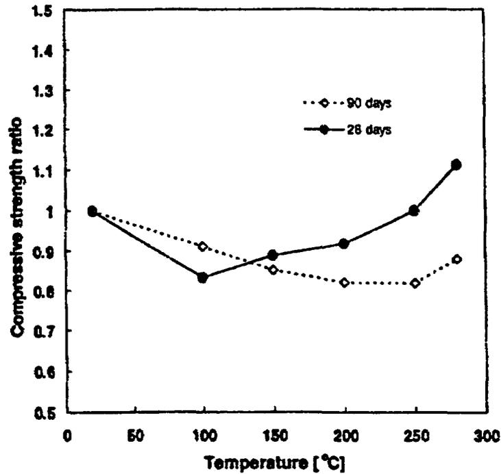
Figure 31 Effect of temperature on compressive strength ratio of concrete. Source: F. Vodak et al., "The Effect of Temperature on Strength—Porosity Relationship for Concrete," *Construction and Building Materials* 18, 529-534 (2004).
