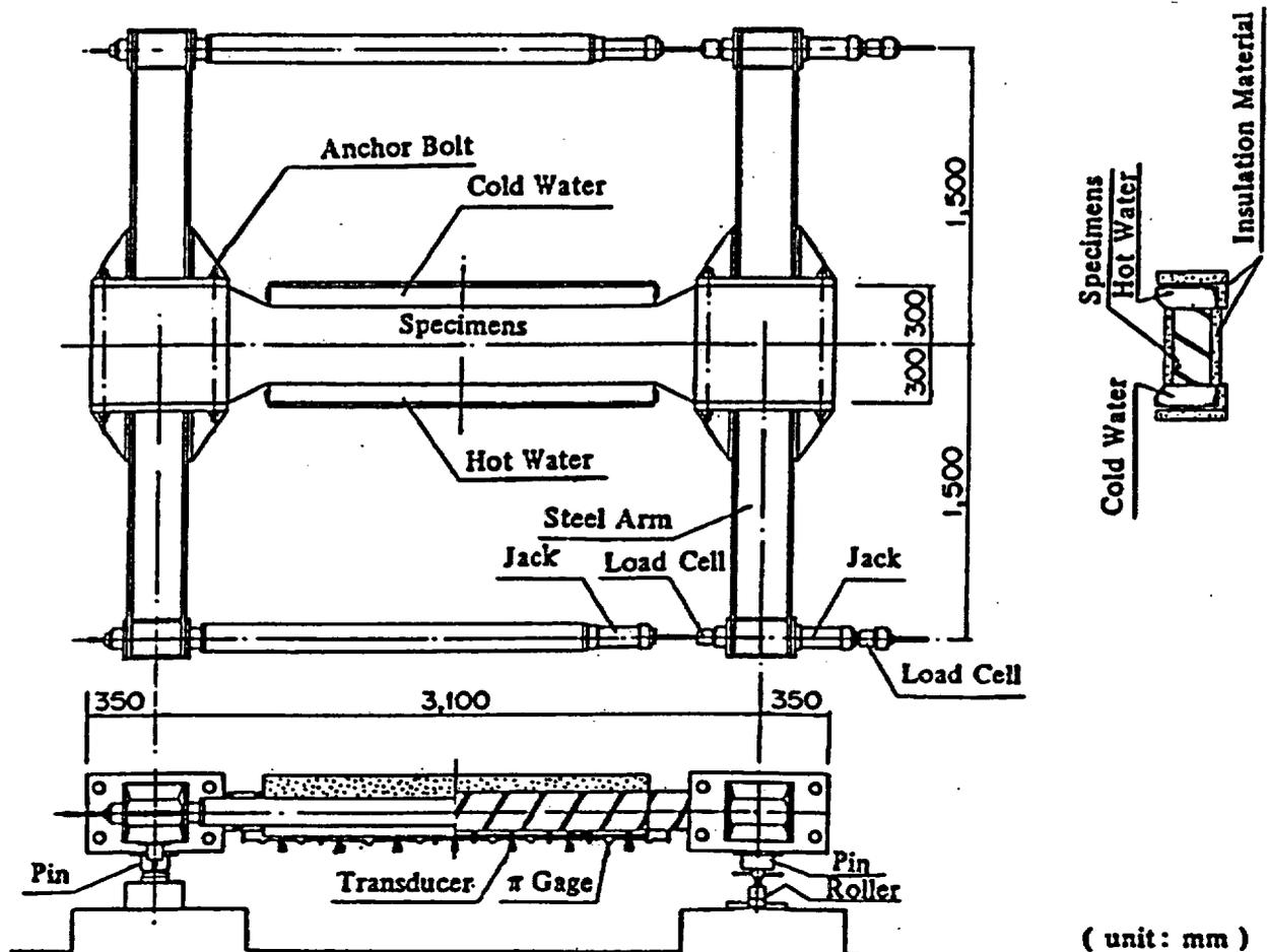
Figure 143 Apparatus used to test specimen shown in Fig. 142. Source: N. Shibasaki et al., "An Experimental Study on Thermal Stress of Reinforced Concrete Members Under Short-Term Loading," Paper J4/3, Vol. J, *Trans. of 7th Ind. Conf. on St. Mech. in Reactor Technology*, pp. 189-197, Chicago, Illinois, August 22-26, 1983.
