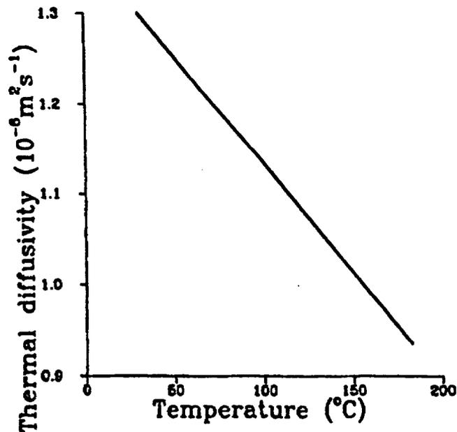
Figure 92 Temperature dependence of thermal diffusivity of a nuclear power plant concrete. Source: F. Vodak et al., "The Effect of Temperature on Strength—Porosity Relationship for Concrete," *Construction and Building Materials* 18, 529–534 (2004).
