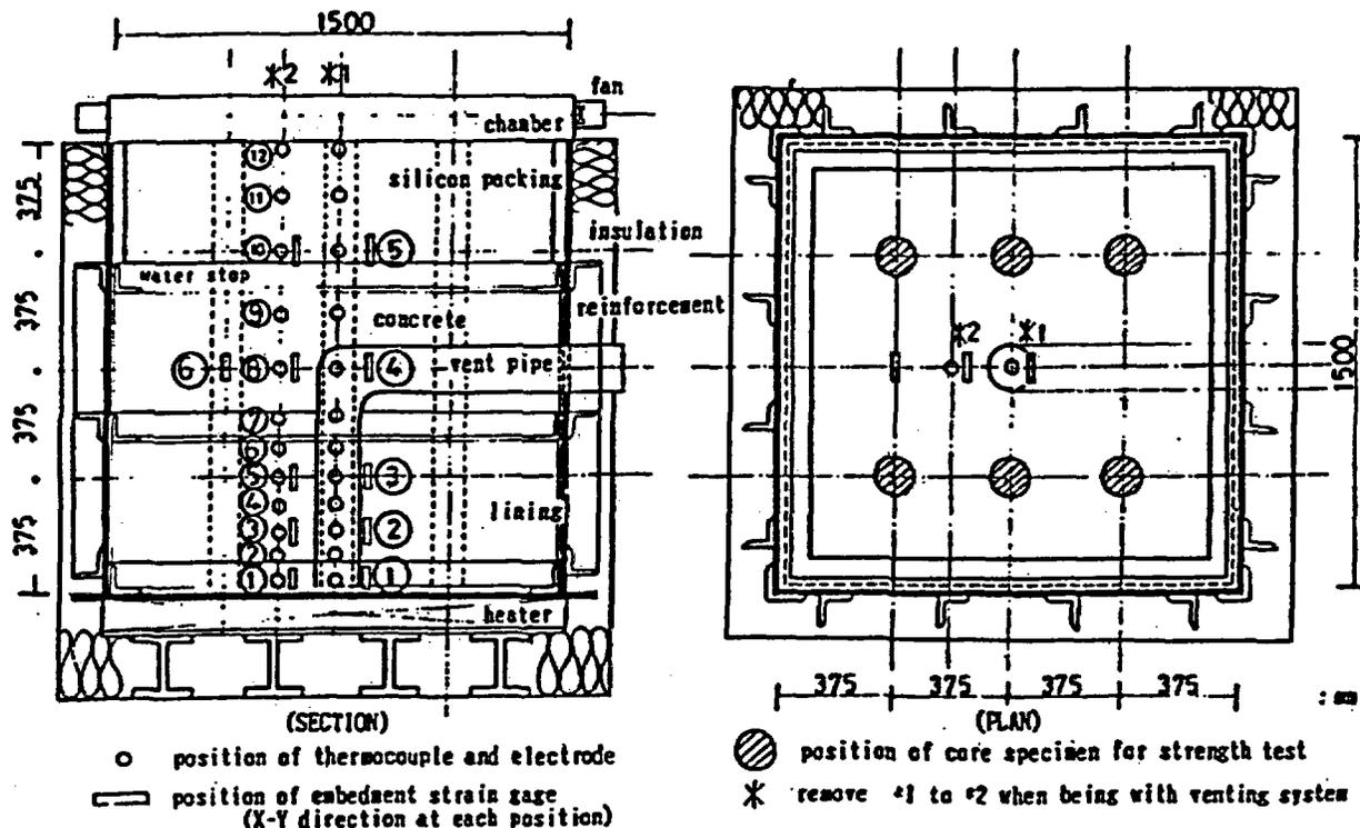
**Figure 127** Details of simulated section of mass concrete wall and measurement positions. Source: T. Takeda et al., "Experimental Studies on Characteristics of Concrete Members Subjected to High Temperature," Vol. H, *Trans. of 9th Intl. Conf. on St. Mech. in Reactor Technology*, pp. 195-200, Lausanne, Switzerland, August 17-21, 1987.
