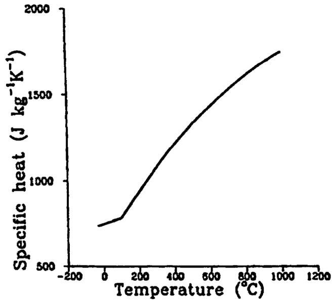
**Figure 97** Temperature dependence of specific heat of a nuclear power plant concrete. *Source:* F. Vodak et al., "The Effect of Temperature on Strength—Porosity Relationship for Concrete," *Construction and Building Materials* 18, 529–534 (2004).
