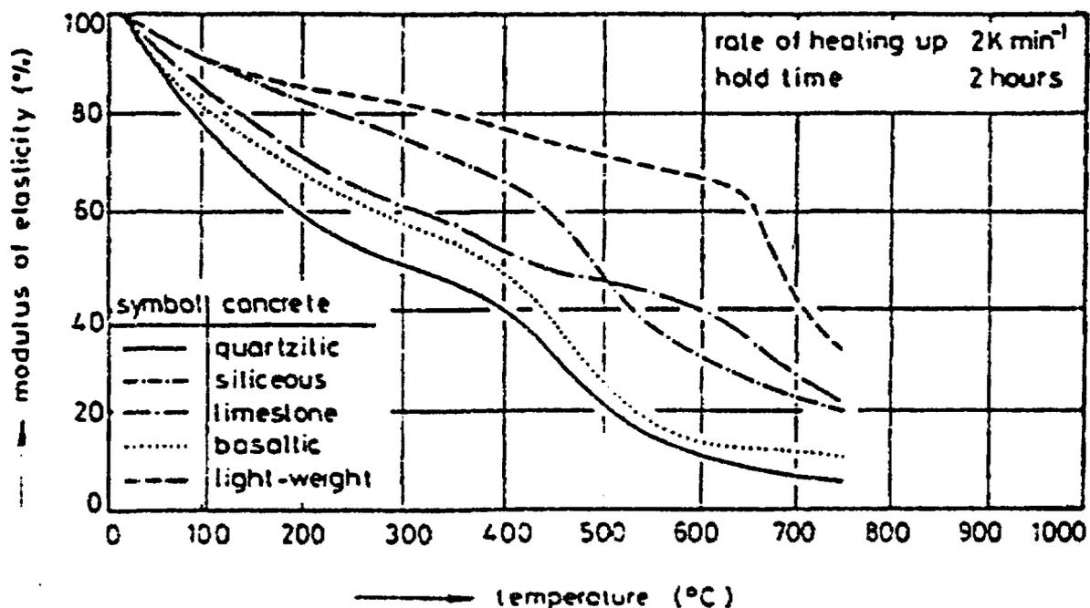
Figure 19 Modulus of elasticity of different concretes at elevated temperature. Source: U. Schneider, C. Diererichs, and C. Ehm, "Effect of Temperature on Steel and Concrete for PCRV's," *Nuclear Engineering and Design* 67, 245-258 (1981).
