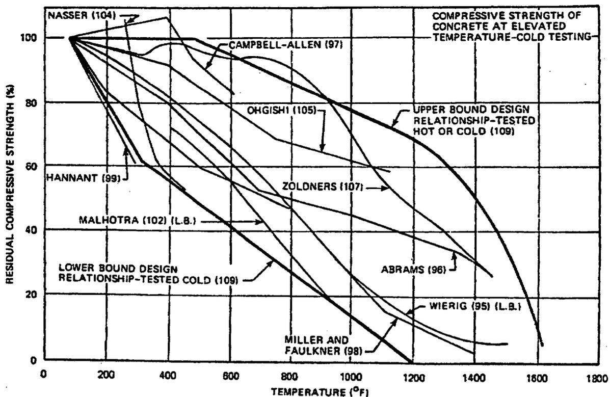
Figure 22 Effect of temperature exposure on compressive strength of concrete: tested cold. Source: G. N. Freskakis et al., "Strength Properties of Concrete at Elevated Temperature," *Civil Engineering Nuclear Power*, Vol. 1, ASCE National Convention, American Society of Civil Engineers, Boston, Massachusetts, April 1979.
