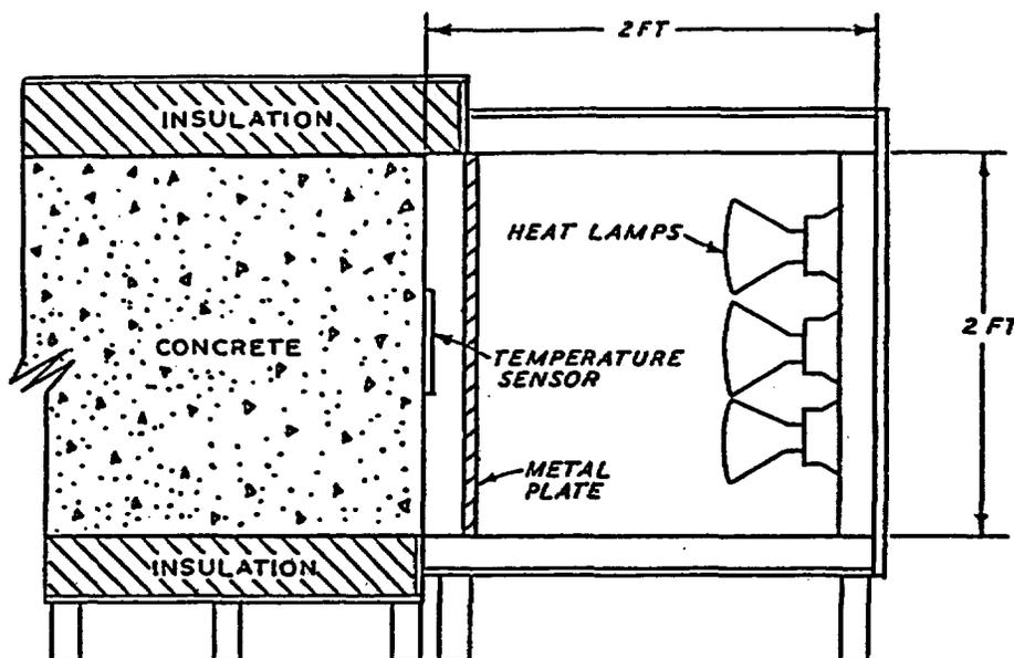
**Figure 164** Heating arrangement for moisture migration test conducted at Waterways Experiment Station. Source: J. E. McDonald, *Moisture Migration in Concrete*, Technical Report C-75-1, U.S. Army Waterways Experiment Station, Vicksburg, Mississippi, May 1975.
