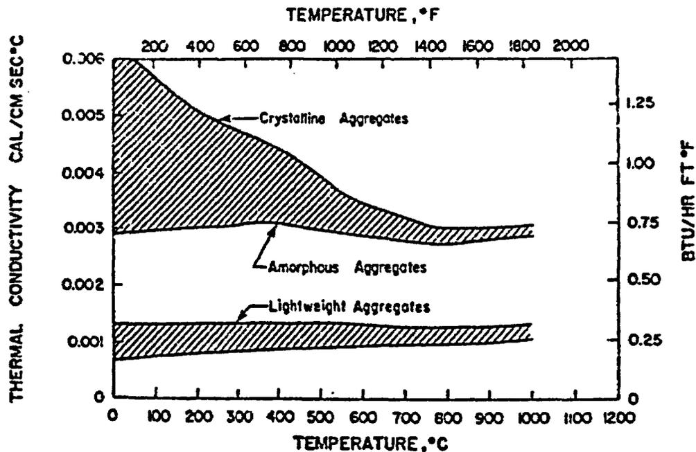
Figure 85 Thermal conductivity of Portland cement concretes. Source: T. Z. Harmathy and L.W. Allen, "Thermal Properties of Selected Masonry Unit Concretes," *J. American Concrete Institute* 70, 132-142 (1973).
