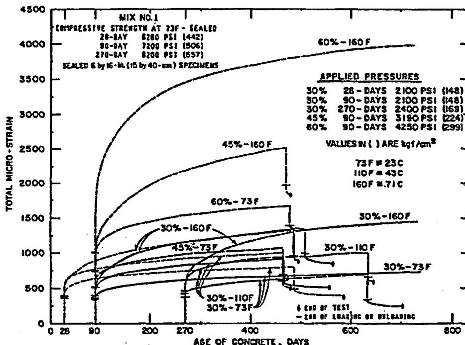
Figure 51 Total strains for a number of test parameters. Source: J. Komendant et al., "Effects of Temperature, Stress Level, and Age at Loading on Creep of Sealed Concrete," Paper SP 55-3 in *Douglas McHenry International Symposium on Concrete and Concrete Structures*, American Concrete Institute, Farmington Hills, Michigan, 1978.
