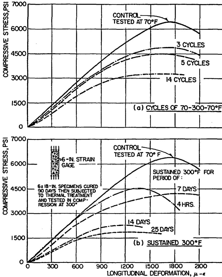
**Figure 39** Influence of thermal cycling on  $\sigma$ - $\epsilon$  response of sealed concrete tested at 300°F (149°C). Source: V. V. Bertero and M. Polivka, "Influence of Thermal Exposures on Mechanical Characteristics of Concrete," Paper SP 34-28 in Special Publication 34, Vol. I-III, American Concrete Institute, Farmington Hills, Michigan, 1972.
