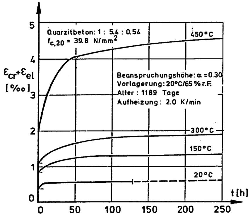
**Figure 53** High-temperature creep of ordinary concrete with quartz aggregate.
