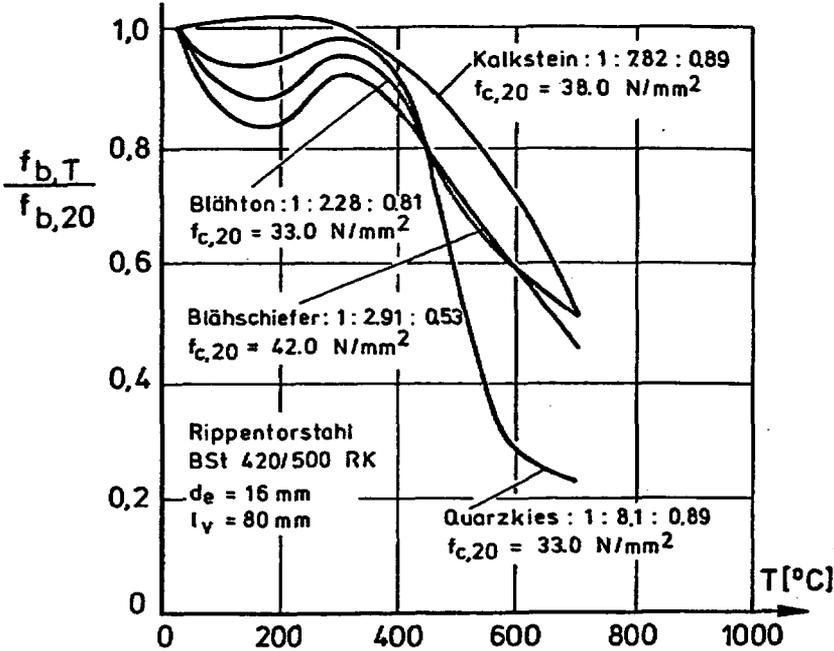
Figure 60 Bond between concrete and deformed bars exposed to high temperature. Source: H. Sager et al., "High Temperature Behavior of Reinforcing and Prestressing Steels," *Sonderforschungs-Bereich 148*, Part II, pp. 51-53, Technical Universität Braunschweig, Germany, 1980.
