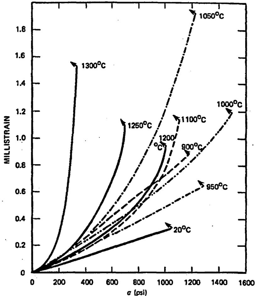
**Figure 102** Effect of temperature on stress-strain behavior of alumina-silicate bricks. *Source:* G. C. Padgett et al., "Stress/Strain Behavior of Refractory Materials at High Temperatures," Research Paper 608, The British Ceramic Association.
