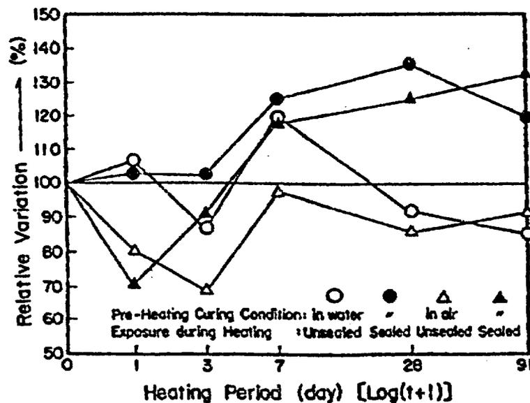
Figure 61 Relative variation in bond strength at start of pull-out for a hard sandstone aggregate concrete after various heating periods at 175°C. Source: K. Hirano et al., "Physical Properties of Concrete Subjected to High Temperature for MONJU," Paper P2-25, Power Reactor and Nuclear Fuel Development Corporation, Tokyo, Japan.
