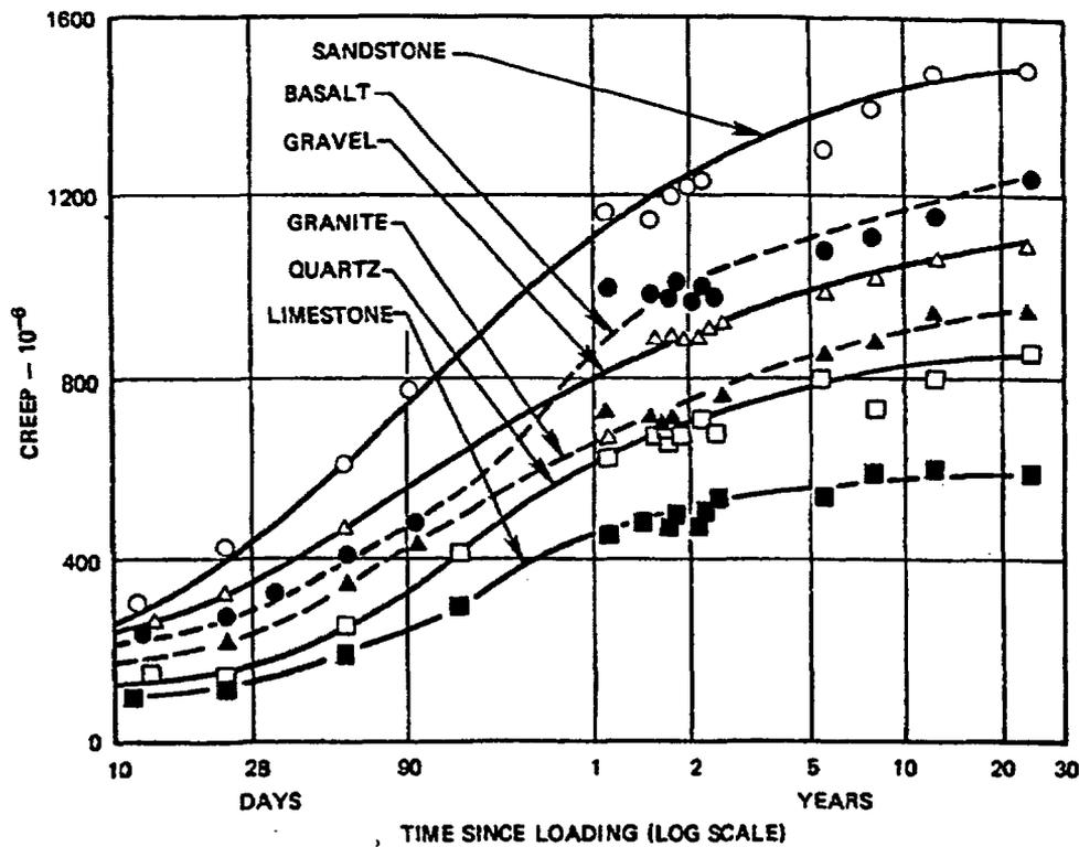
Figure 46 Creep of concrete with different aggregates (aggregate/cement ratio = 5.67, w/c = 0.59, stress = 56 kg/cm<sup>2</sup>). Source: G. E. Troxell et al., *Composition and Properties of Concrete*, 2nd Ed., McGraw-Hill, New York, 1968.
