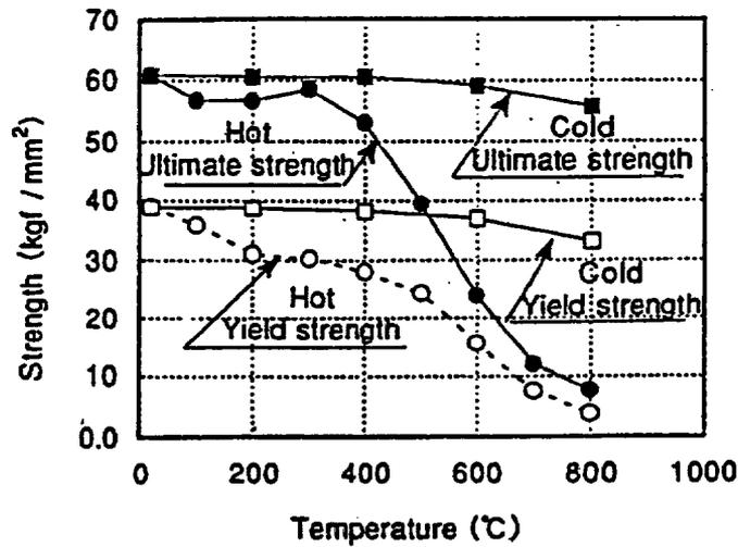
**Figure 10** Yield strength and ultimate tensile strength of reinforcing bars at elevated temperature. *Source:* M. Takeuchi et al., "Material Properties of Concrete and Steel Bars at Elevated Temperatures," *12th International Conference on Structural Mechanics in Reactor Technology*, Paper H04/4, pp. 133-138, Elsevier Science Publishers, North-Holland, The Netherlands, 1993.
