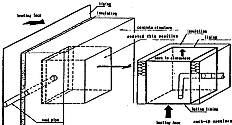
Figure 126 Simulated section of mass concrete wall. Source: T. Takeda et al., "Experimental Studies on Characteristics of Concrete Members Subjected to High Temperature," Vol. H. *Trans. of 9th Intl. Conf. on St. Mech. in Reactor Technology*, pp. 195–200, Lausanne, Switzerland, August 17–21, 1987.
