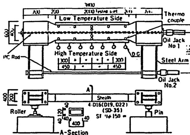
**Figure 121** Test setup for investigating effect of thermal gradients on RC beam performance. Source: K. Irino et al., "Studies on Thermal Stress Design Method for Reinforced Concrete Members of Nuclear Power Plant," Paper J4/5, Vol. J, *Trans. of 7th Ind. Conf. on St. Mech. in Reactor Technology*, pp. 209-219, Chicago, Illinois, August 22-26, 1983.
