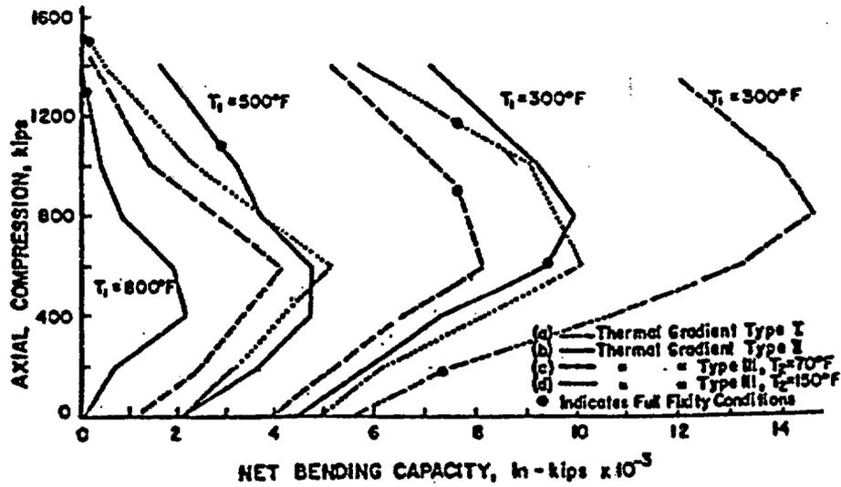
Figure 114 Effect of temperature distribution on net bending capacity. Source: G. N. Freskakis, "Behavior of Reinforced Concrete at Elevated Temperature," Paper 3-4, *Second ASCE Conf. on Civ. Eng. and Nuclear Power*, Vol. 1, Paper 3-5, pp. 3-5-1 to 3-5-21, Knoxville, Tennessee, September.
