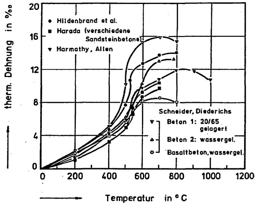
Figure 83 Thermal expansion of siliceous aggregate concretes. Source: U. Schneider, "Behaviour of Concrete at High Temperature," HEFT 337, Deutscher Ausschuss für Stahlbeton, Wilhelm Ernst & Sohn, Munich, Germany, 1982.
