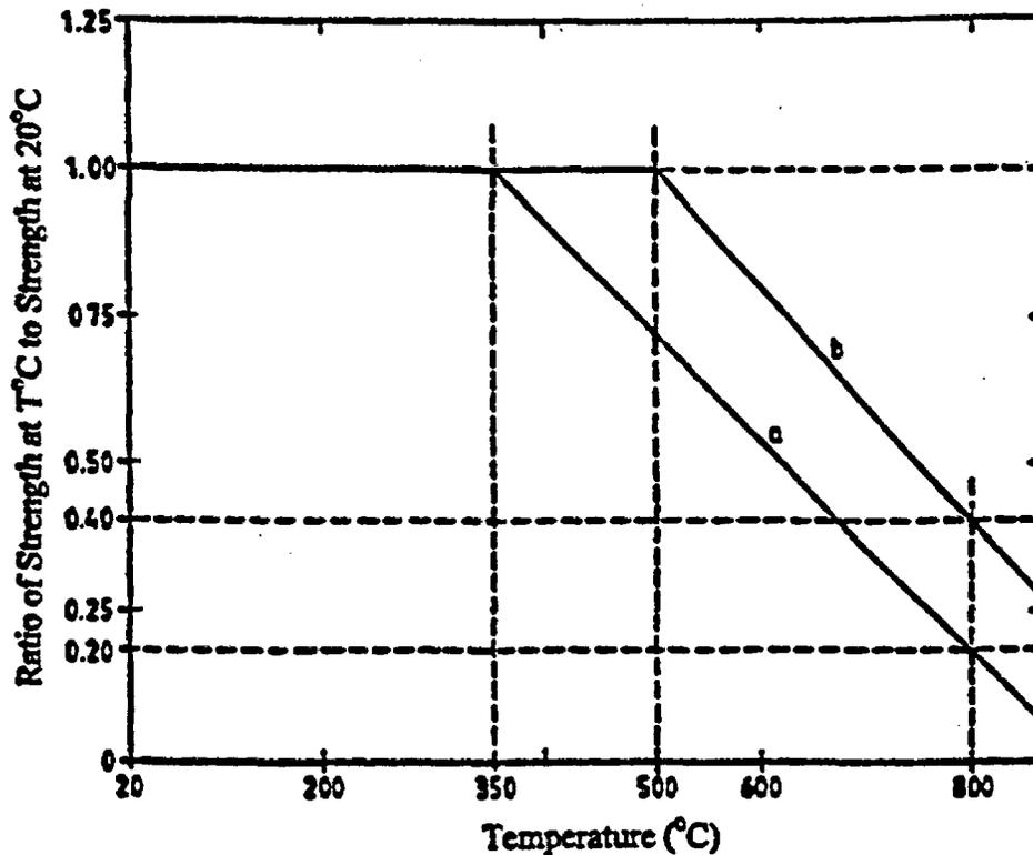
Figure 104 BS8110 design curves for strength variation with the temperature of (a) dense concrete and (b) lightweight concrete. *Source:* "Specification for Prestressed Concrete Pressure Vessels for Nuclear Reactors," BS 4975, British Standards Institution, United Kingdom, July 1973.
