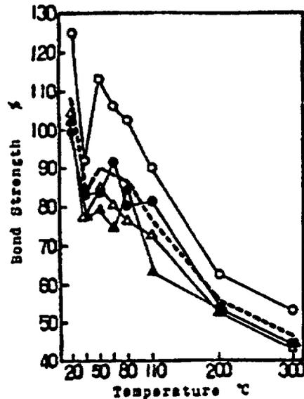
**Figure 70** Bond strengths of heated concretes. *Source:* H. Kasami, T. Okuno, and S. Yamane, "Properties of Concrete Exposed to Sustained Elevated Temperature," Paper HI/5 in *Proc. 3rd International Conference on Structural Mechanics in Reactor Technology*, Elsevier Science Publishers, North-Holland, The Netherlands, 1975.
