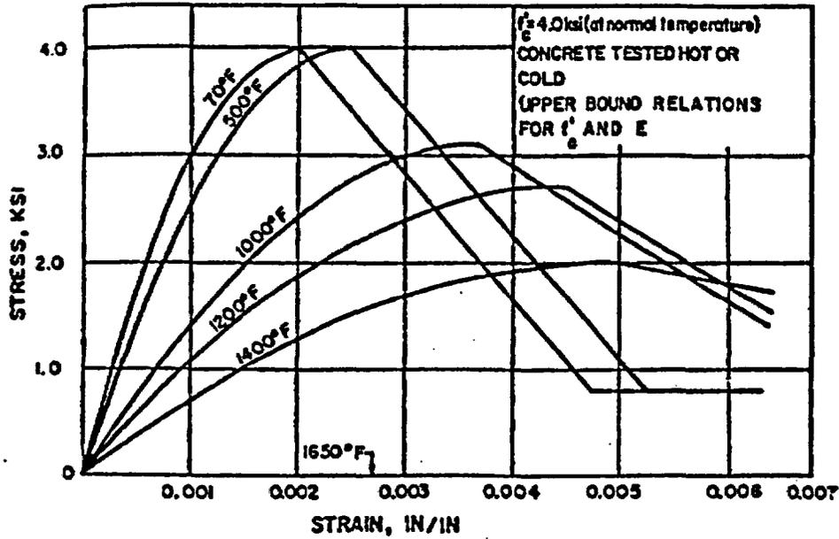
Figure 108 Stress-strain relationships used by Freskakis (upper bound). Source: G. N. Freskakis, "Behavior of Reinforced Concrete at Elevated Temperature," Paper 3-4, *Second ASCE Conf. on Civ. Eng. and Nuclear Power*, Vol. 1, Paper 3-5, pp. 3-5-1 to 3-5-21, Knoxville, Tennessee, September 15-17, 1980.
