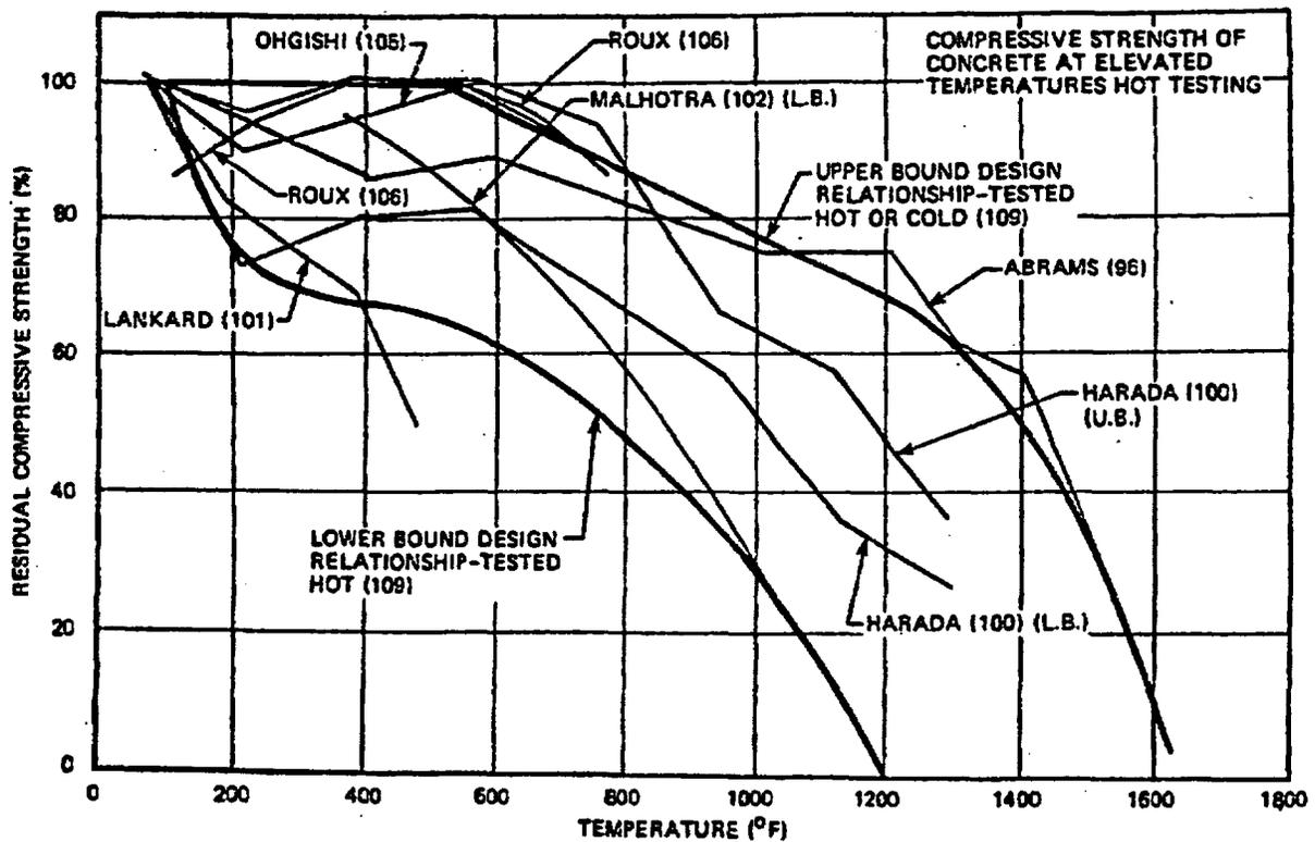
Figure 23 Effect of temperature exposure on compressive strength of concrete: tested hot. Source: G. N. Freskakis et al., "Strength Properties of Concrete at Elevated Temperature," *Civil Engineering Nuclear Power*, Vol. 1, ASCE National Convention, American Society of Civil Engineers, Boston, Massachusetts, April 1979.
