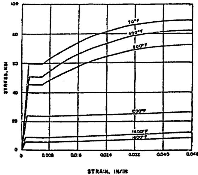
Figure 109 Stress-strain relationships for rebar used by Freskakis. Source: G. N. Freskakis, "Behavior of Reinforced Concrete at Elevated Temperature," Paper 3-4, *Second ASCE Conf. on Civ. Eng. and Nuclear Power*, Vol. 1, Paper 3-5, pp. 3-5-1 to 3-5-21, Knoxville, Tennessee, September 15-17, 1980.
