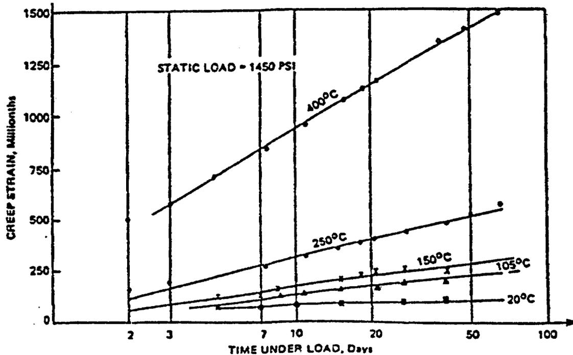
Figure 50 Creep of Portland cement/porphyry concrete at various temperatures. Source: A. C. Marechal, "Variations in the Modulus of Elasticity and Poisson's Ratio with Temperature," Paper SP 34-27 in Special Publication SP-34, Vol. I-III, American Concrete Institute, Farmington Hills, Michigan, 1972.
