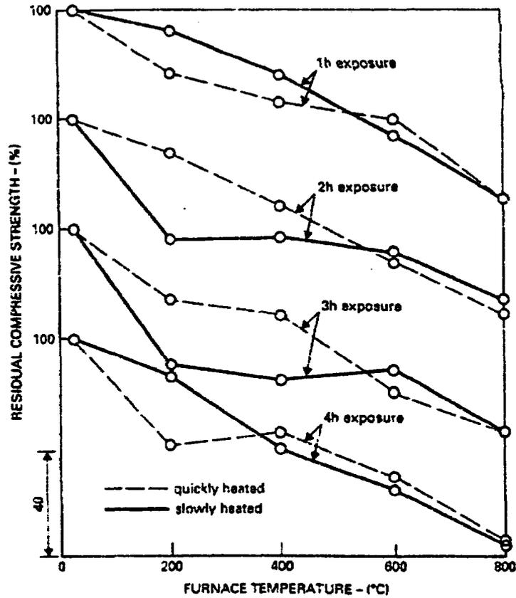
**Figure 33** Effect of rate of heating on residual strength of slowly cooled concrete. *Source:* G. T. C. Mohamedbhai, "Effect of Exposure Time and Rates of Heating and Cooling on Residual Strength of Heated Concrete," *Magazine of Concrete Research* 38(136), 151-158 (September 1986).
