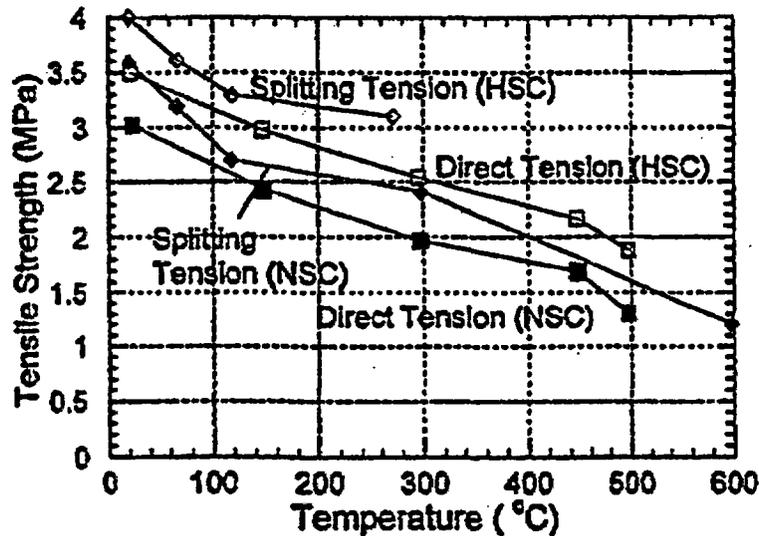
Figure 40 Residual tensile strengths of HSC and NSC. Source: A. N. Noumowe et al., "Thermal Stresses and Water Vapor Pressure of High Performance Concrete at High Temperature," *Proc. 4th International Symposium on Utilization of High-Strength/High-Performance Concrete, Paris, 1996*.
