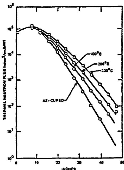
**Figure 74** Thermal neutron distribution in ordinary concrete as a function of temperature. *Source:* E. G. Peterson, "Shielding Properties of Ordinary Concretes as a Function of Temperature," HW-65572, Hanford Atomic Products Operation, Richland, Washington, August 2, 1960.
