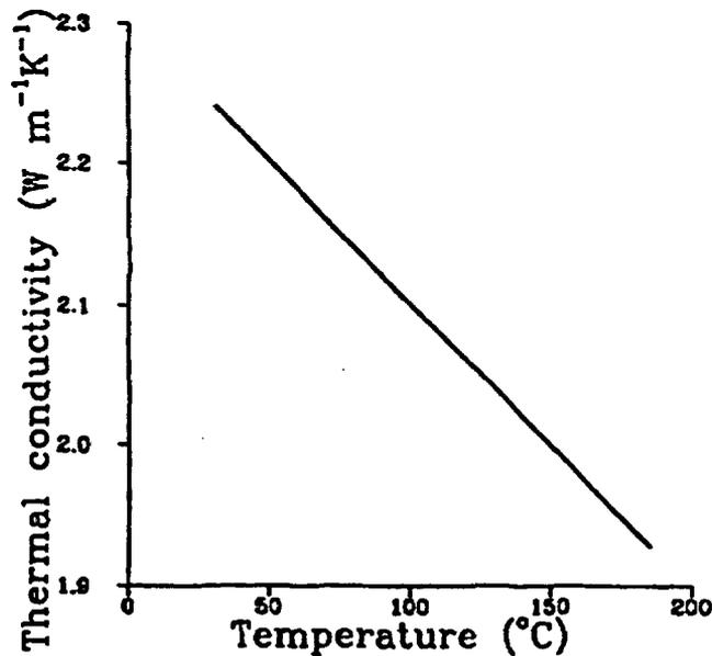
Figure 89 Temperature dependence of thermal conductivity of a nuclear power plant concrete. Source: F. Vodak et al., "Thermophysical Properties of Concrete for Nuclear Safety-Related Structures," *Cement and Concrete Research* 27(3), 415-426 (1997).
