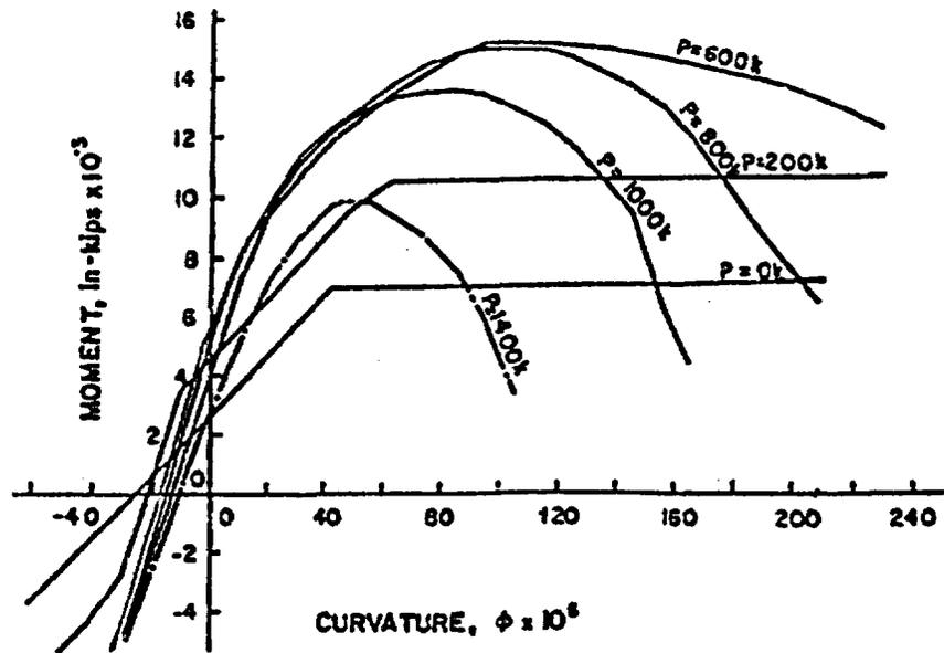
**Figure 112**  $M-\phi-P$  relationships:  $T_1 = 300^\circ\text{F}$  (based on lower bound relations). Source: G. N. Freskakis, "Behavior of Reinforced Concrete at Elevated Temperature," Paper 3-4, *Second ASCE Conf. on Civ. Eng. and Nuclear Power*, Vol. 1, Paper 3-5, pp. 3-5-1 to 3-5-21, Knoxville, Tennessee, September.
