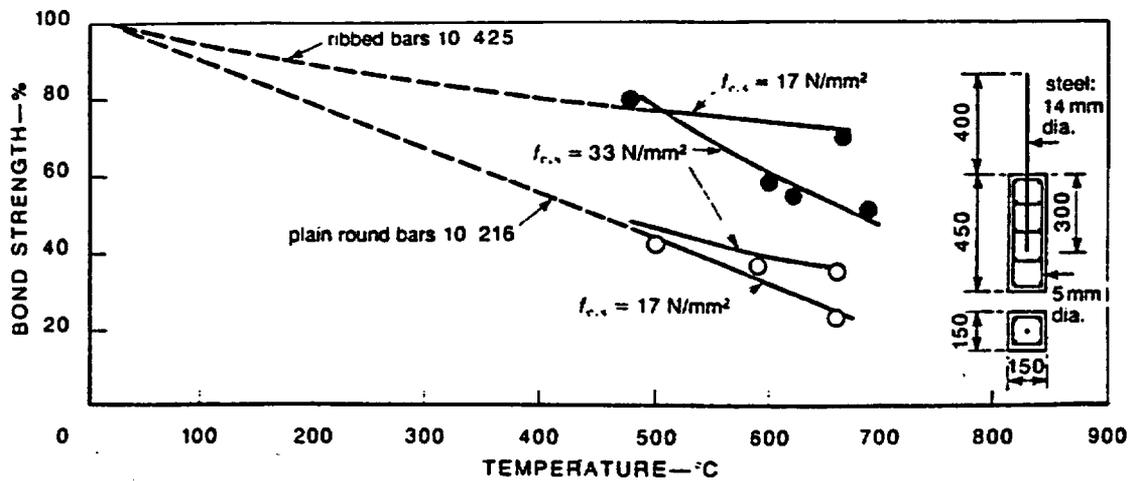
Figure 55 Bond strength of ribbed and plain round bars for different concrete compressive strengths. Source: H. V. Reichel, "How Fire Affects Steel-to-Concrete Bond," *Building Research and Practice* 6(3), 176-186 (May/June 1978).
