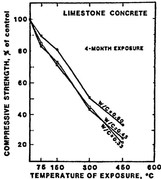
**Figure 66** Compressive strength of limestone concrete after 4-month exposure to various temperatures (up to 450°C). *Source:* G. G. Carrette and V. M. Malhotra, "Performance of Dolostone and Limestone Concretes at Sustained High Temperatures," *Proceedings of Symposium Temperature Effects on Concrete*, ASTM Special Technical Publication 858, pp. 38-67, American Society for Testing and Materials, West Conshohocken, Pennsylvania, 1985.
