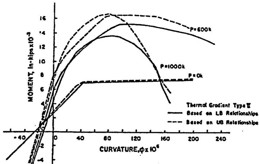
Figure 115  $N-\phi-P$  diagrams based on upper and lower bound strength relations. Source: G. N. Freskakis, "Behavior of Reinforced Concrete at Elevated Temperature," Paper 3-4, *Second ASCE Conf. on Civ. Eng. and Nuclear Power*, Vol. 1, Paper 3-5, pp. 3-5-1 to 3-5-21, Knoxville, Tennessee, September 15-17, 1980.
