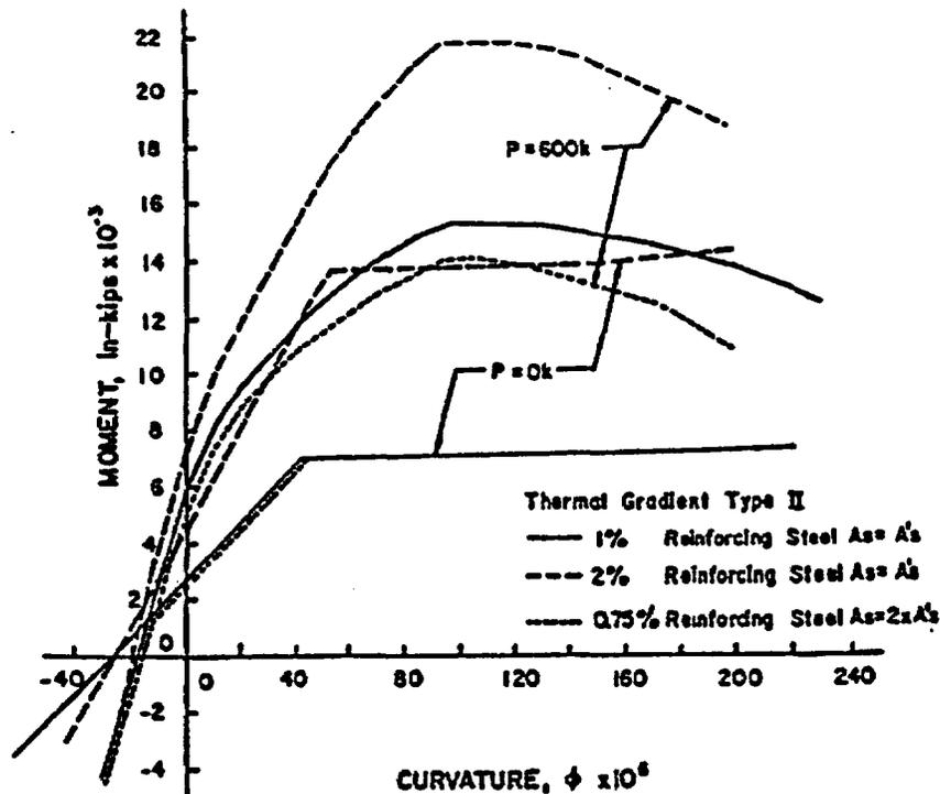
Figure 117 Effect of reinforcing steel on behavior (based on lower bound relations). Source: G. N. Freskakis, "Behavior of Reinforced Concrete at Elevated Temperature," Paper 3-4, *Second ASCE Conf. on Civ. Eng. and Nuclear Power*, Vol. 1, Paper 3-5, pp. 3-5-1 to 3-5-21, Knoxville, Tennessee, September 15-17, 1980.
