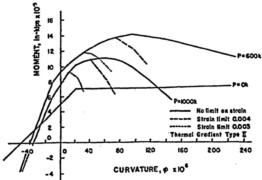
Figure 119 Effect of strain limits on behavior:  $T_1 = 500^\circ\text{F}$  (based on lower bound relation). Source: G. N. Freskakis, "Behavior of Reinforced Concrete at Elevated Temperature," Paper 3-4, *Second ASCE Conf. on Civ. Eng. and Nuclear Power*, Vol. 1, Paper 3-5, pp. 3-5-1 to 3-5-21, Knoxville, Tennessee, September 15-17, 1980.
