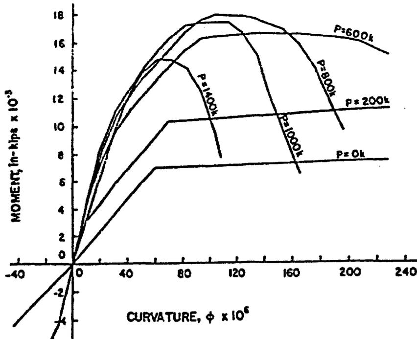
Figure 111 M- $\phi$ -P relationships: normal temperature. Source: G. N. Freskakis, "Behavior of Reinforced Concrete at Elevated Temperature," Paper 3-4, *Second ASCE Conf. on Civ. Eng. and Nuclear Power*, Vol. 1, Paper 3-5, pp. 3-5-1 to 3-5-21, Knoxville, Tennessee, September 15-17, 1980.
