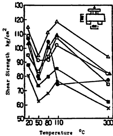
Figure 73 Shear strength of heated concrete. Source: H. Kasami, T. Okuno, and S. Yamane, "Properties of concrete Exposed to Sustained Elevated Temperature," Paper H1/5 in *Proc. 3rd International Conference on Structural Mechanics in Reactor Technology*, Elsevier Science Publishers, North-Holland, The Netherlands, 1975.
