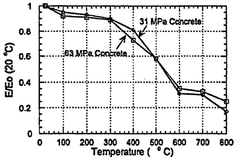
Figure 21 Normalized modulus of elasticity versus temperature relationships NSC and HSC. Source: C. Castillo and A. J. Durani, "Effect of Transient High Temperature on High-Strength Concrete," *J. American Concrete Institute*, 87(1) (1990).
