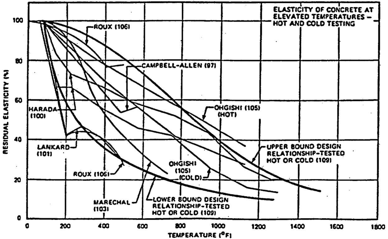
Figure 17 Effect of temperature on the modulus of elasticity of concrete: hot and cold test results. Source: G. N. Freskakis, "Behavior of Reinforced Concrete at Elevated Temperature," Paper 3-4, Source: ASCE Conf. on Civ. Eng. and Nuclear Power 1, Paper 3-5, pp. 3-5-1 to 3-5-21, Knoxville, Tennessee, Sept. 15-17, 1980.
