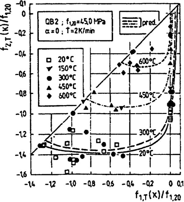
**Figure 76** Biaxial compressive strength at different temperatures. *Source:* K.-Ch. Thienel and F. S. Postasy, "Strength of Concrete Subjected to High Temperature and Biaxial Stress; Experiments and Modelling: Materials and Structures," 28, 575-581 (1995).
