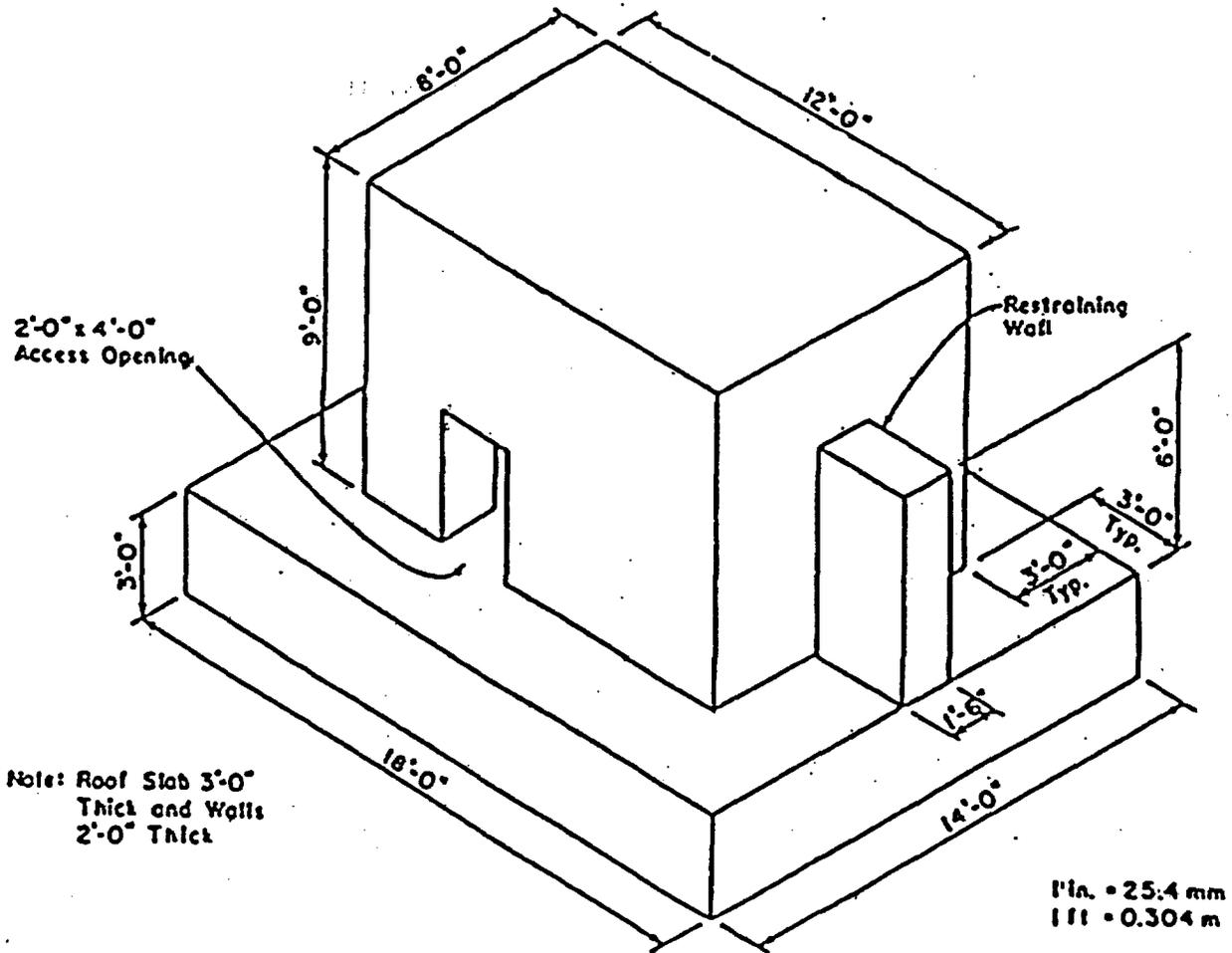
**Figure 146** Reinforced concrete box structure subject to thermal and mechanical loads to determine the general behavior of reinforced concrete at elevated temperature. *Source:* G. N. Freskakis, "High Temperature Concrete Testing," 8th CRIEP/EPRI Workshop, Agenda Item 7.2, Palo Alto, California, September 23-25, 1987.
