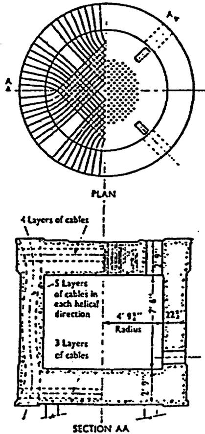
**Figure 157** 1:8-scale Oldbury PCRV Model. *Source:* I. W. Hornby, "The Behaviour of the Oldbury Model Vessel with Time Under Thermal and Pressure Loadings," Paper No. 11, *Model Techniques for Prestressed Concrete Pressure Vessels*, The British Nuclear Energy Society, London, 1968.
