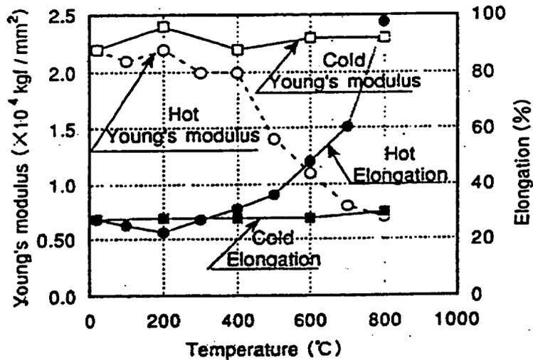
**Figure 9** Influence of temperature on Young's modulus and elongation of reinforcing bars. *Source:* M. Takeuchi et al., "Material Properties of Concrete and Steel Bars at Elevated Temperatures," *12th International Conference on Structural Mechanics in Reactor Technology*, Paper H04/4, pp. 133-138, Elsevier Science Publishers, North-Holland, The Netherlands, 1993.
