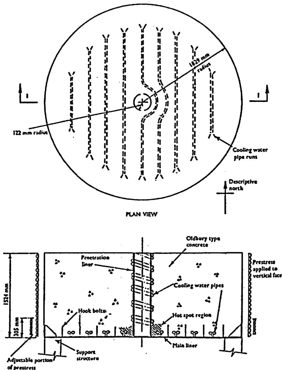
**Figure 158** Full-scale Oldbury hot-spot model. *Source:* J. Irving et al., "A Full Scale Model Test of Hot Spots in the Prestressed Vessels of Oldbury Nuclear Power Station," Paper 7699, *Proc. Instn. Civil Engineers* 57, June 1974.
