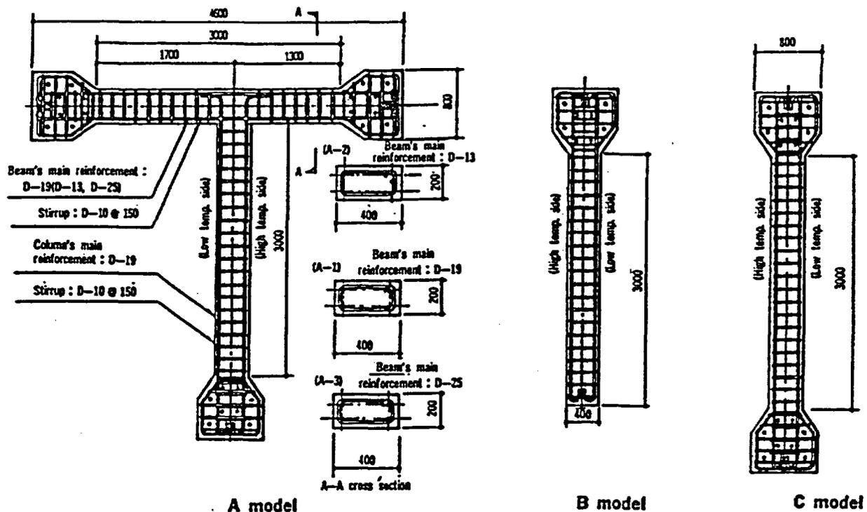
**Figure 124** Test articles used to demonstrate the decreased trend of bending moments and axial forces due to cracking and creep in RC structures. *Source:* G. T. Ikoma and N. Tanaka, "Restraining Force and Moment of Reinforced Concrete Beam Column Under a Sustained Long-Term Temperature Crossfall," Vol. H, *Trans. of 9th Ind. Conf. on St. Mech. in Reactor Technology*, pp. 201-208, Lausanne, Switzerland, August 17-21, 1987.
