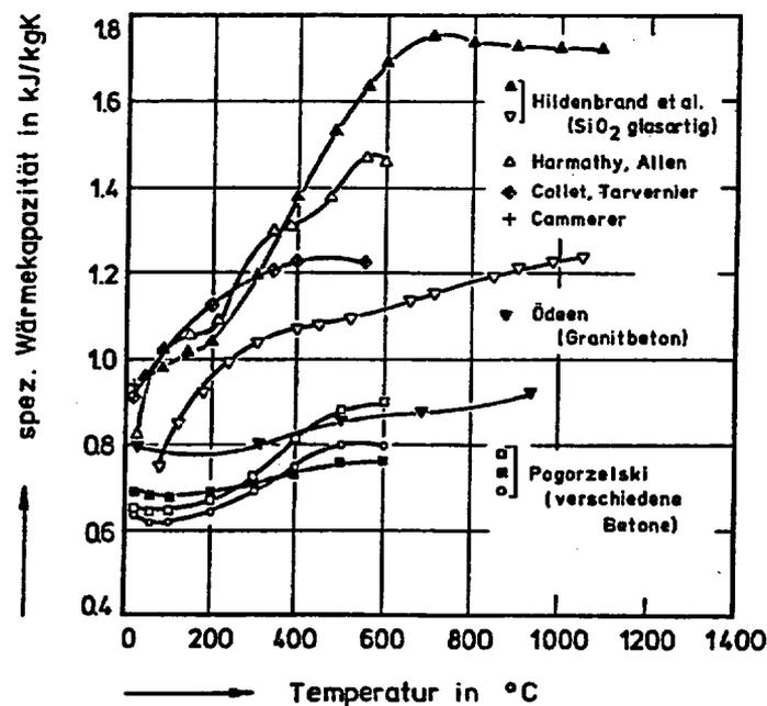
Figure 96 Specific heat capacity of siliceous aggregate concrete.
