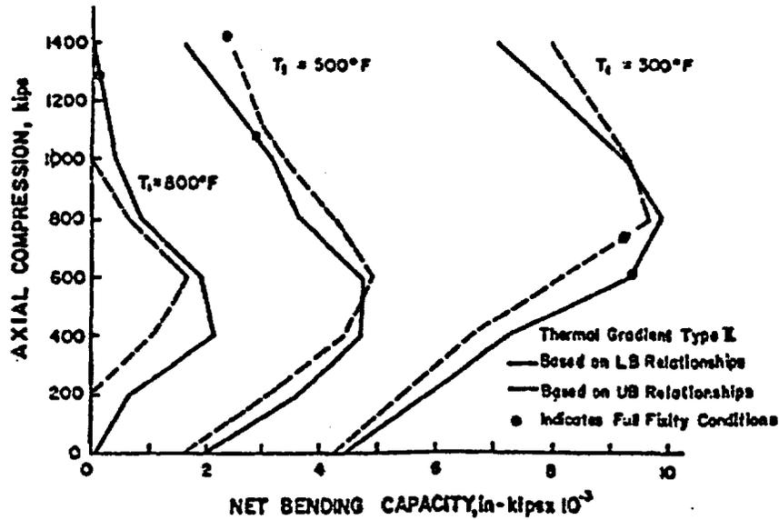
Figure 116 Net bending capacity based on upper and lower bound strength relations. Source: G. N. Freskakis, "Behavior of Reinforced Concrete at Elevated Temperature," Paper 3-4, *Second ASCE Conf. on Civ. Eng. and Nuclear Power*, Vol. 1, Paper 3-5, pp. 3-5-1 to 3-5-21, Knoxville, Tennessee, September 15-17, 1980.
