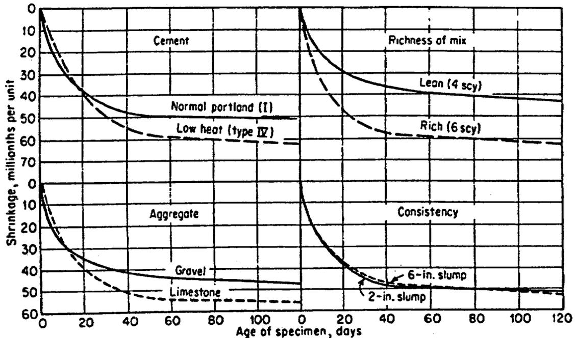
Figure 45 Effect of several factors on autogenous shrinkage of concrete. Source: G. E. Troxell, H. E. Davis, and J. W. Kelly, "Composition and Properties of Concrete," 2nd Ed., McGraw-Hill, New York, 1968.
