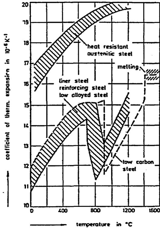
**Figure 7** Coefficient of expansion of different steels. *Source:* U. Schneider, C. Dierichs, and C. Ehm, "Effect of Temperature on Steel and Concrete for PCRV's," *Nuclear Engineering and Design* 67, 245-258 (1981).
