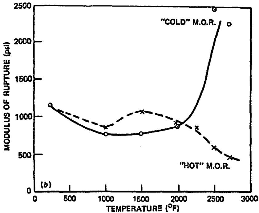
Figure 101 Typical hot and cold modulus of rupture results for a 40-50%  $\text{Al}_2\text{O}_3$  castable using (a) intermediate-purity cement and (b) high-purity cement. Source: W. T. Bakker et al., "Blast Furnace Gunning in the USA," *Proceedings International Feuerfest Colloquium, Aachen, Germany, October 27-29, 1971.*
