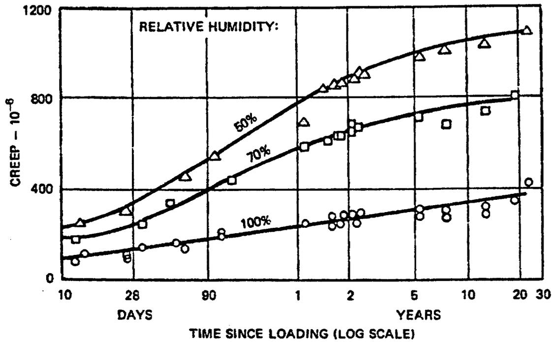
Figure 47 Creep of concrete stored at different relative humidities. Source: A. M. Neville, *Properties of Concrete*, Pitman, London, United Kingdom, 1970.
