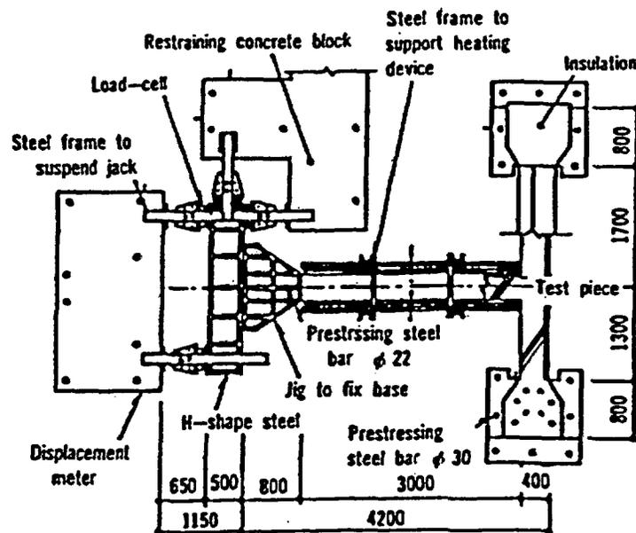
**Figure 125** Setup for applying loads and restraint to test articles in Fig. 124. Source: T. Ikoma and N. Tanaka, "Restraining Force and Moment of Reinforced Concrete Beam Column Under a Sustained Long-Term Temperature Crossfall," Vol. H, *Trans. of 9th Ind. Conf. on St. Mech. in Reactor Technology*, pp. 201-208, Lausanne, Switzerland, August 17-21, 1987.
