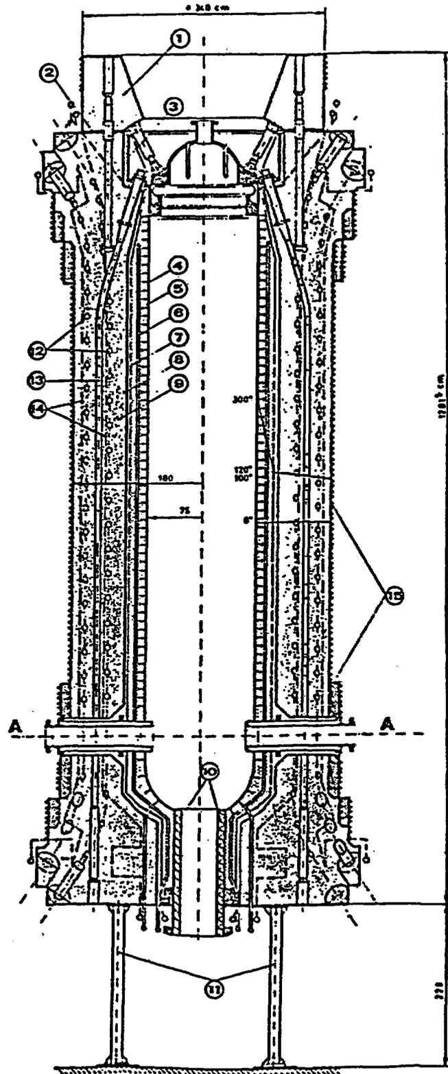
Figure 152 Austrian large PCRV model with hot liner. Source: J. Nemet et al., "Testing of a Prestressed Concrete Pressure Vessel with Hot Liner," Report SBB/He-3E, Reaktorbau Forschungs-und Baugesellschaft, Seibersdorf, Austria, November 1977.
