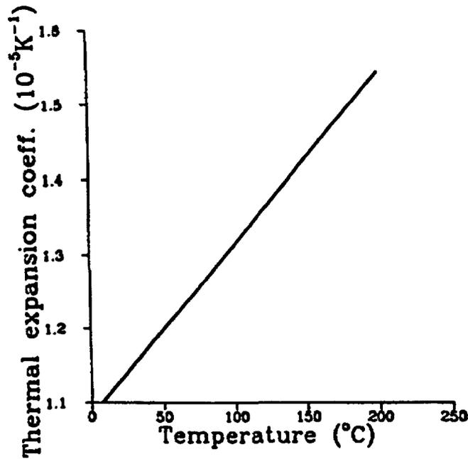
**Figure 84** Temperature dependence of linear thermal expansion coefficient of nuclear power plant concrete. *Source:* F. Vodak et al., "The Effect of Temperature on Strength—Porosity Relationship for Concrete," *Construction and Building Materials* 18, 529–534 (2004).
