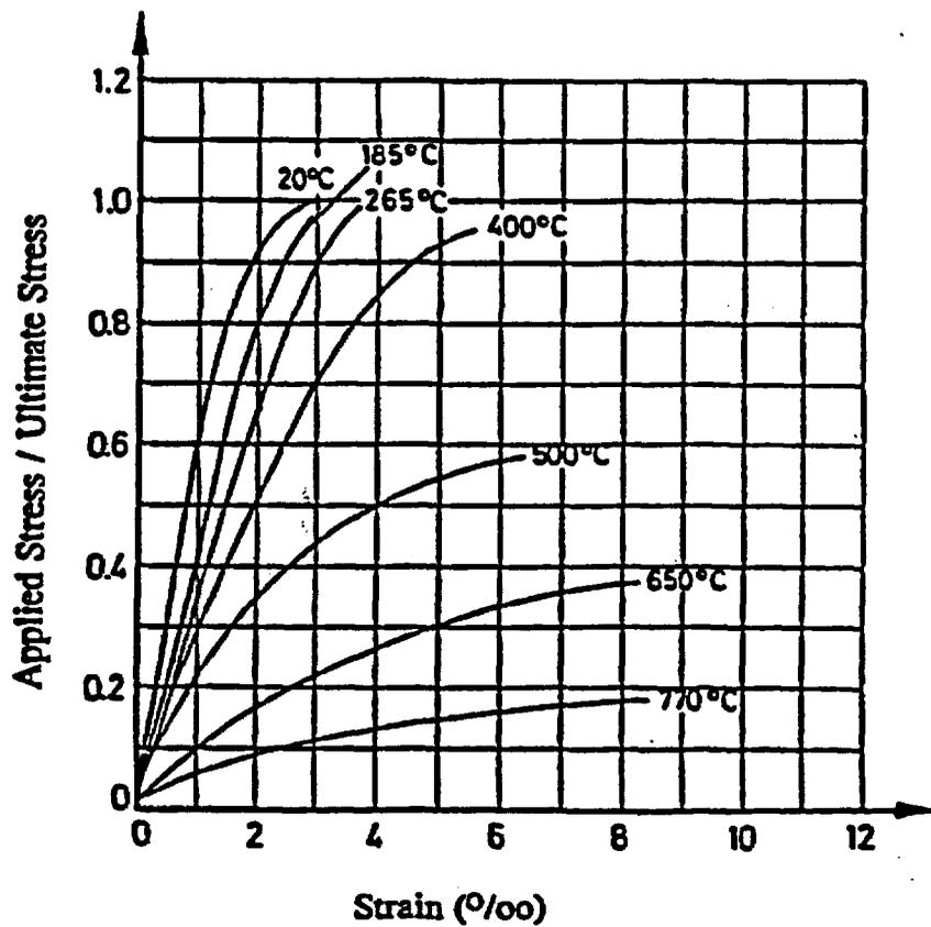
Figure 13 Influence of temperature on the stress-strain relation of unsealed quartz aggregate concrete. *Source:* Y. Anderberg and S. Thelanderson, "Stress and Deformation Characteristics of Concrete at High Temperatures, 2-Experimental Investigation and Material Behaviour Model," Bulletin 54, Lund Institute of Technology, Lund, Sweden, 1976.
