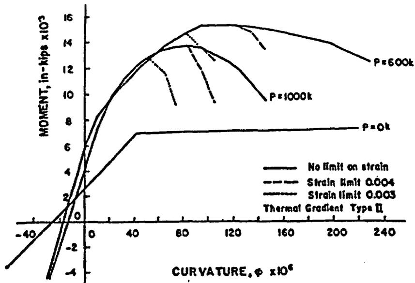
Figure 118 Effect of strain limits on behavior:  $T_1 = 300^\circ\text{F}$  (based on lower bound relations). Source: G. N. Freskakis, "Behavior of Reinforced Concrete at Elevated Temperature," Paper 3-4, *Second ASCE Conf. on Civ. Eng. and Nuclear Power*, Vol. 1, Paper 3-5, pp. 3-5-1 to 3-5-21, Knoxville, Tennessee, September 15-17, 1980.
