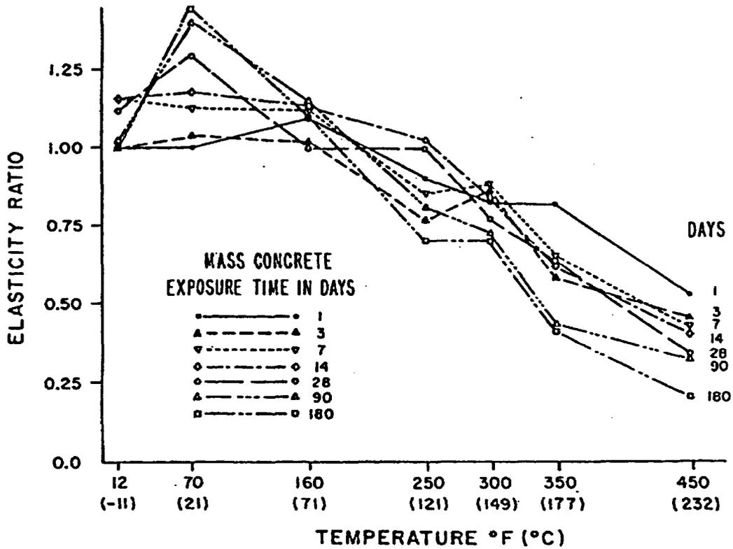
**Figure 64** Relationship of elasticity ratio and temperature of mass concrete (sealed). *Source:* K. W. Nasser and M. Chakraborty, "Temperature Effects on Strength and Elasticity of Concrete Containing Admixtures," *Proceedings of Symposium Temperature Effects on Concrete*, ASTM Special Technical Publication 858, American Society for Testing and Materials, West Conshohocken, Pennsylvania, 1985.
