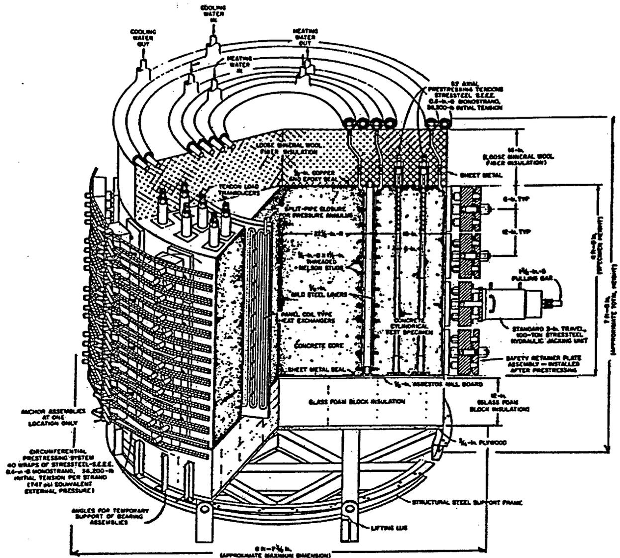
Figure 163 Isometric of ORNL thermal cylinder test structure. Source: J. J. P. Callahan et al., *Prestressed Concrete Reactor Vessel Thermal Cylinder Model Study*, ORNL/TM-5613, Oak Ridge National Laboratory, June 1977.
