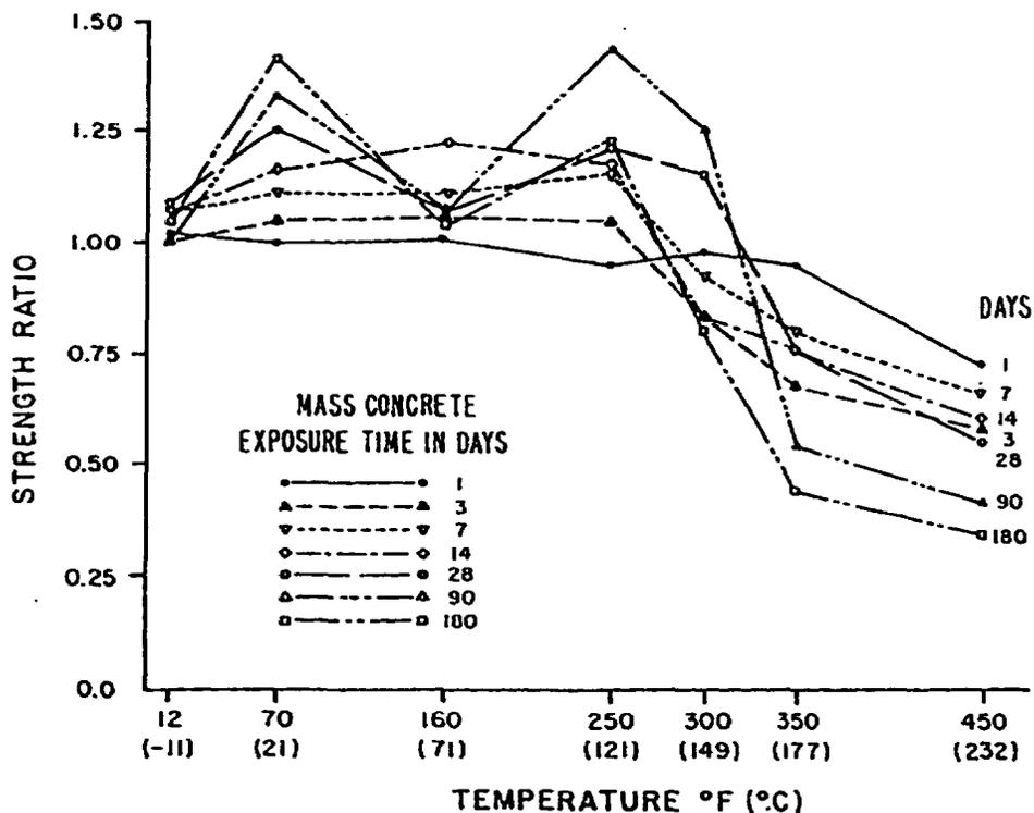
**Figure 63** Relationship of strength ratio and temperature of mass concrete (sealed).
