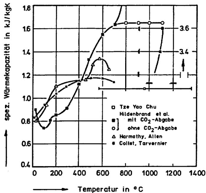
Figure 95 Specific heat capacity of limestone aggregate concrete.
