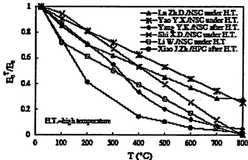
Figure 18 Temperature dependence of the concrete modulus of elasticity (normalized). Source: J. Xiao and G. König, "Study of Concrete at High Temperature in China—An Overview," *Fire Safety Journal* 39, 89-103 (2004).
