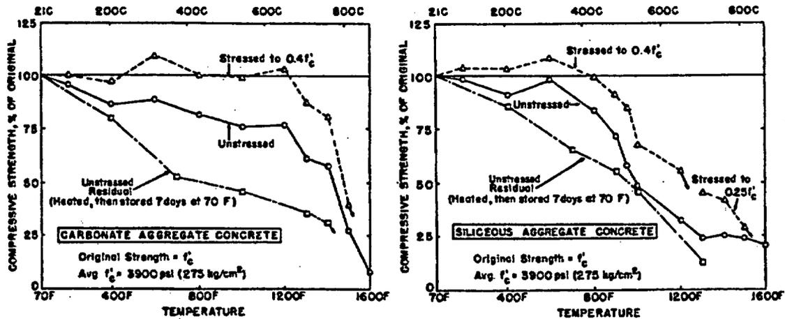
Figure 36 Effect of exposure time on residual strength of carbonate and siliceous aggregate concretes. Source: M. S. Abrams, "Compressive Strength of Concrete at Temperatures to 1600°F," SP-25 *Temperature and Concrete*, American Concrete Institute, pp. 33-58, 1971.
