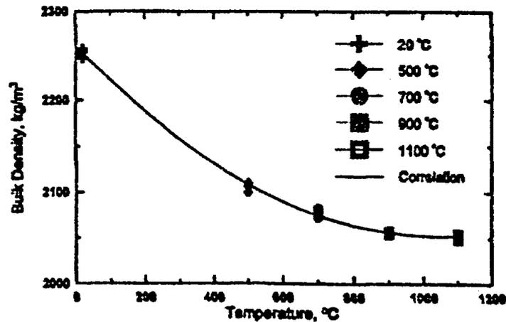
Figure 79 Density of a nuclear power plant concrete. Source: K.-Y. Shin et al., "Thermo-Physical Properties and Transient Heat Transfer of Concrete at Elevated Temperatures," *Nuclear Engineering and Design* 212, 233–241 (2002).
