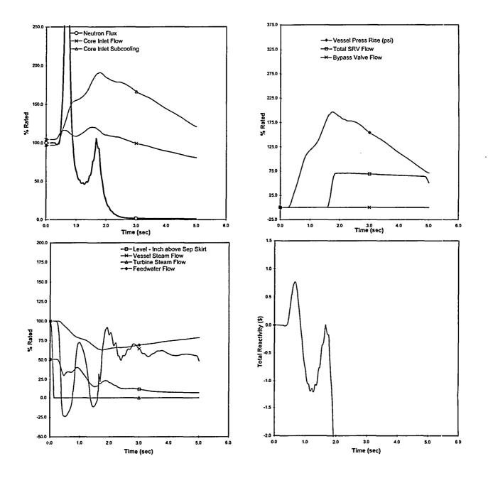
Figure 4 Plant Response to Load Rejection w/o Bypass (EOC ICF (HBB))
