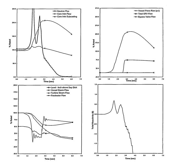
Figure 8 - Plant Response to MSIV Closure (Flux Scram) - ICF (HBB)
