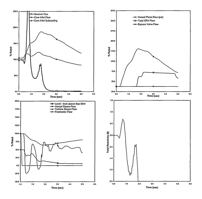
Figure 2 Plant Response to Load Rejection w/o Bypass (MOC ICF (HBB))
