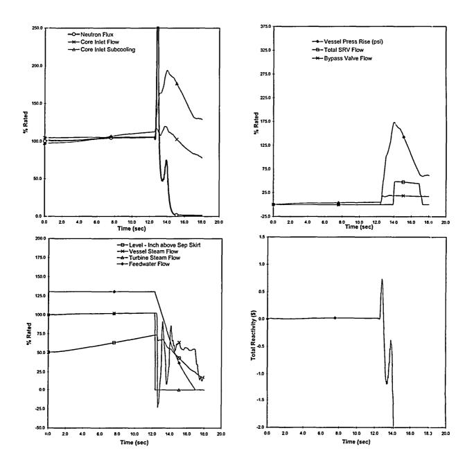
Figure 5 Plant Response to FW Controller Failure (EOC ICF (HBB))
