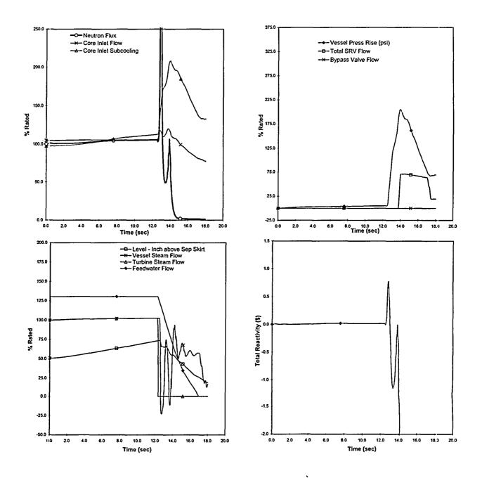
Figure 6 Plant Response to FW Controller Failure (EOC NFWT ICF (HBB) with TBVOOS)
