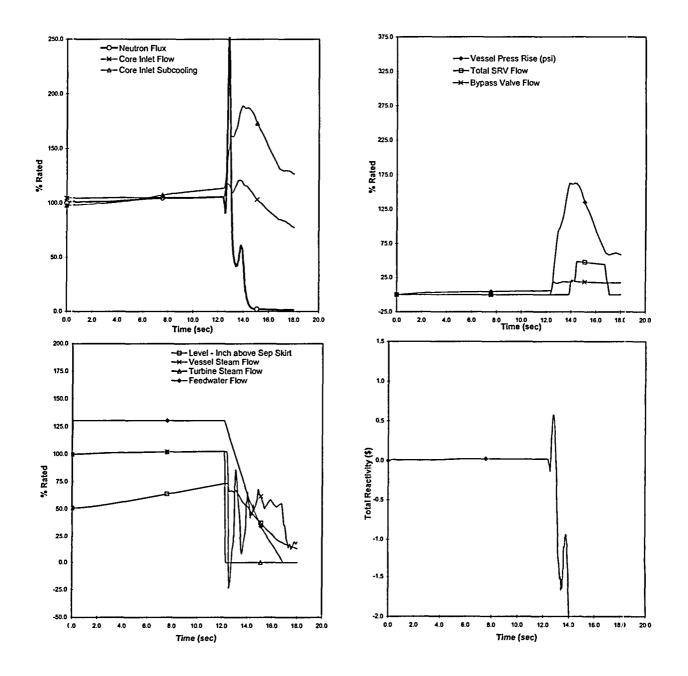
Figure 3 Plant Response to FW Controller Failure (MOC ICF (HBB))
