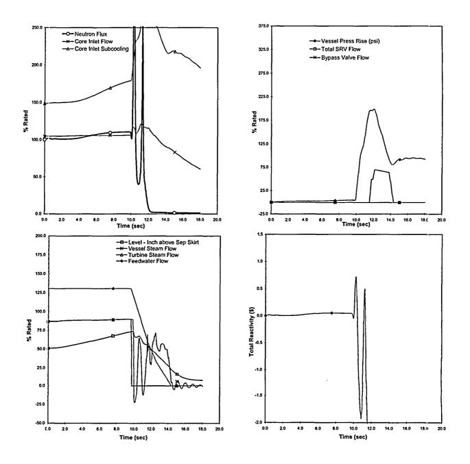
Figure 7 Plant Response to FW Controller Failure (EOC RFWT ICF (UB) with TBVOOS)
