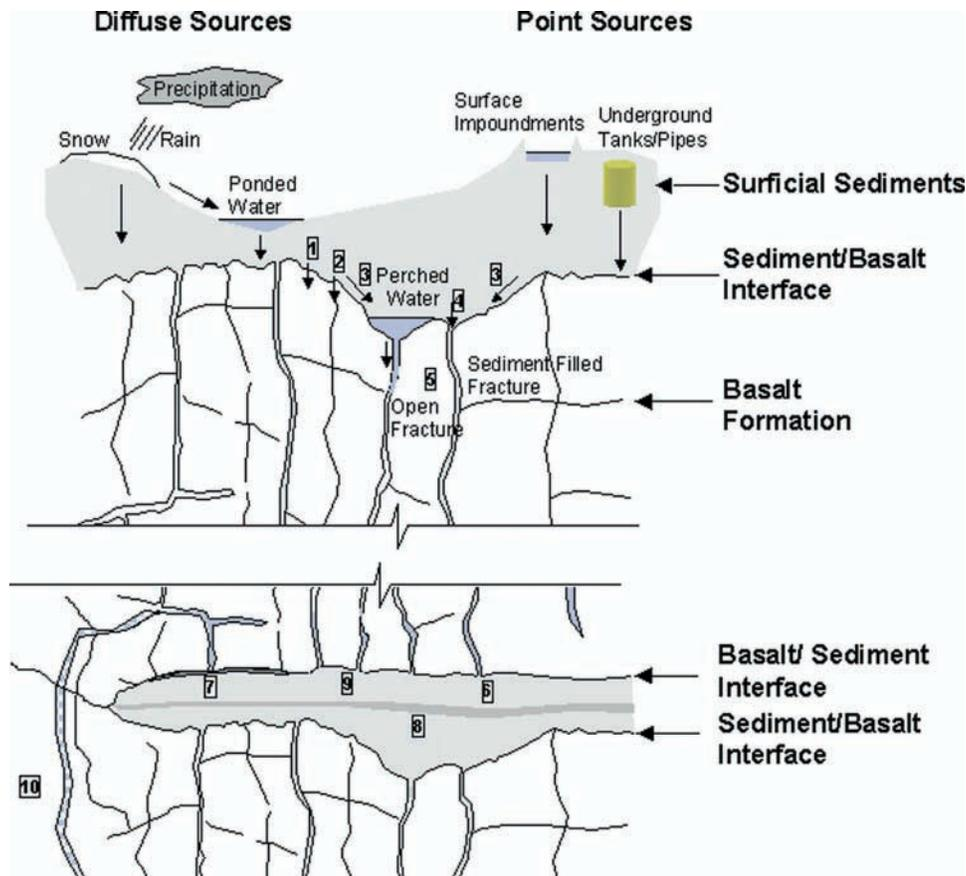
Fig. 5. Mechanism controlling water recharge at the upper sedimentary–basalt interface and at subsurface sedimentary interbeds.
