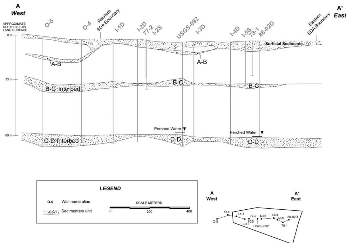
Fig. 2. Stratigraphic illustration of the sedimentary interbed structure beneath the Subsurface Disposal Area.
