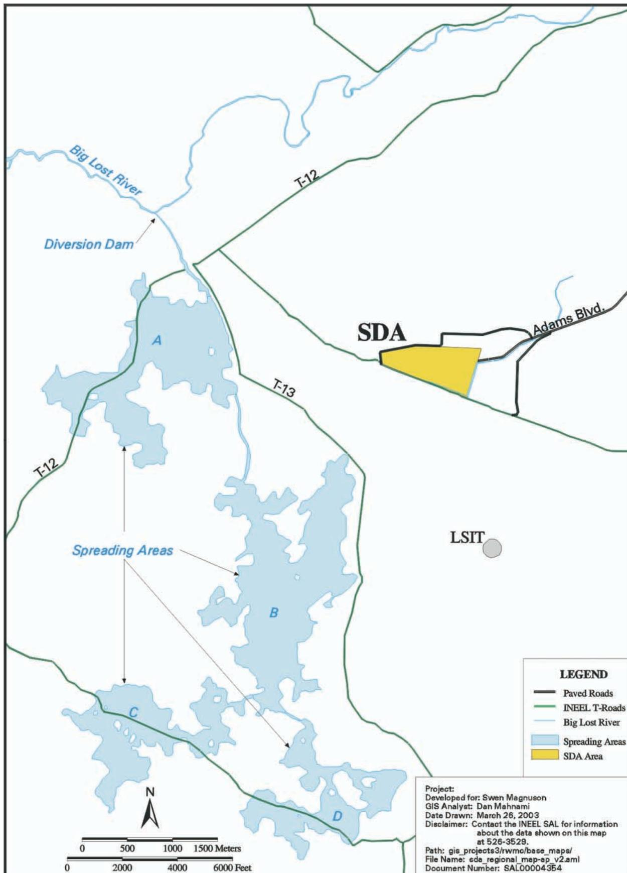
Fig. 3. Location of the Big Lost River, the spreading areas and the large-scale infiltration test in relationship to the Subsurface Disposal Area.
