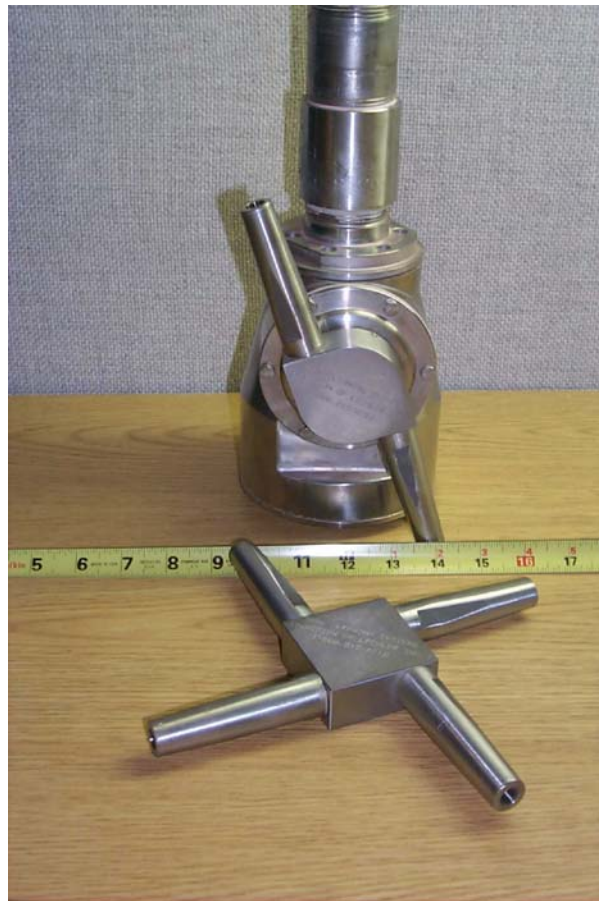
Figure 2. Wash ball with 2 head nozzle attached, 4 head nozzle shown in foreground.
