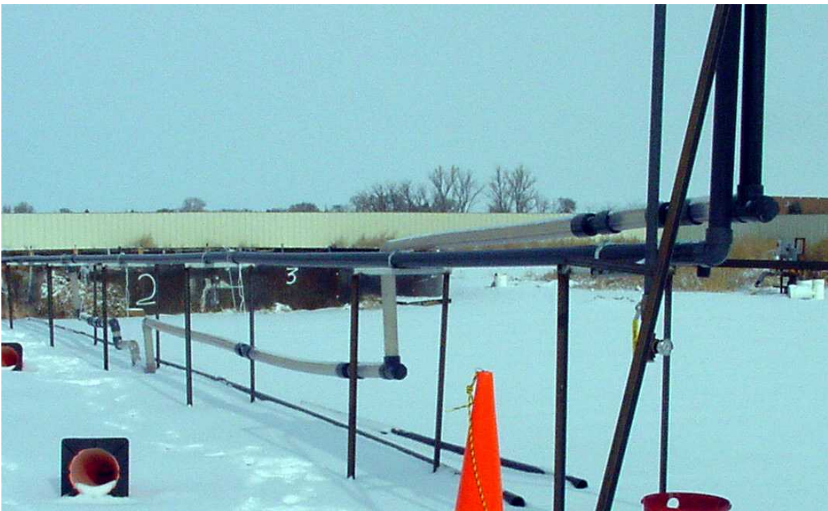
Figure 15. Clear pipe for Mockup solids transfer testing.
