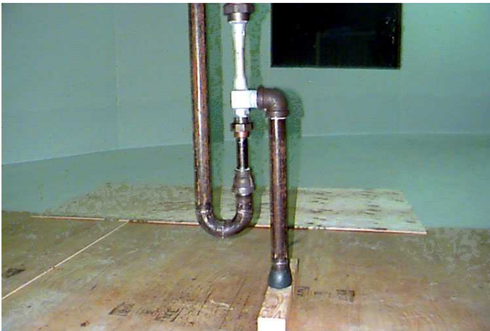
Figure 11. Steam jet mounted in Mockup structure prior to washing.
