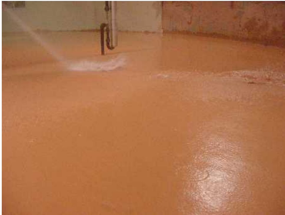
Figure 7. Mockup tank washing spray from wash ball.
