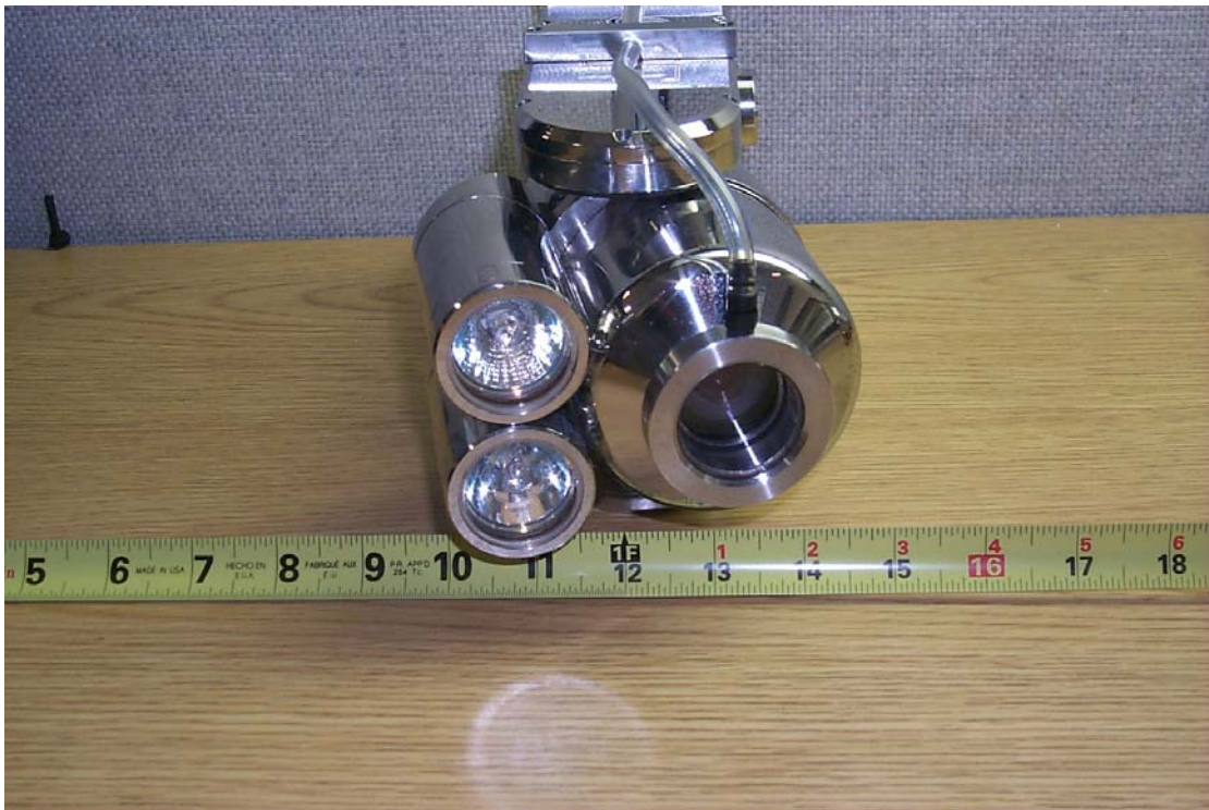
Figure 6. Video camera, showing air lance ring and the two factory mounted lights.
