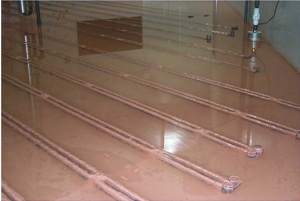
Figure 10. Mockup tank floor before directional spray wash.
