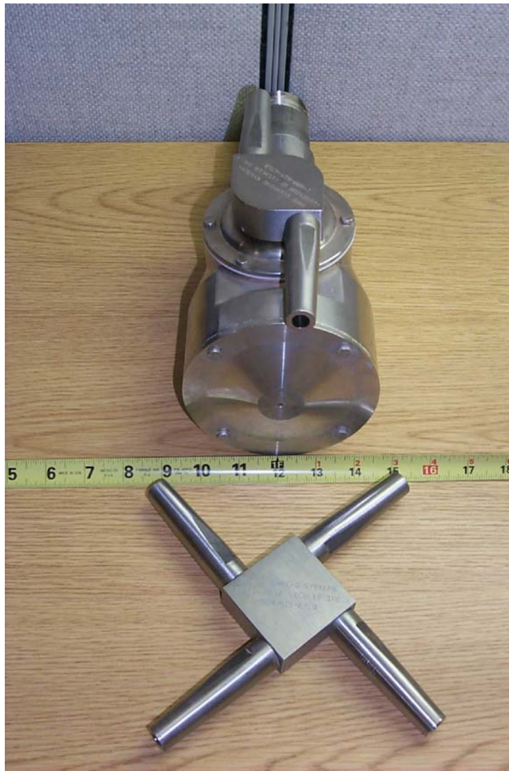
Figure 8. Wash ball, four-head nozzle and two head nozzle cross section comparison.
