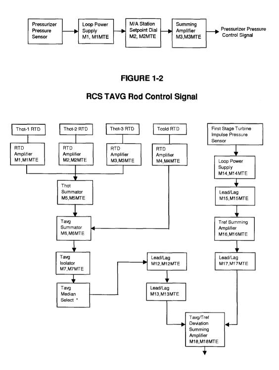
\* The Tavg Median Select Module consists of four individual devices which are shown in Table 1-2 as M8,M8MTE to M11,M11MTE.
