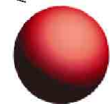
Dia. 0,5mm Uranium Dioxide Fuel Kernel
