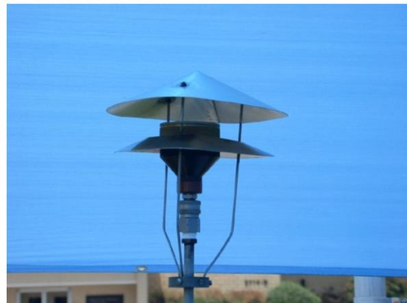
Device for monitoring airborne radiation
