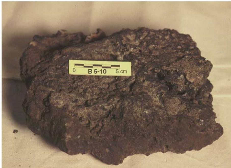
Figure 1-4. Hand sample of Site B slag. This sample is more crystalline than the one shown in Figure 1-3 indicating that it was from the interior of a melt block. (Photograph courtesy of CNWRA).
