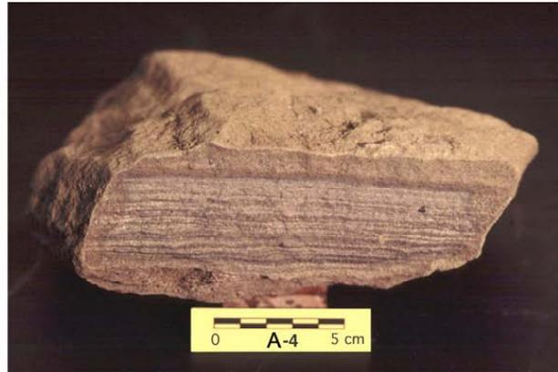
Figure 1-2. Site A samples. Note the sedimentary features of these samples. This material was produced by crushing, leaching, and deposition of the material in a settling pond. The dark layers are enriched in thorium. The outer 1.2 cm top surface of the slag is weathered to a red-brown phase (Ba oxyhydroxides). (Photograph courtesy of CNWRA).
