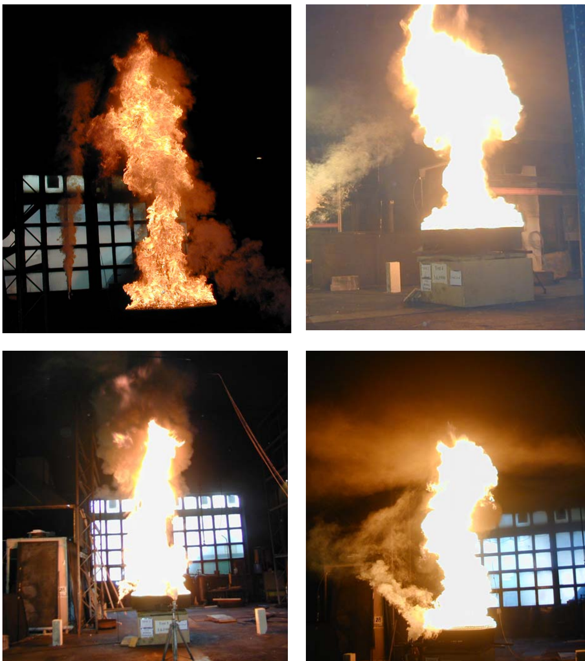
Figure A-12: Photographs of heptane pan fires, ICFMP BE #2, Case 2. Courtesy, Simo Hostikka, VTT Building and Transport, Espoo, Finland.
