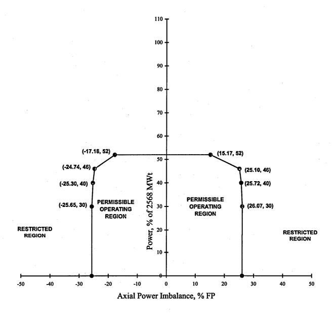
\* Assumes that no individual short emitter detector affecting the minimum in-core imbalance calculation exceeds 60% sensitivity depletion, and that no individual long emitter detector exceeds 73% sensitivity depletion, or both. The imbalance setpoints for the minimum in-core system must be reduced by 2.80% FP at the earliest time-in-life that this assumption is no longer valid.
