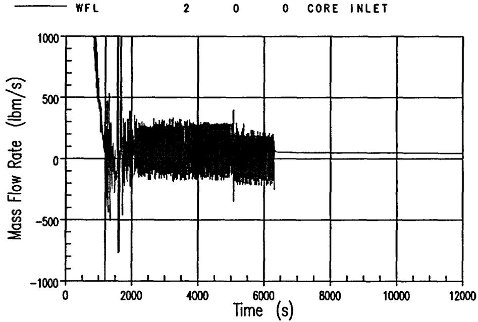
Figure E.13-18 BVPS-2 1.5-Inch Break, Core Inlet Flow
