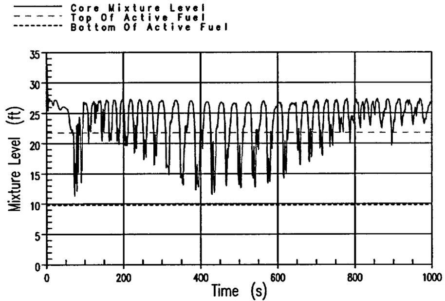
Figure E.11-8 BVPS-1 1.0-ft<sup>2</sup> Break, Core/Upper Plenum Mixture Level
