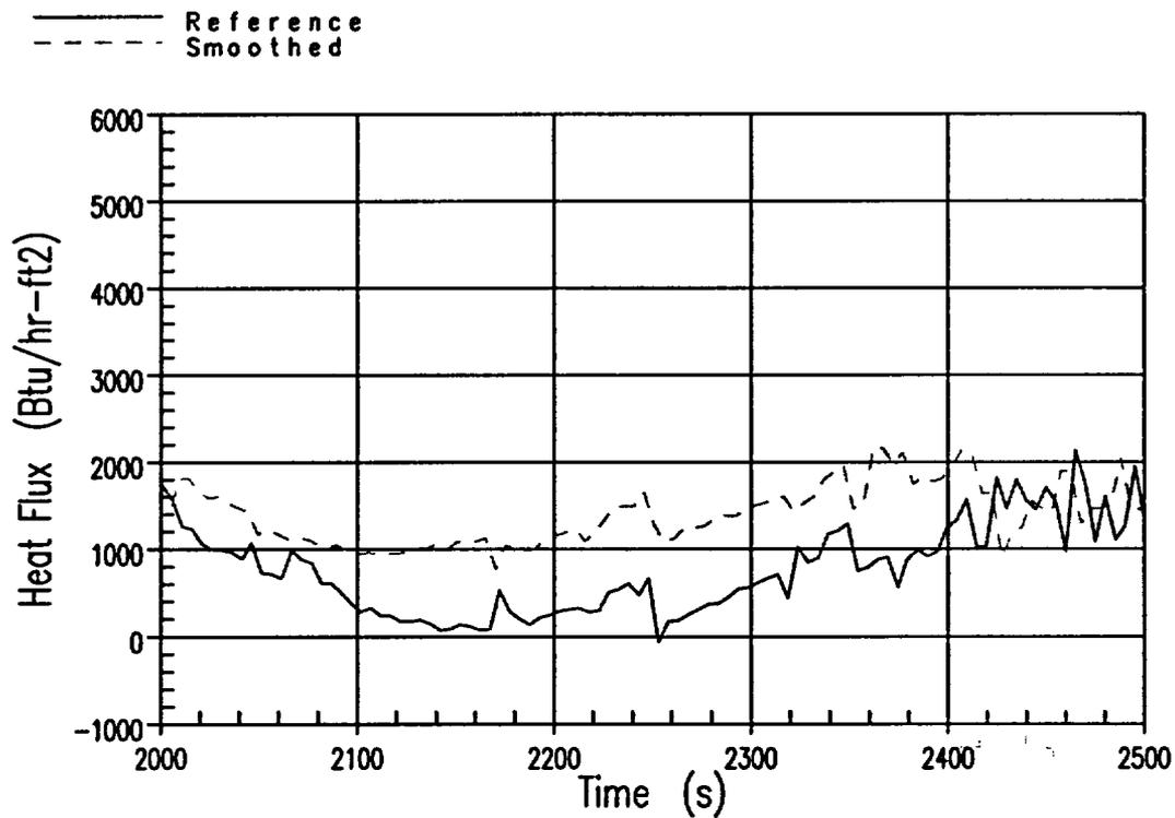
Figure E.6-4 BVPS-2 2-Inch Clad Surface Heat Flux (2200-2500 sec.)
