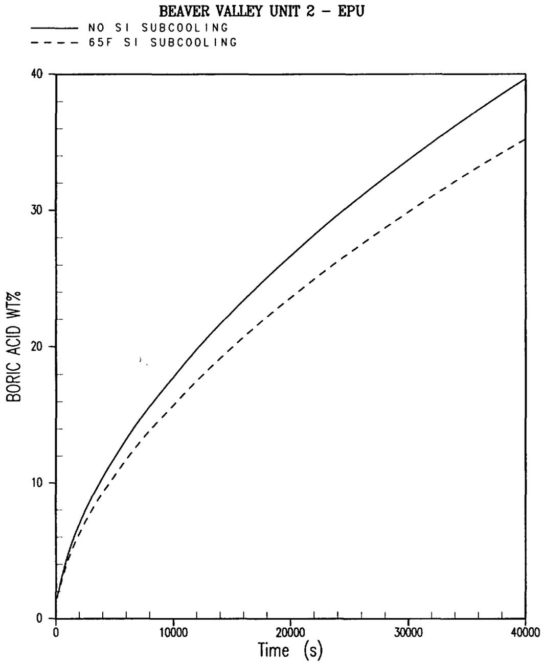
**Figure F-3 - Effect of 65°F Subcooling on Boric Acid Concentration (BVPS-2)**
