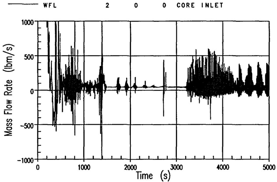
Figure E..13-22 BVPS-2 3-Inch Break, Core Inlet Flow
