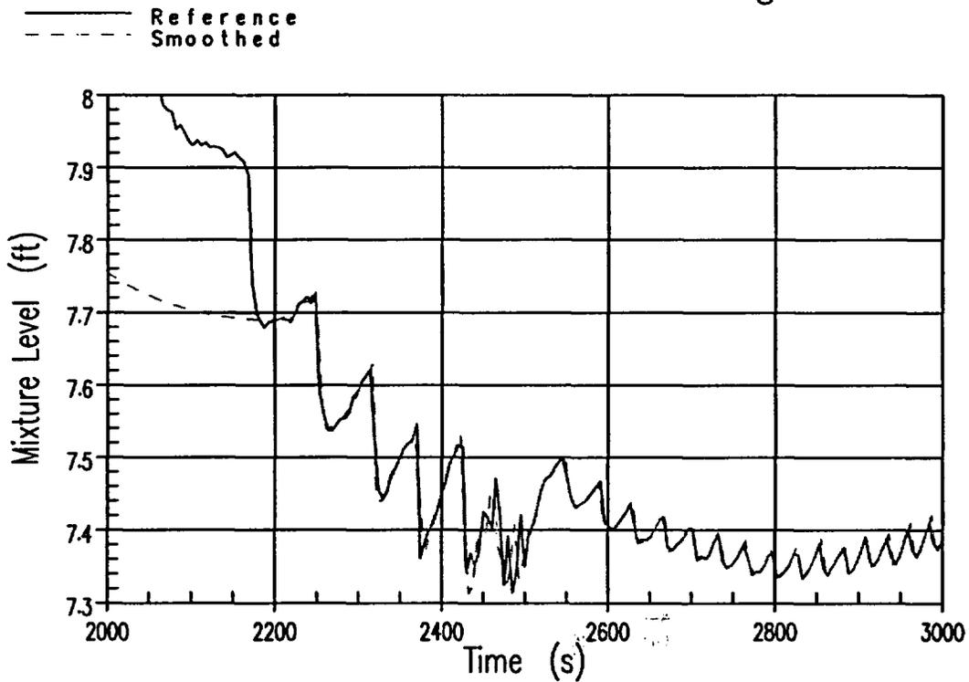
Figure E.6-2 BVPS-2 2-Inch Core Mixture Level Response (2200-3000 sec.)
