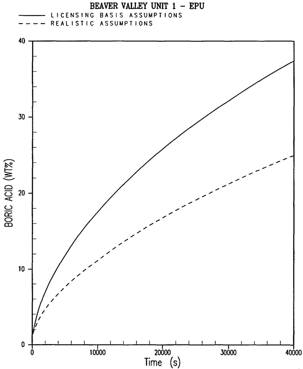
**Figure F-4 - Realistic Calculation of Vessel Boric Acid Concentration (BVPS-1)**
