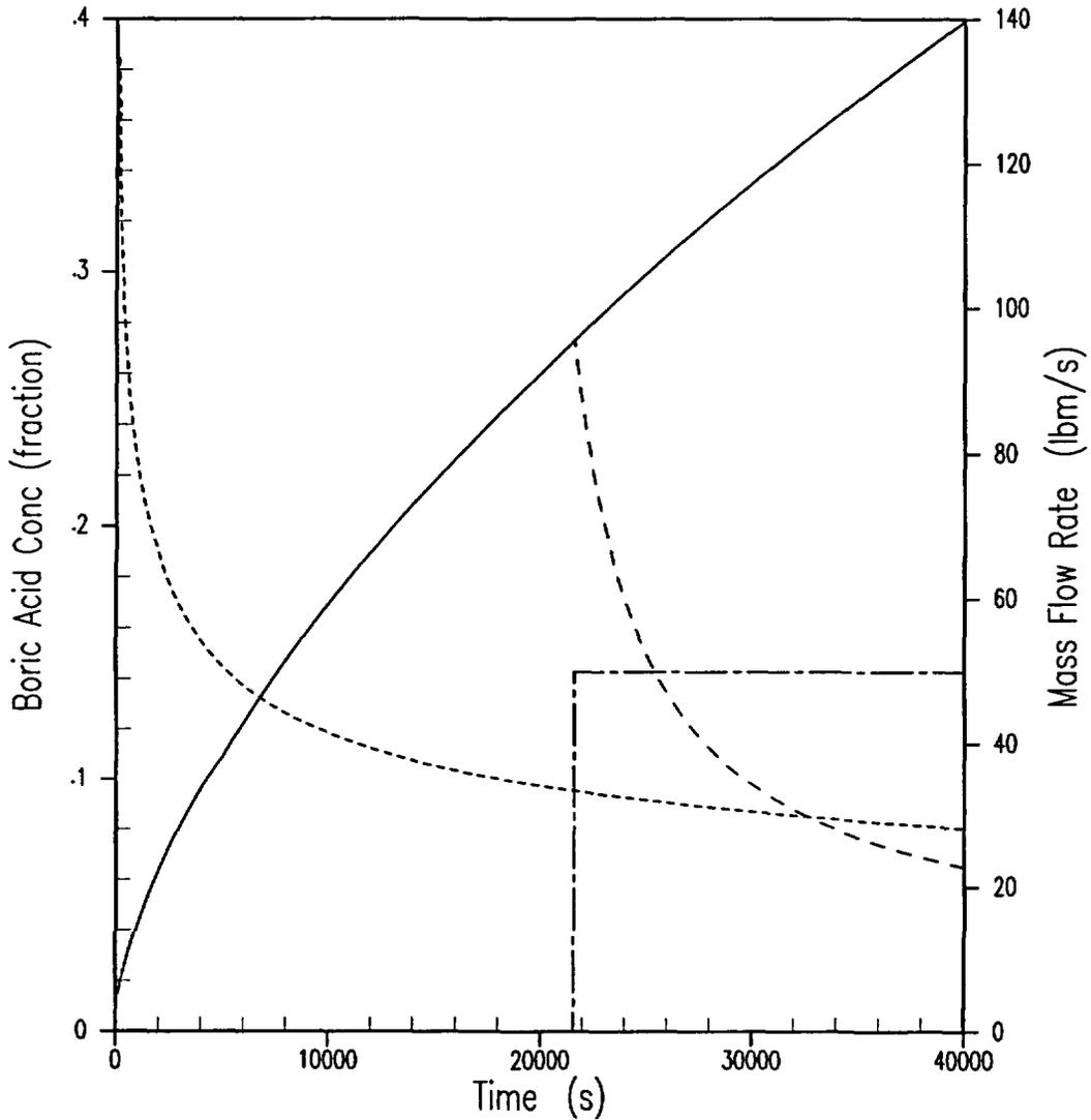
Figure F-7 - Vessel Boric Acid Concentration for 120 psia RCS Pressure (BVPS-2)
