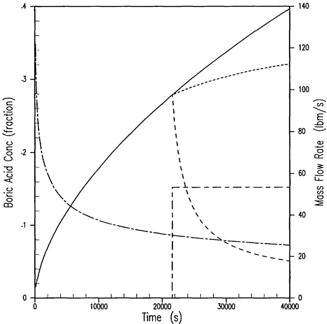
Figure F-9 - Boil-off, SI, and Core Dilution Rate at Hot Leg Switchover Time (BVPS-2)
