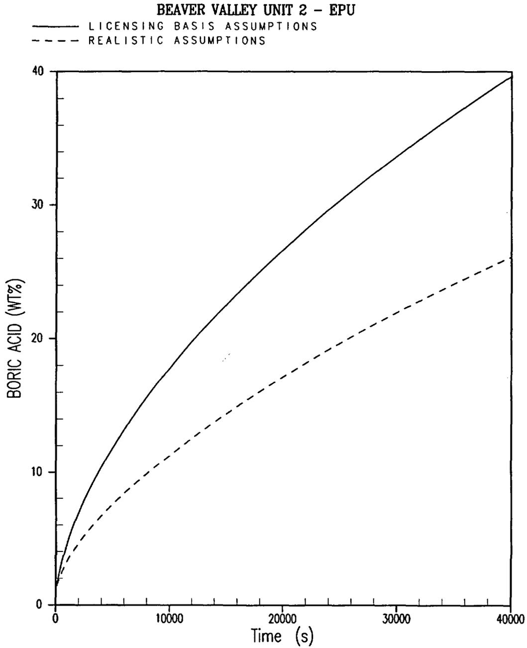
**Figure F-5 - Realistic Calculation of Vessel Boric Acid Concentration (BVPS-2)**
