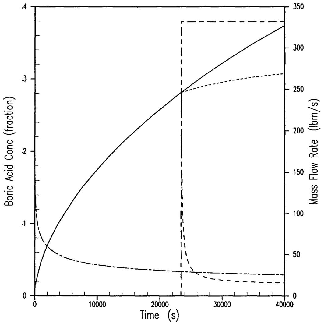
Figure F-8 - Boil-off, SI, and Core Dilution Rate at Hot Leg Switchover Time (BVPS-1)
