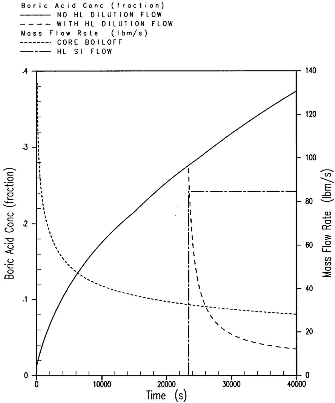
Figure F-6 - Vessel Boric Acid Concentration for 120 psia RCS Pressure (BVPS-1)
