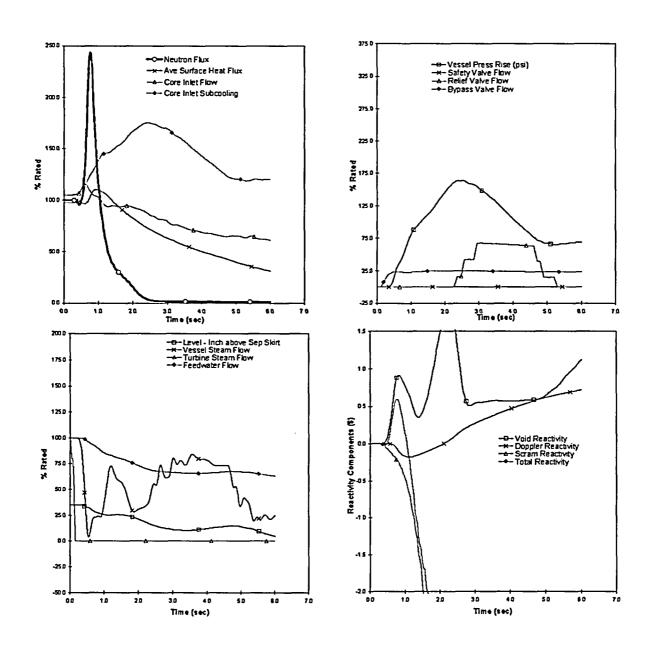
Figure 3-7: Load Rejection With Bypass
