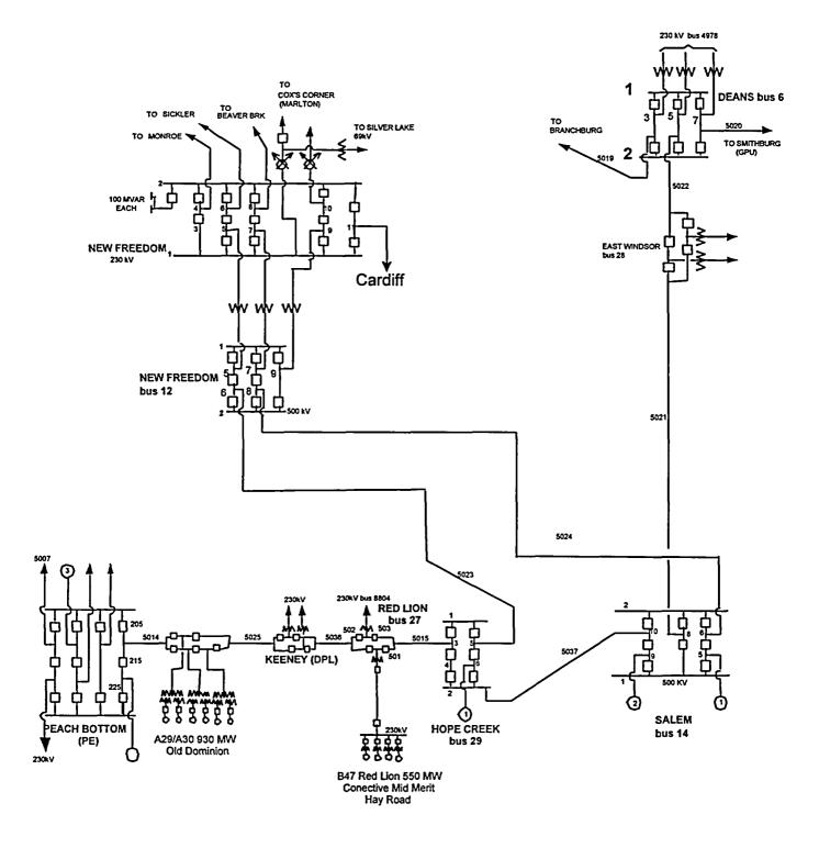
Figure 1 Artificial Island Offsite Electrical System One Line Diagram
