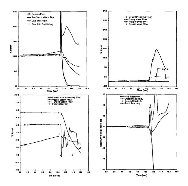
Figure 3-1: Feedwater Controller Failure
