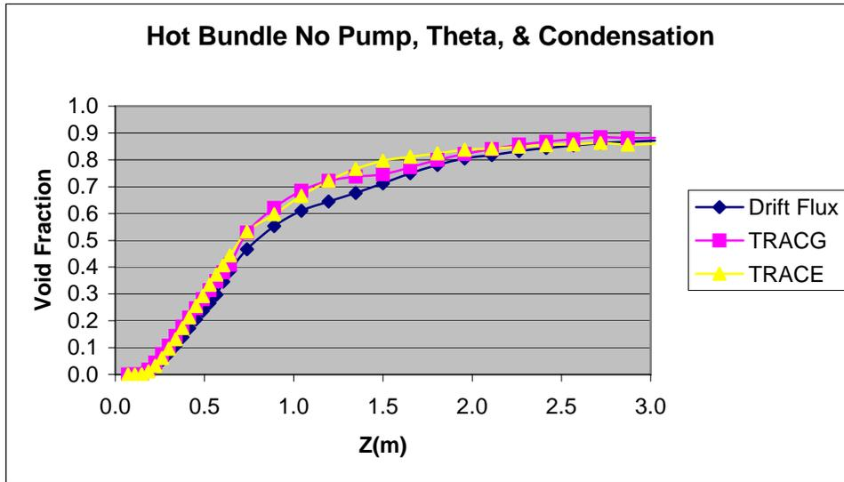
This also agreed quite well, which was not expected. The staff expected that in the subcooled region the TRACG data would agree with the drift flux model in the prior to the modifications since that model is using the same models in Ref. 1.
