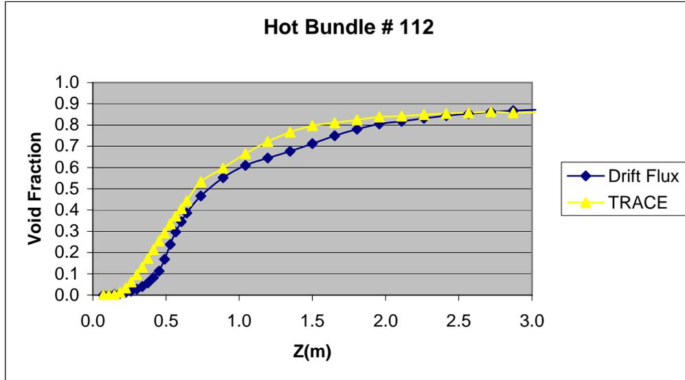
TRACG uses the Rouhani-Bowring model<sup>2</sup> for the energy distribution in subcooled boiling while TRACE uses the Lahey's mechanistic model<sup>3</sup>. The models are essentially the same, except the TRACE model does not include the pumping factor.
