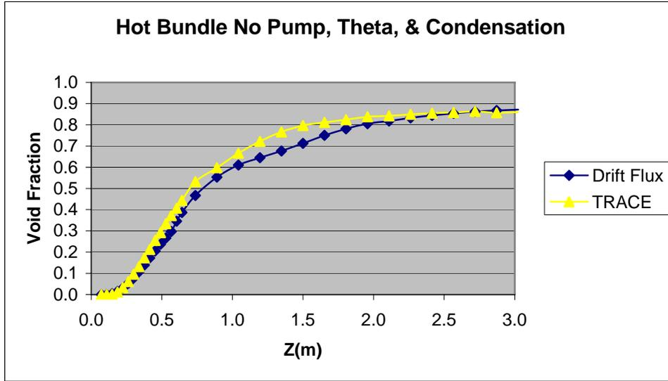
These void fraction profiles were then compared to the TRACG data in the MS Excel file MFN 05-014 Channel Data.
