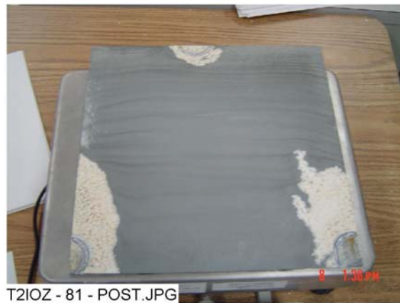
Figure 4-17. IOZ-81 submerged, post-test.
