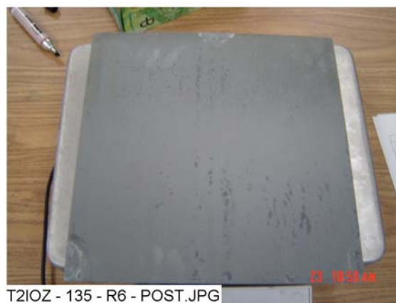
Figure 4-41. IOZ-135 unsubmerged, post-test.
