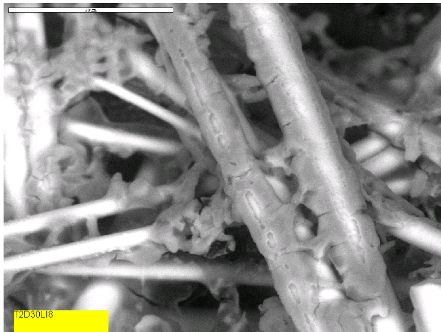
Figure 4-52. Higher-magnification ESEM image of a Test #2 Day 30 low-flow interior fiberglass sample.
