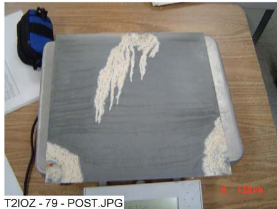
Figure 4-15. IOZ-79 submerged, post-test.
