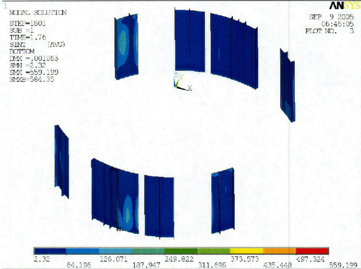
Figure EMEB-B-39-15 – Drain Channel Peak Stress Intensity
