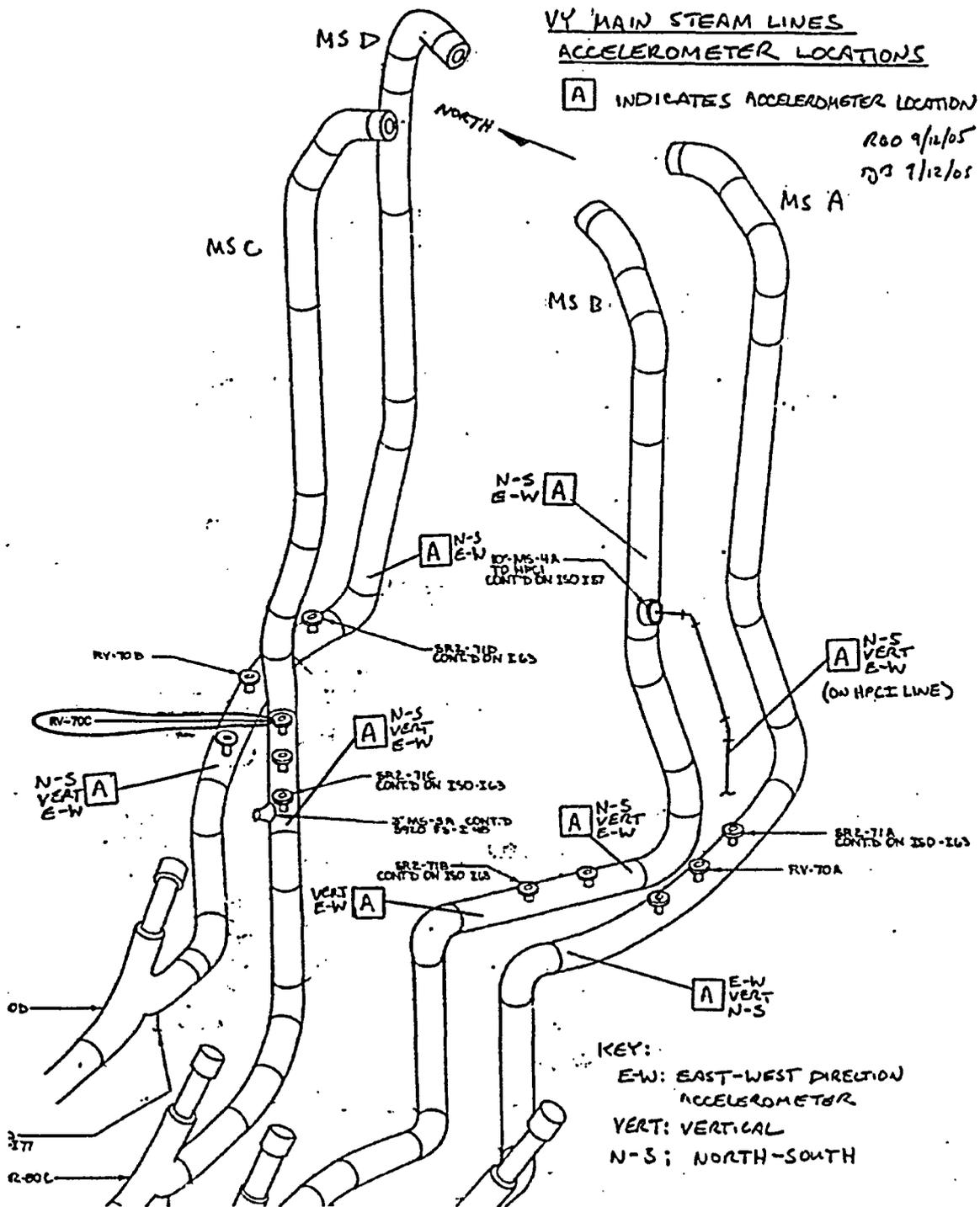
Figure EMEB-B-77-1 – Sheet 4: VYNPS Main Steam Piping Cavities and ACM Measurement Locations
