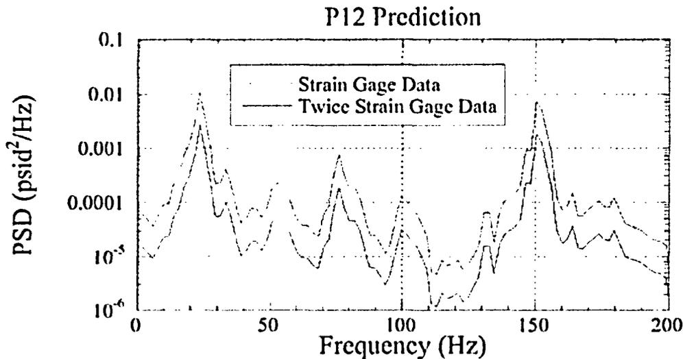
Figure EMEB-B-143-1-1: PSDs of Pressure Sensor P 12, with 1X and 2X Strain Gage Data.
