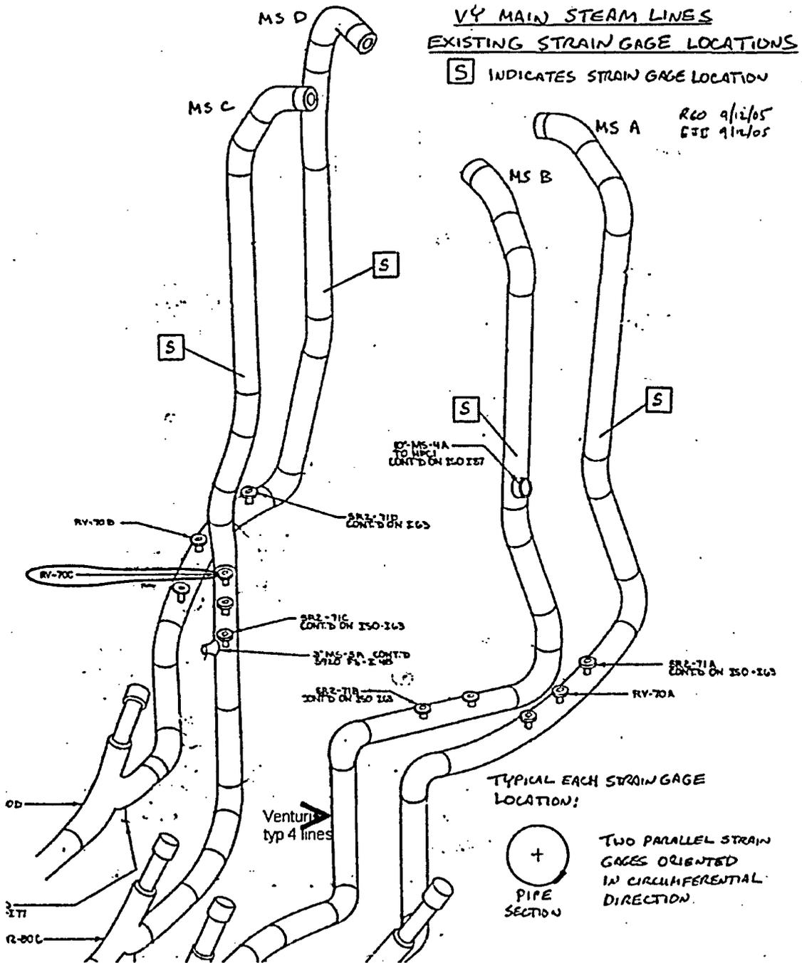
Figure EMEB-B-77-1 – Sheet 3: VYNPS Main Steam Piping Cavities and ACM Measurement Locations
