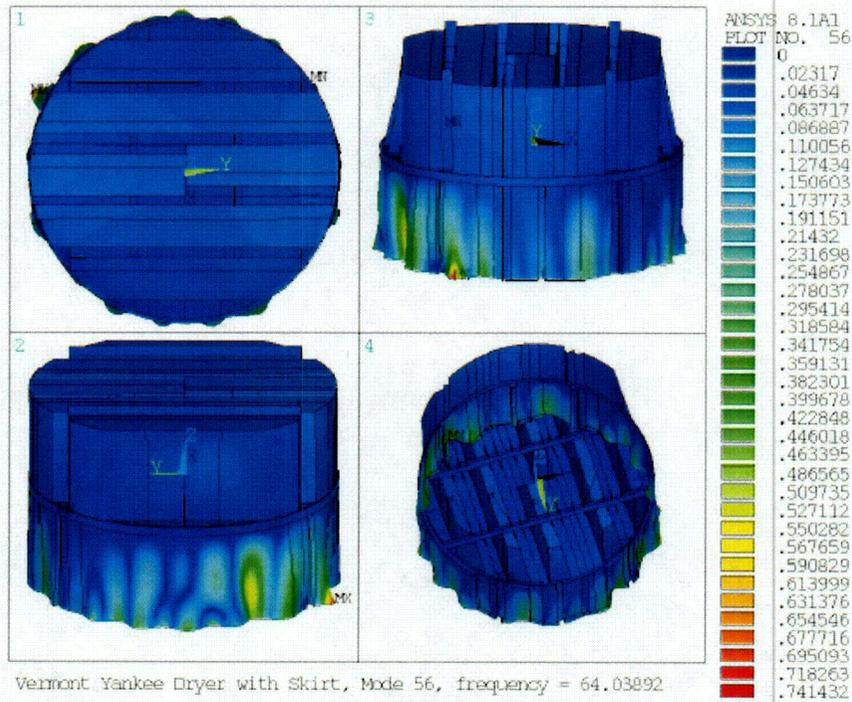
Figure EMEB-B-39-5 Dryer Model with skirt 64 Hz Mode
