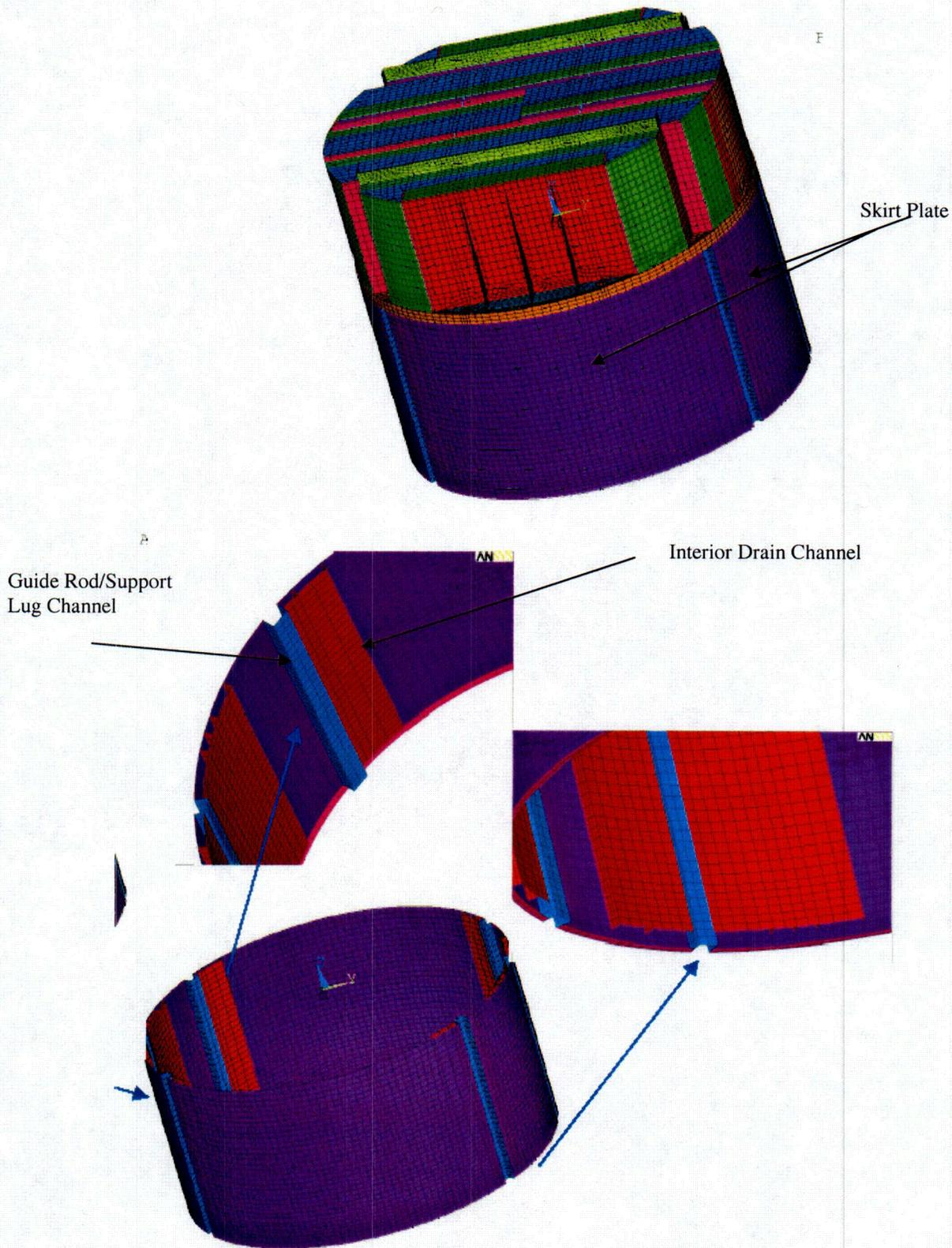
Figure EMEB-B-39-12 - VYNPS Dryer Model with skirt
