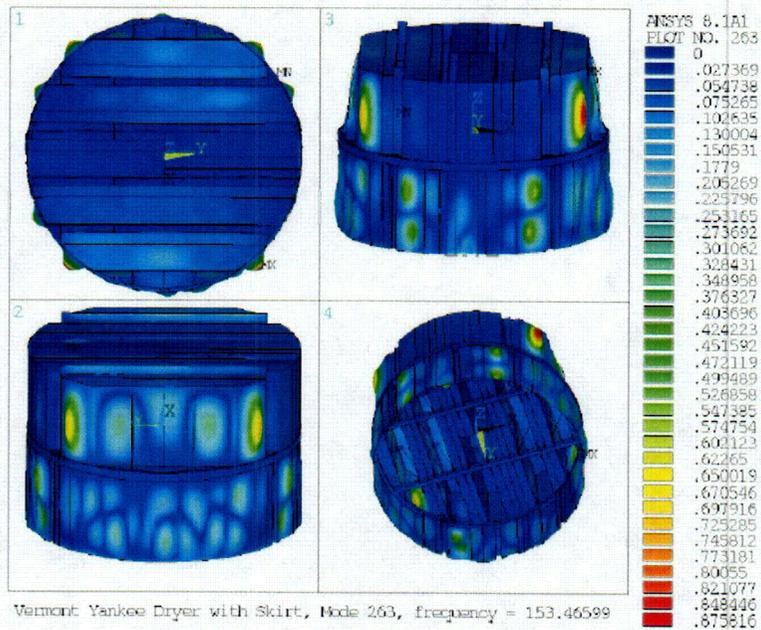
Figure EMEB-B-39-11 Dryer Model with skirt 153 Hz Mode
