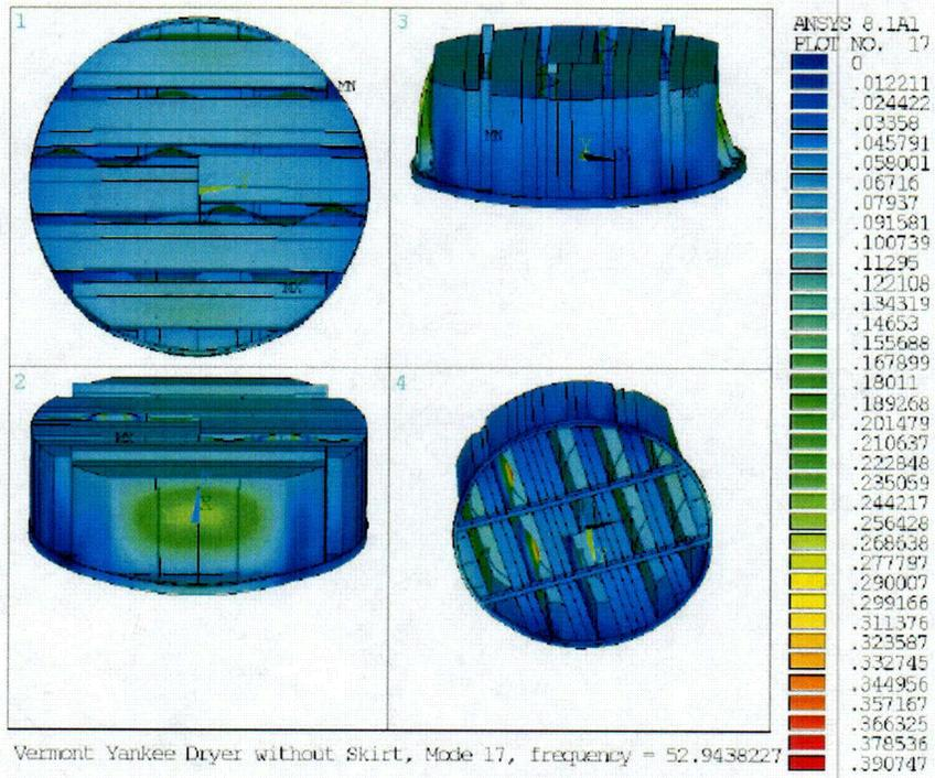
Figure EMEB-B-39-1 Dryer Model without skirt 53 Hz Mode
