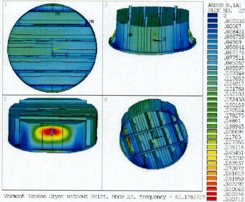
Figure EMEB-B-39-2 Dryer Model without skirt 62 Hz Mode
