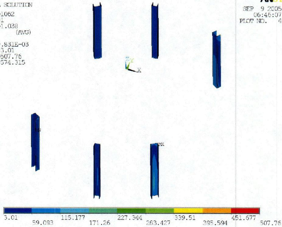
Figure EMEB-B-39-14 – Guide Rod/Support Lug Channel Peak Stress Intensity
