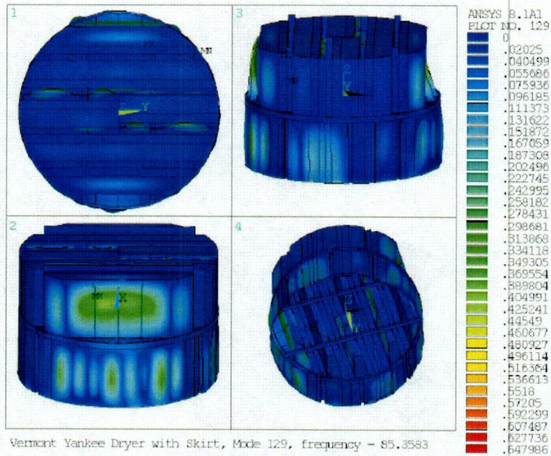
Figure EMEB-B-39-6 Dryer Model with skirt 85 Hz Mode
