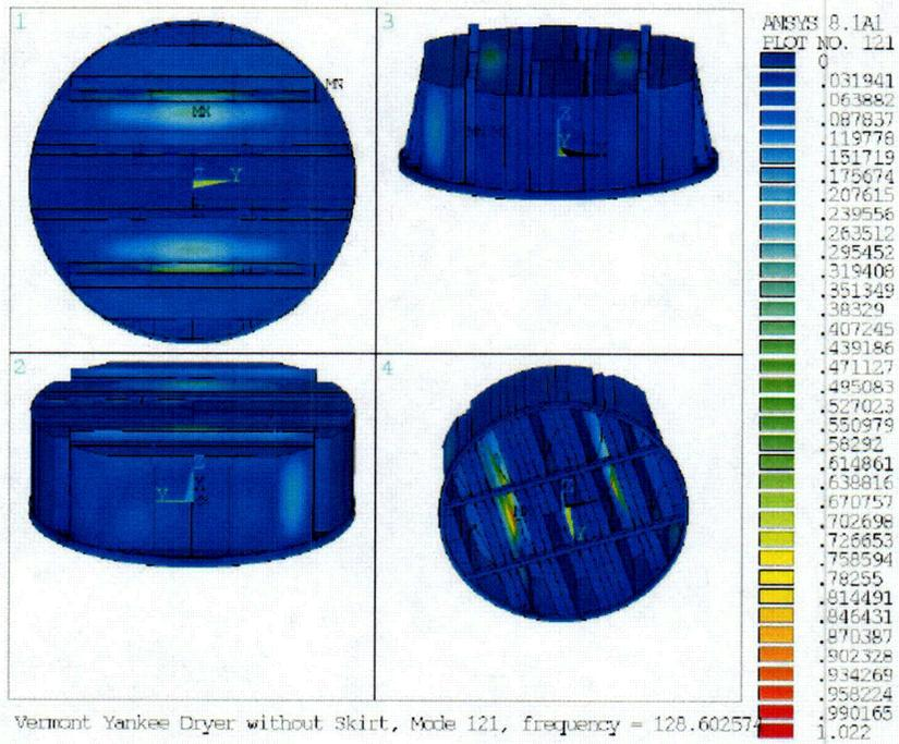
Figure EMEB-B-39-8 Dryer Model without skirt 128 Hz Mode
