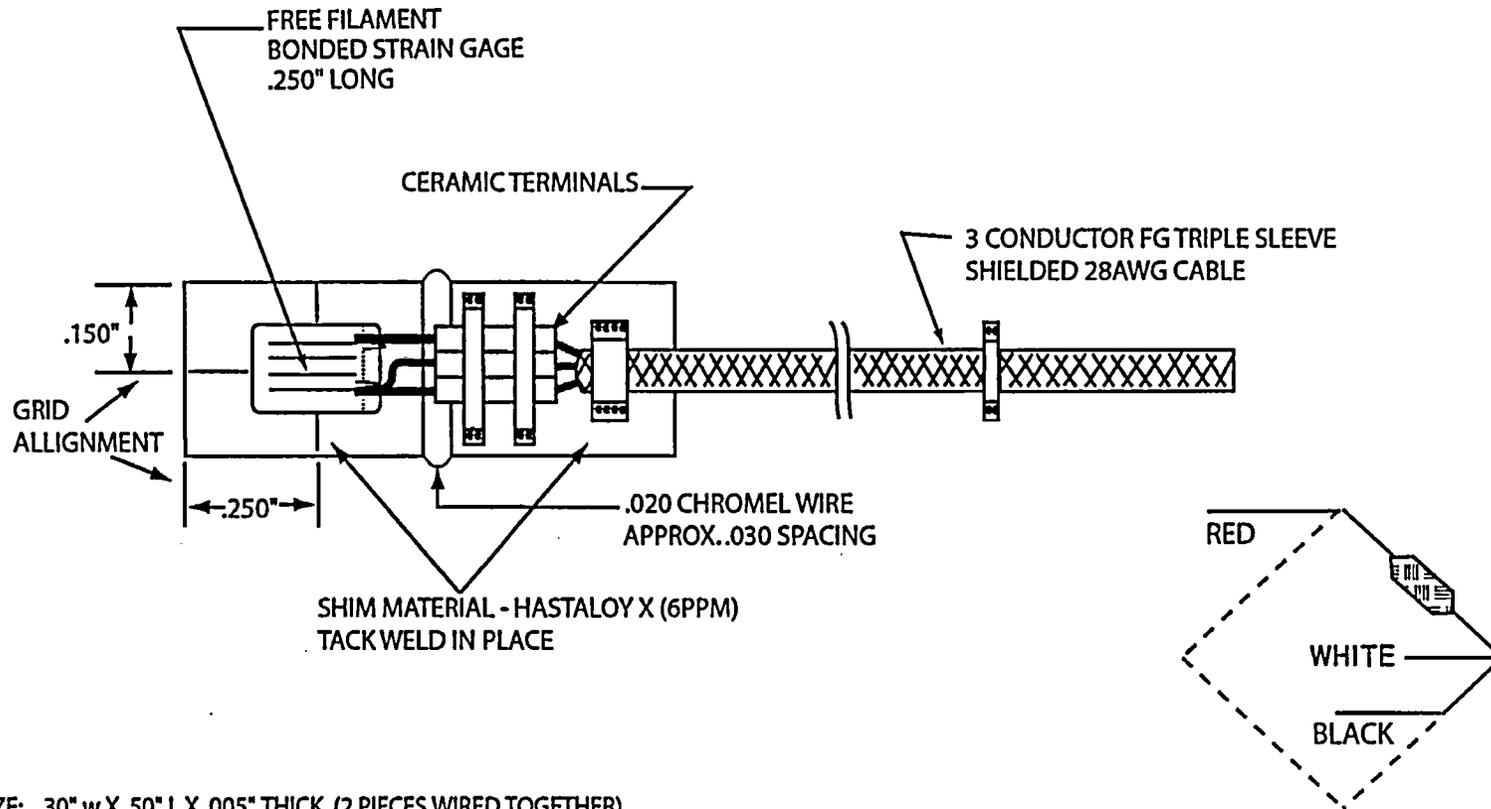
SHIM SIZE: .30" w X .50" L X .005" THICK (2 PIECES WIRED TOGETHER)
