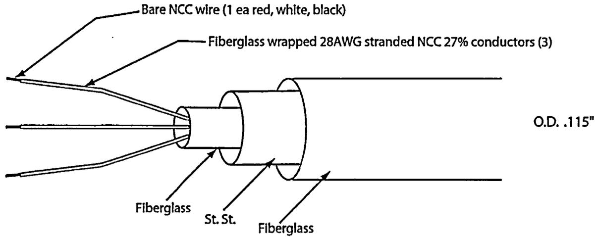
Note: Stainless steel sleeve is cut back for strain gage assembly so it does not come in contact with the metal shim.
