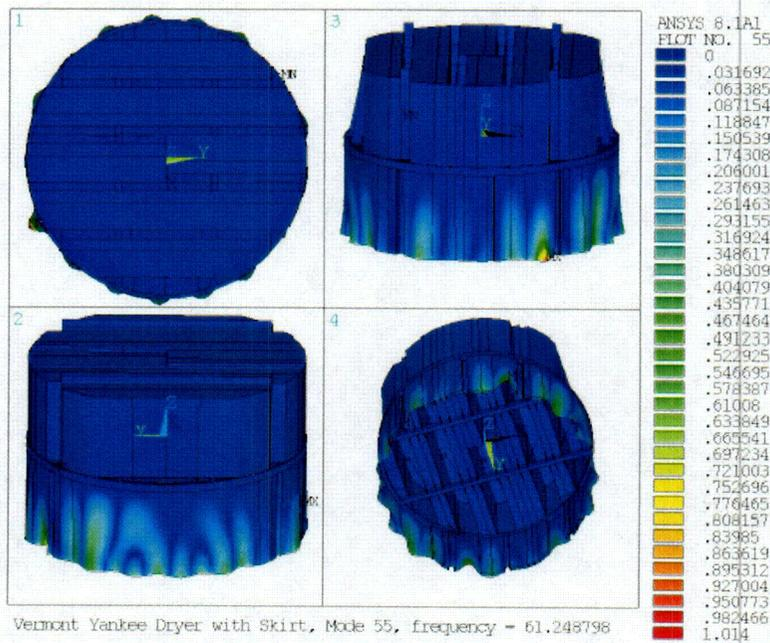
Figure EMEB-B-39-4 Dryer Model with skirt 61 Hz Mode
