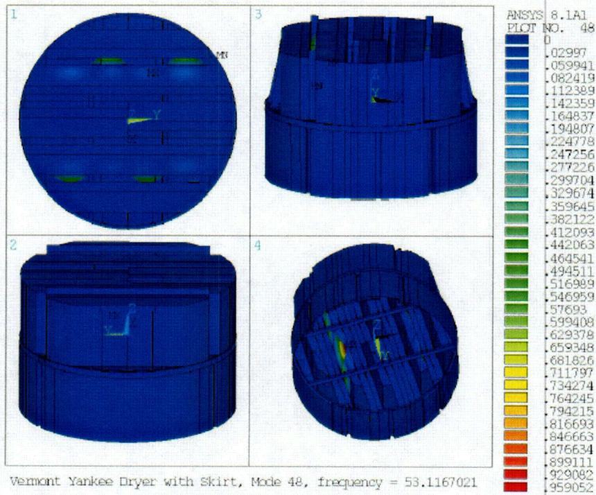
Figure EMEB-B-39-3 Dryer Model with skirt 53 Hz Mode
