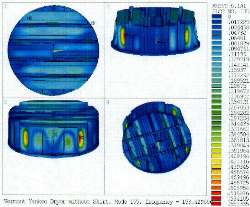
Figure EMEB-B-39-10 Dryer Model without skirt 153 Hz Mode
