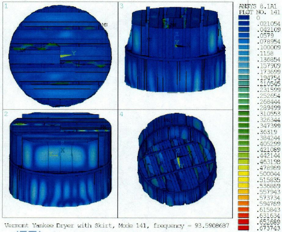
Figure EMEB-B-39-7 Dryer Model with skirt 94 Hz Mode
