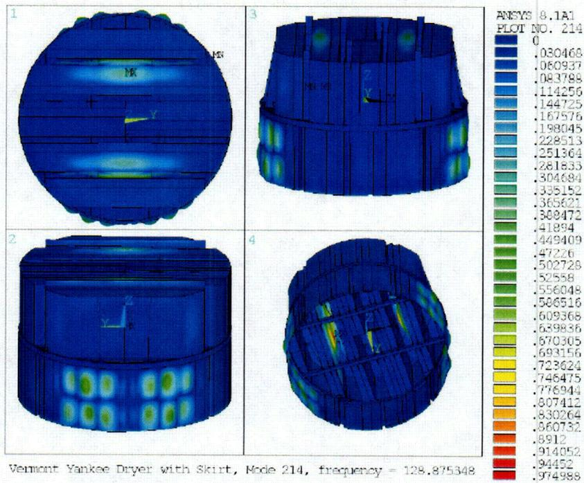
Figure EMEB-B-39-9 Dryer Model with skirt 128 Hz Mode
