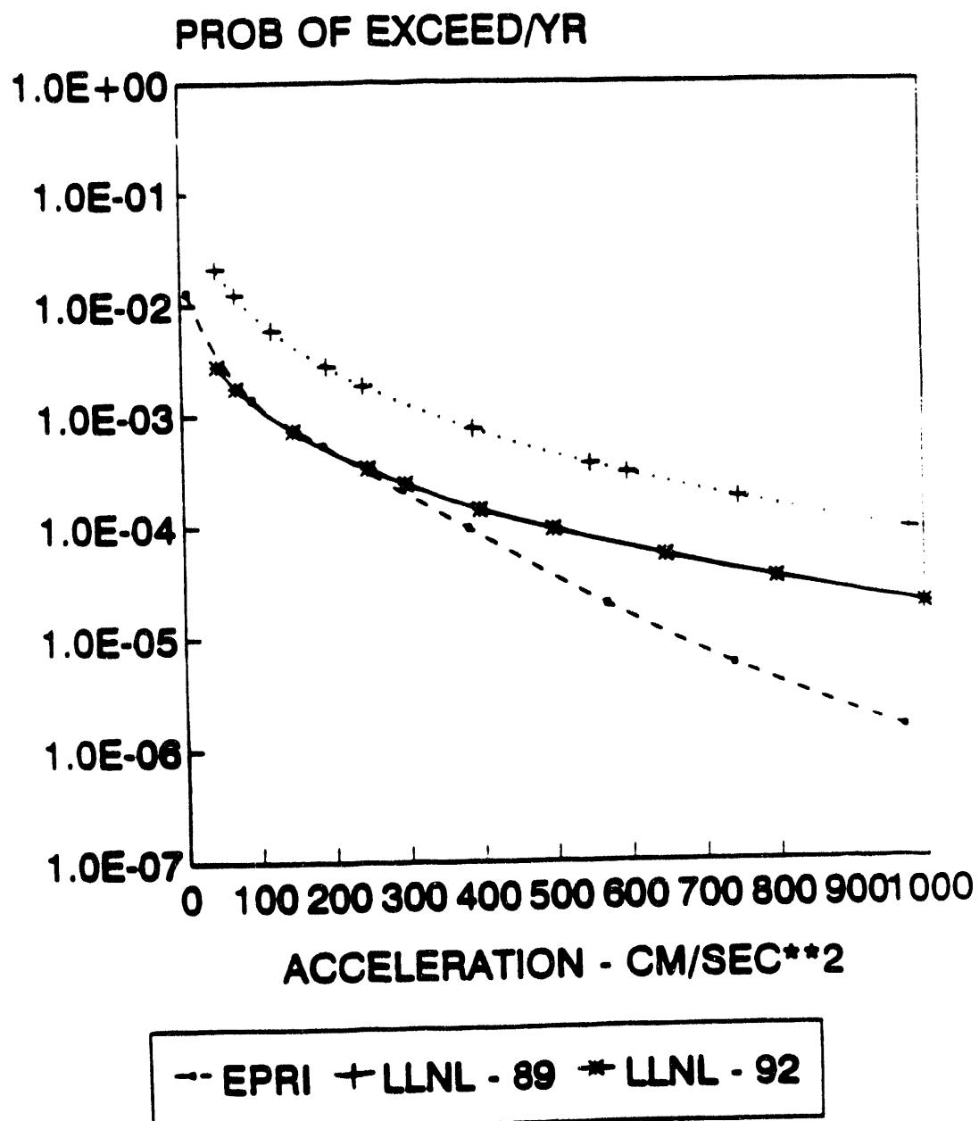
**Figure 3 - Comparison of 1989 LLNL, 1992 LLNL and EPRI estimates of probability of exceeding peak ground acceleration per year versus acceleration - Shearon Harris site.**
