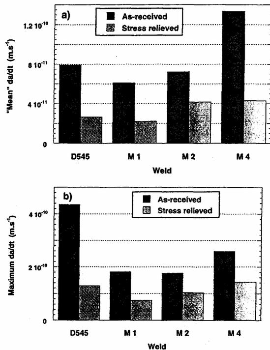
Figure 3 Effects of heat treatment on SCC susceptibility of Alloy 182 [2], results of CGR tests carried out in primary water at 330 °C and an initial  $K_I$  of 20 MPaK $\sqrt{m}$
