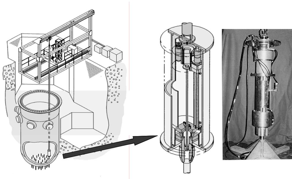
Fig.2 Concept of WJP for BMI nozzle and the system
