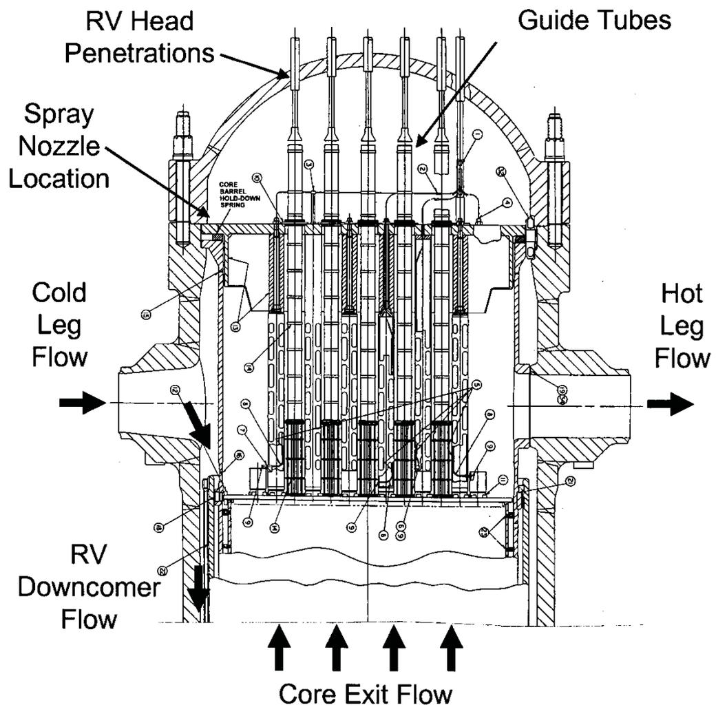
Figure 1: Upper Internals Components and Reactor Coolant Flow Paths
