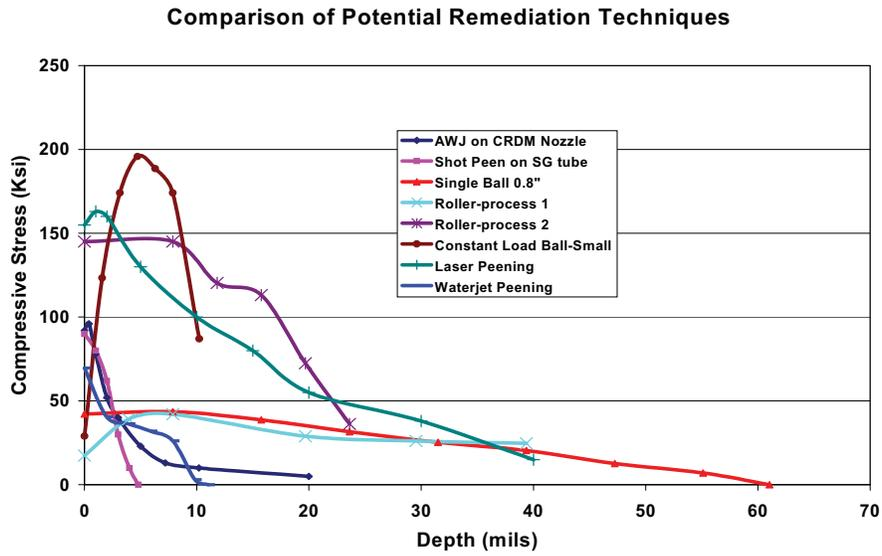
Figure 6. Typical Compressive Stress Distribution Comparison of Several Remediation Techniques.
