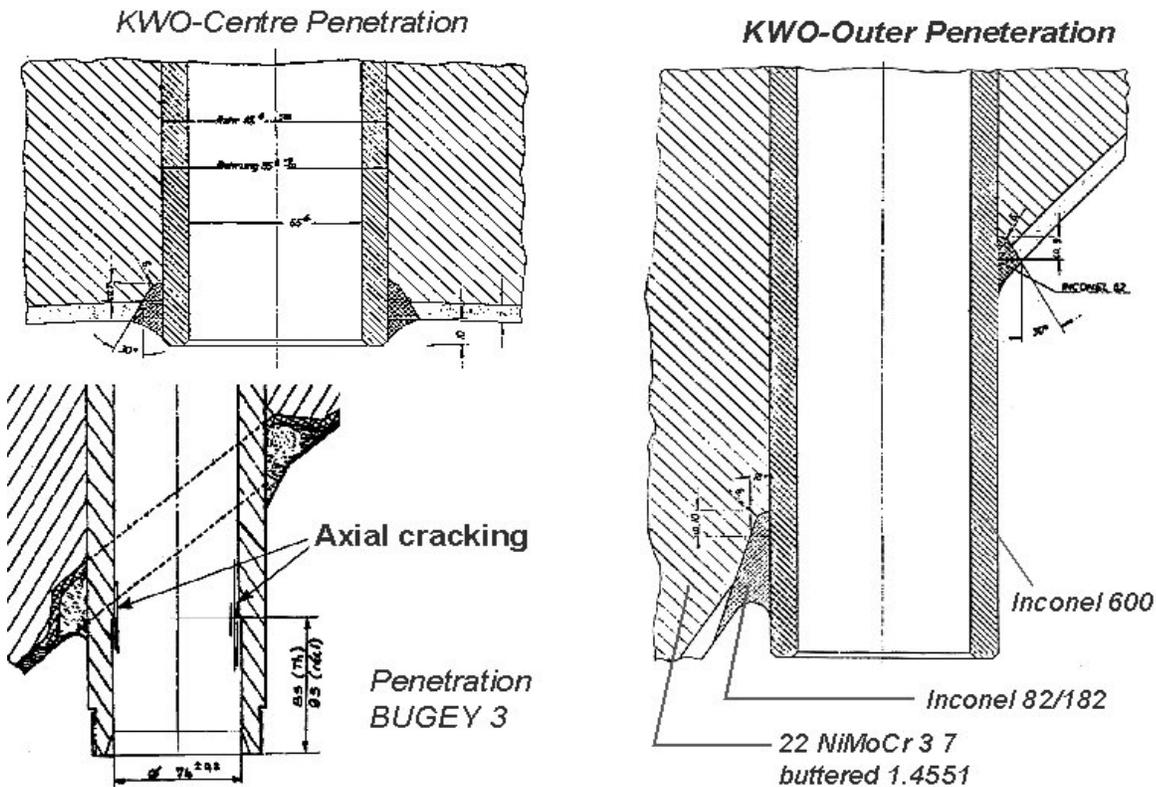
Figure 2 Weld layout at different locations of head penetrations in the RPV head
