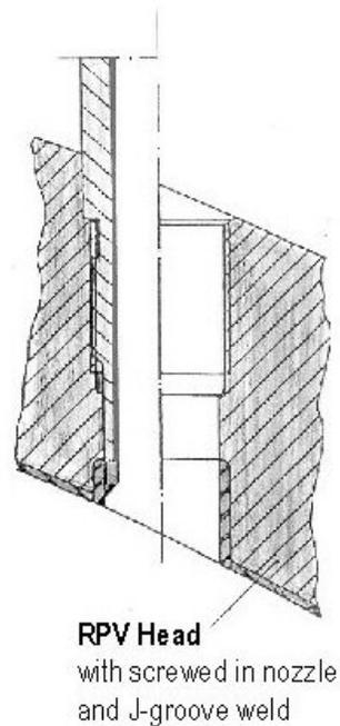
Figure 7 Section of RPV head with screwed-in and seal welded nozzle end
