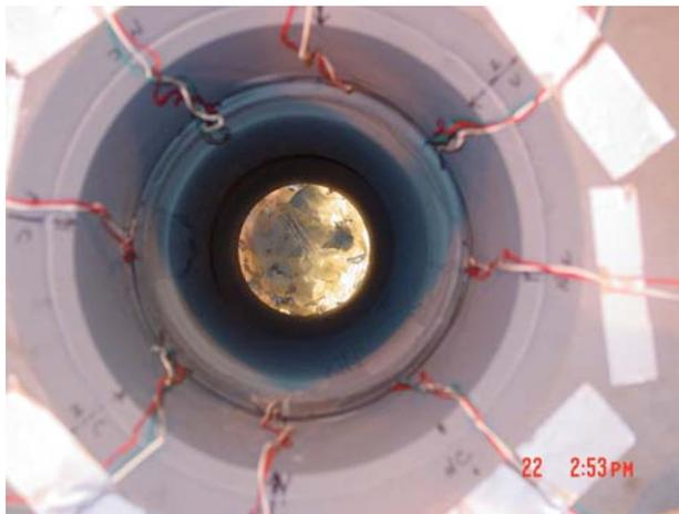
**Figure 4(a) Illustration of the Instrumented Strain Gauges Installed on the ID Surface Near the Weld Location of the Mockup Pressurizer Nozzle**
