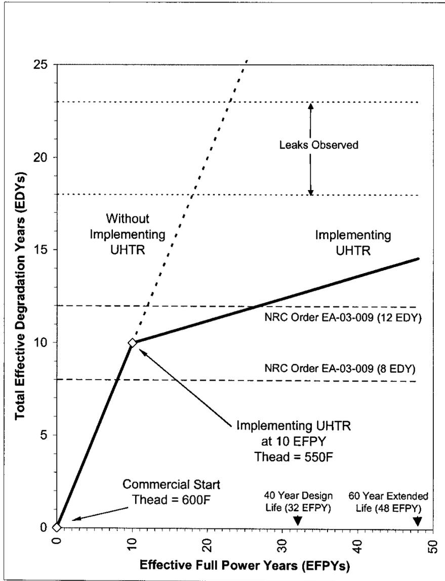
Figure 5: Example of UHTR Effectiveness for a Unit Approaching the 12 EDY Limit (with Respect to NRC Order EA-03-009)
