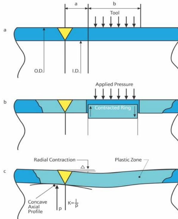
Figure 1 - Schematic Illustration of MSIP Process
