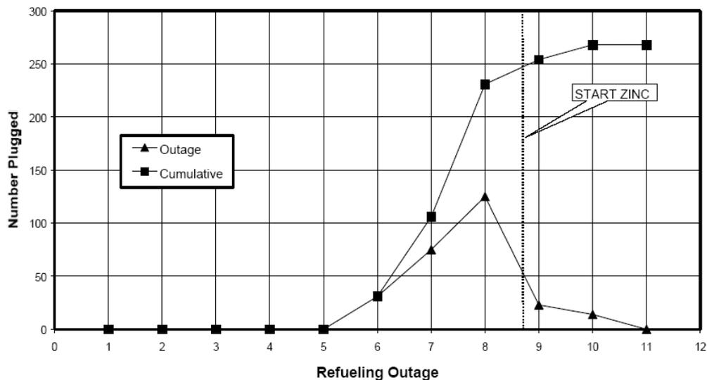
**Figure 6** Example of field data from Diablo Canyon Unit 1: plugging for PWSCC at tube-support-plate (TSP) locations
