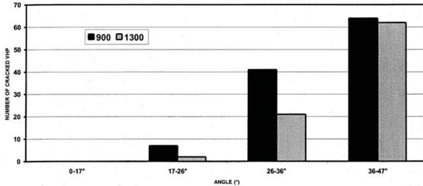
Fig. 5 : Importance of the “angle effect” versus VH penetrations cracking
