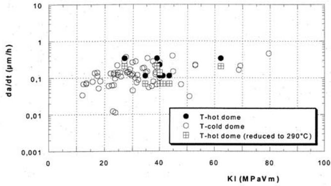
Fig 2 : Field data - T-hot dome data (300°C) reduced to 290°C with  $Q = 130$  KJ/mol and T-cold dome data (290°C)
