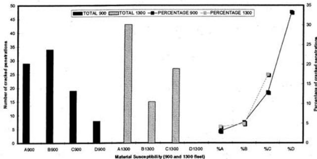
Fig 6 : Importance of the material susceptibility versus VH penetrations cracking (percentage values are given versus the total number of penetrations in standardized plant series 900 or 1300)
