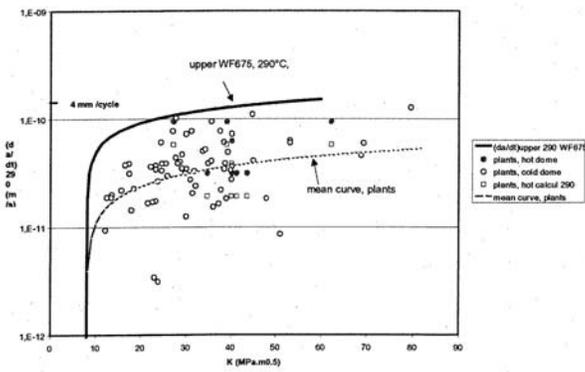
Fig. 3 : Comparison between laboratory and field experience
