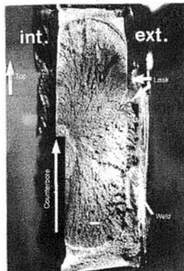
Fig. 1: TWE crack in T54 VH penetration
