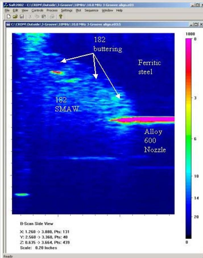
Normal incidence using 10MHz spherically focused, F8
