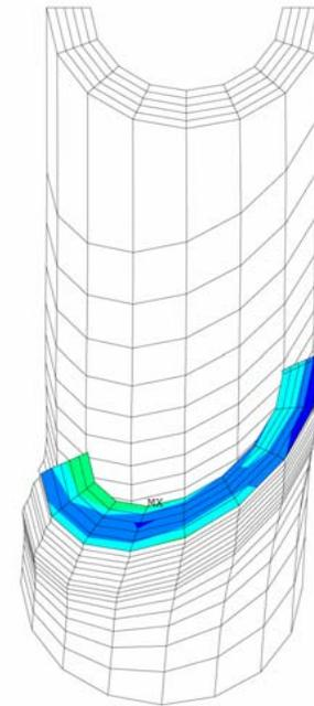
**Example of Operating Stress Perpendicular to Circ Crack Plane**
