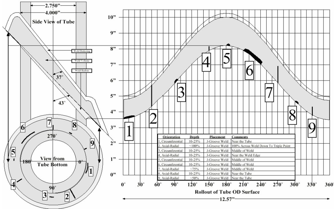
NOTE: Flaw locations and sizes are shown only to describe typical types of flaws to be included in blind mockups. Actual flaw sizes and locations are confidential. Drawing is not to scale.
