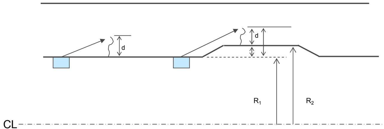
Profiling techniques can improve accuracy of depth sizing when the probe is not on the same surface as the crack
