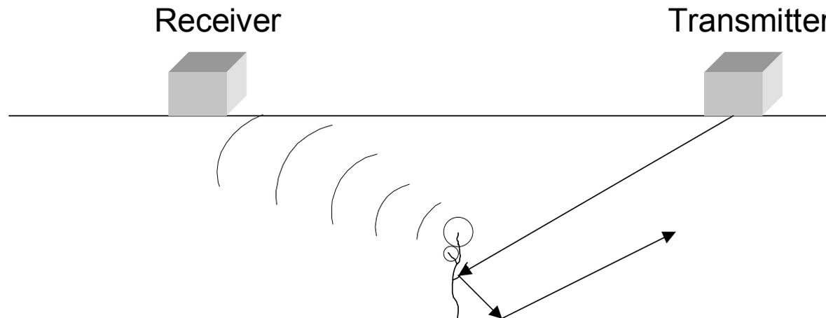
Low-amplitude, secondary wave generated by excitation of flaw
