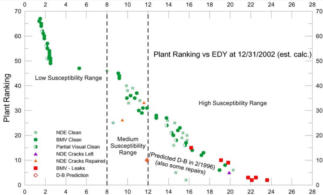
Figure 1. Ranking of domestic plants according to the EDY formula, showing results of inspections, evidence of leakage, and repairs. Many plants are shown with multiple symbols, indicating a “clean” inspection at inspection opportunity, followed by a different finding at a subsequent inspection (e.g., Oconee 2: clean NDE @ EDY=15.7, leaks and circ. flaws @ 22.1)
