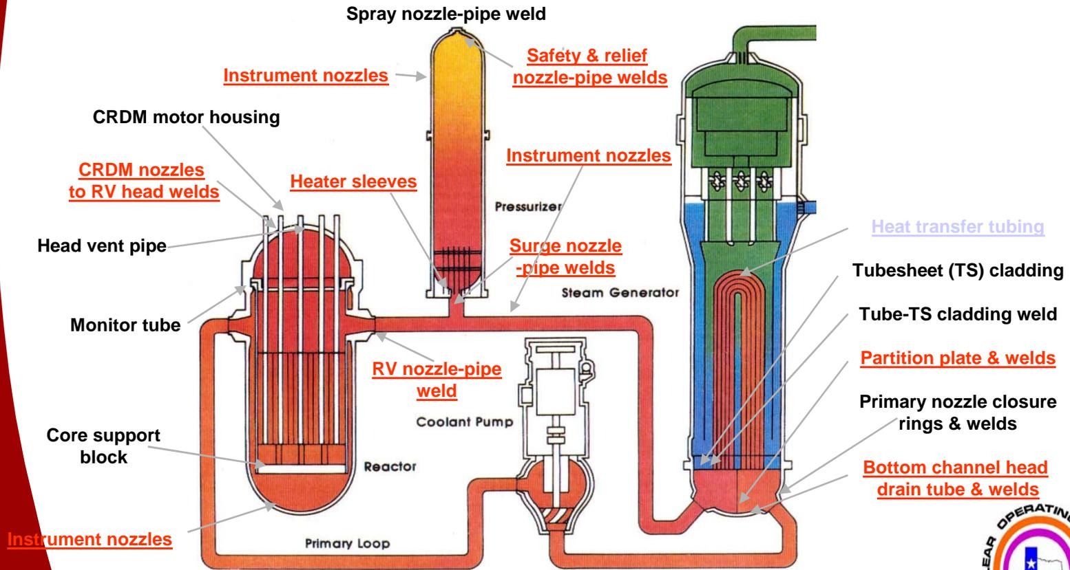
\* Represents locations that have experienced cracking and or leakage at other PWRs are highlighted in red.
