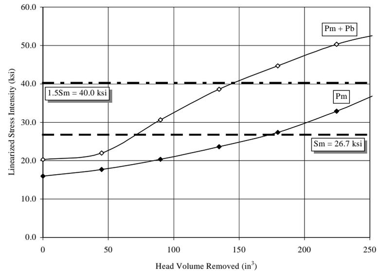
**Primary Membrane and Membrane Plus Bending Stress as Function of Wastage Volume**
