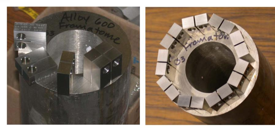
Considered various orientations; chose orientation at right, designated C-L Approximate representation of specimen removal at mid-wall position
