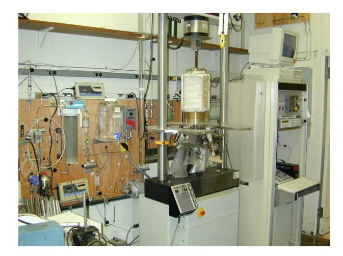
Fully instrumented high temp. water SCC systems, incorporating water supply, autoclave, digital load control, digital temp. control, data acquisition...
