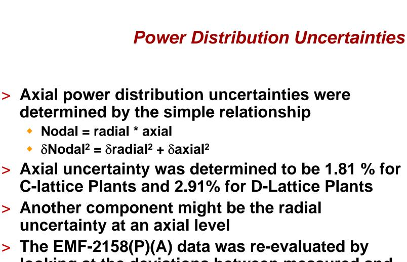
looking at the deviations between measured and calculated TIP response for each axial level
