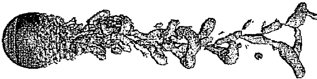
Figure 6. Vortical structure in the near-wake of the sphere for Re_D = 1.14 \times 10^6 - visualized using the iso-contour of the second-invariant of the velocity deformation tensor
