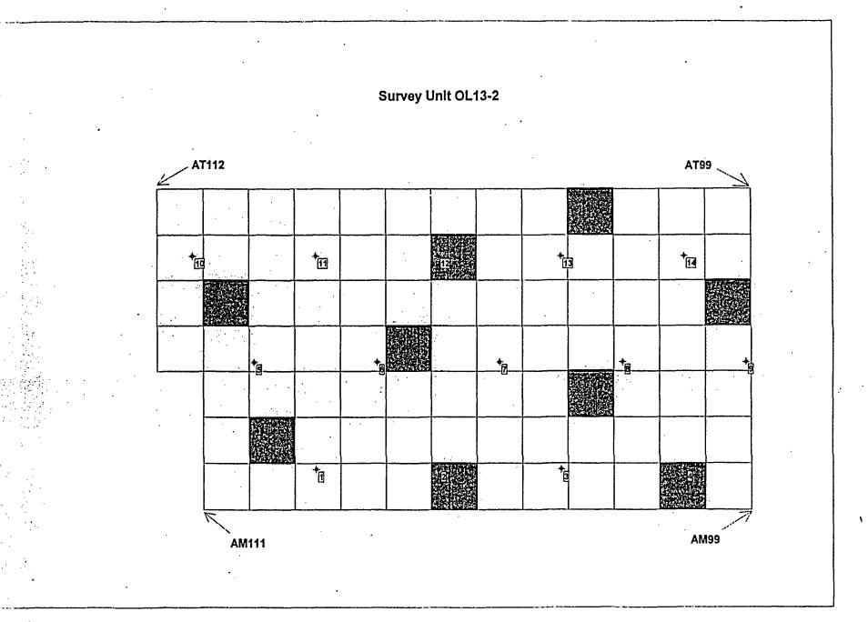
Soil Sample Locations and Scan Survey Grids for Survey Unit OL13-2
