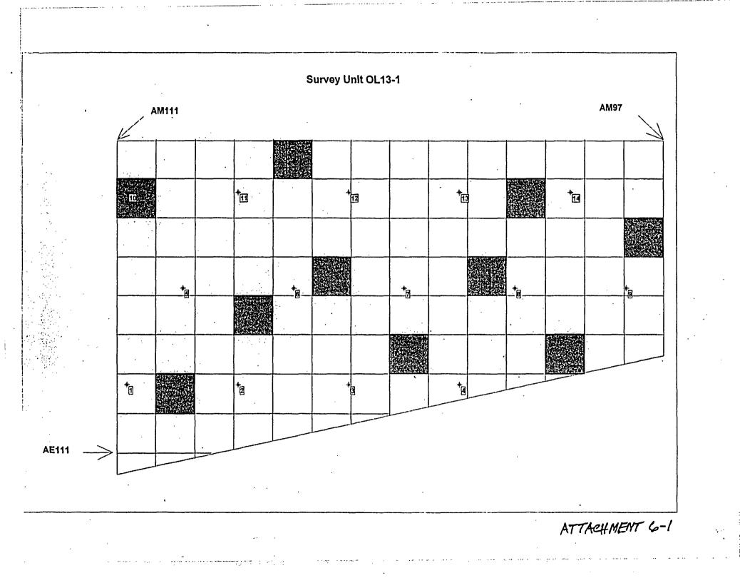
Soil Sample Locations and Scan Survey Grids for Survey Unit OL13-1
