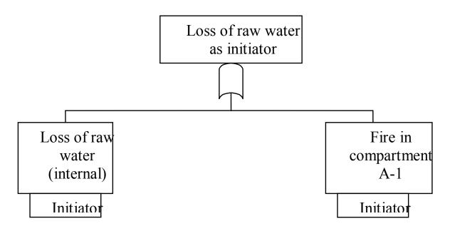
Example of new logic with a fireinduced loss of raw water initiating event
