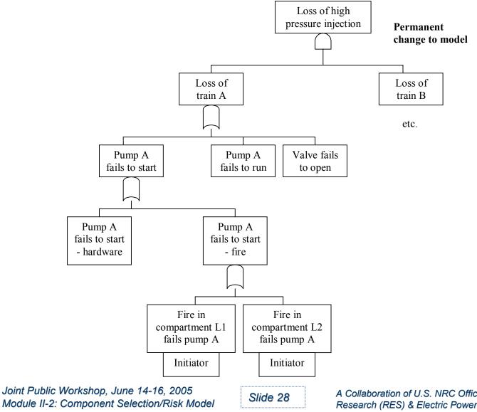
Step 1.3 (2.3): Incorporate fire-induced human failures
