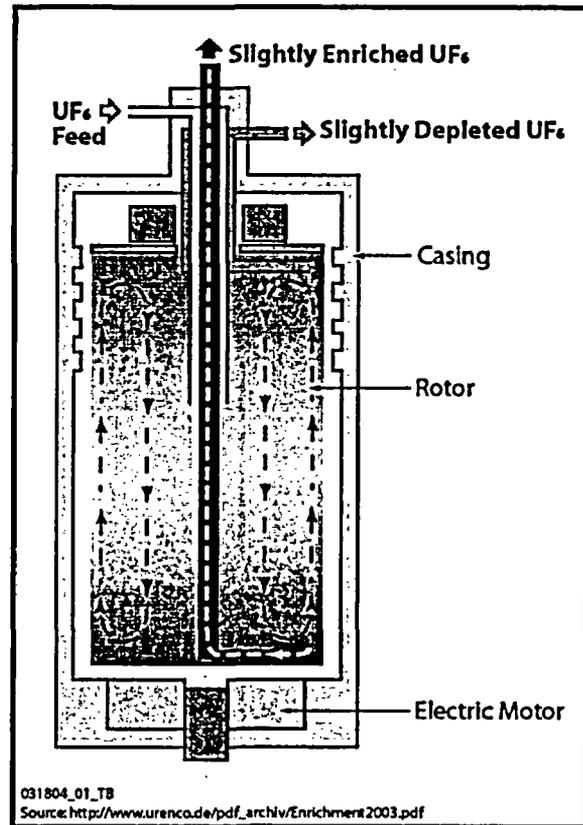
**Figure 2-2 Schematic of a Gas Centrifuge (Urenco, 2003)**
