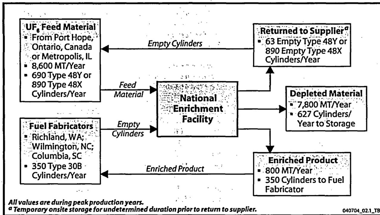
Figure 2-9 Flow from Feed, Enriched, and DUF<sub>6</sub> Material
