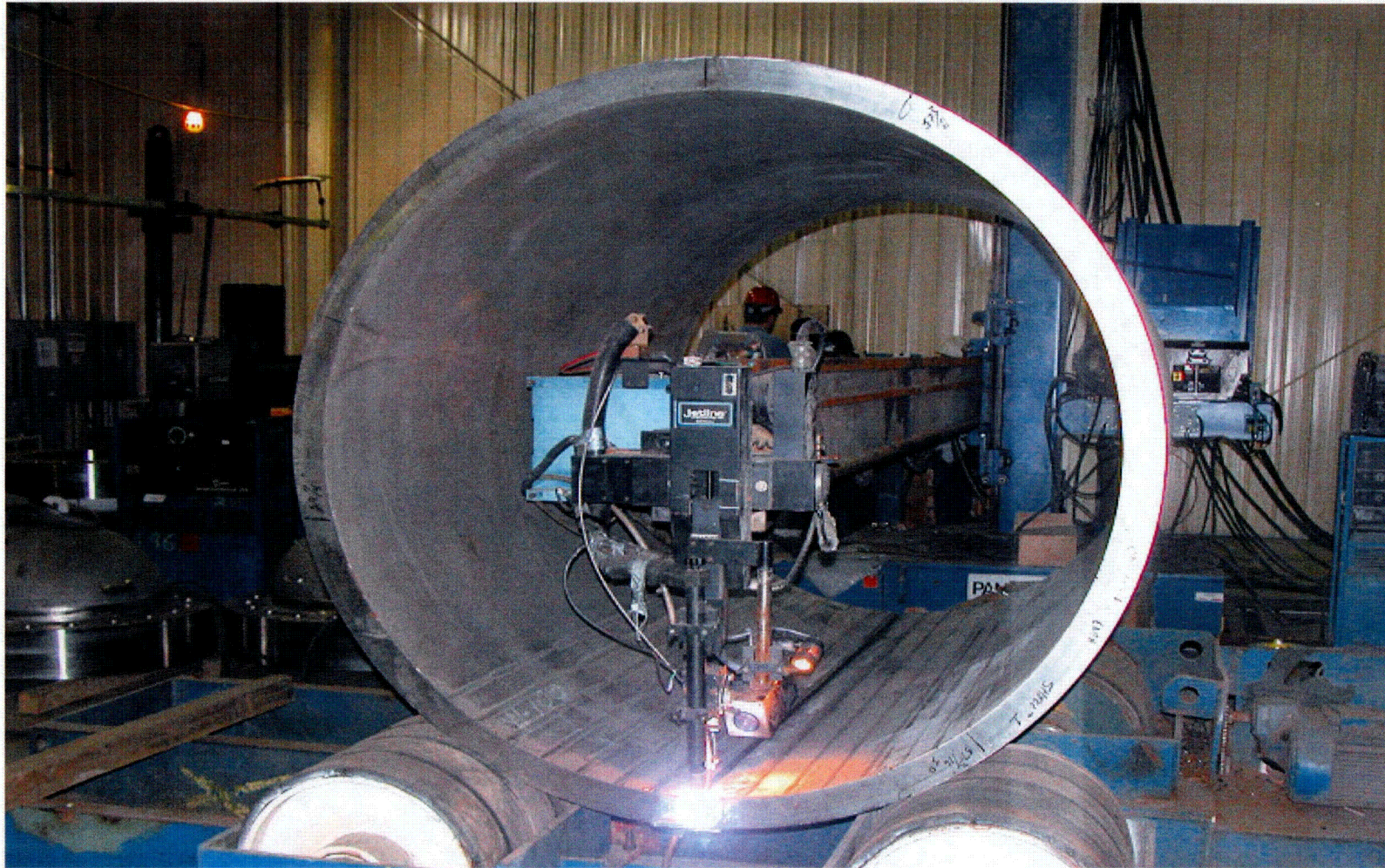
Longitudinal seam welding on the 316 stainless steel inner vessel
