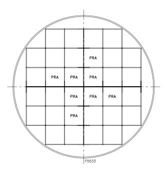
Figure 1-6 Required PRA Locations for the NUHOMS  $^{\tiny @}$  -32PT DSC Configuration with Eight PRAs
