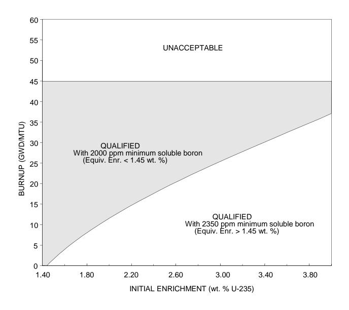
Figure 1-1 PWR Fuel Criticality Acceptance Curve
