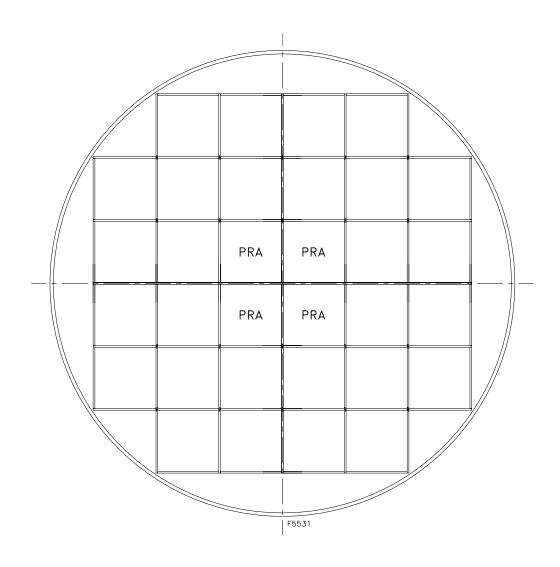
$\label{eq:Figure 1-5} Figure \ 1-5$  Required PRA Locations for the NUHOMS  $^{\tiny @}$  -32PT DSC Configuration with Four PRAs
