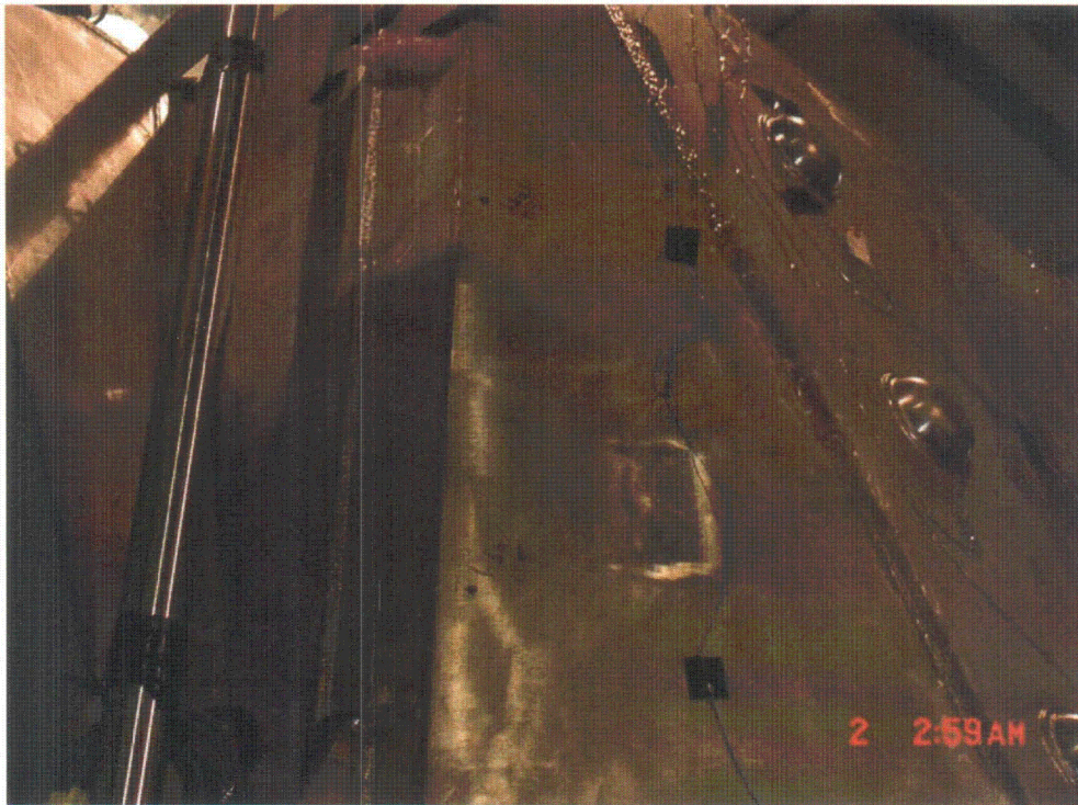
Figure 17: Response locations on side panel to the left of main panel of 90 degree hood of dryer #1 (at angle w.r.t. main panel).
