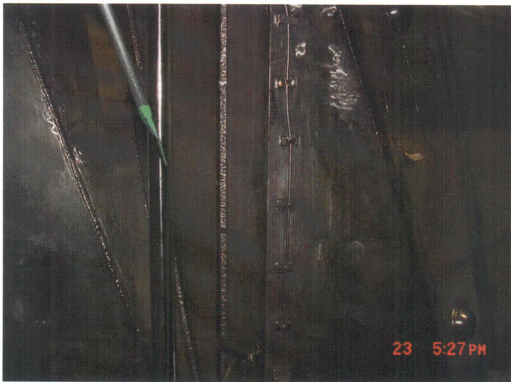
Figure 24: Response locations on side panel to the left of main panel of 270 degree hood of dryer #1 (at angle w.r.t. main panel).
