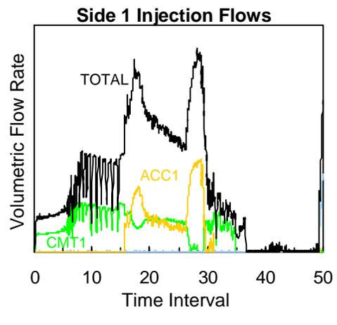
Figure 3.3 Test NRC-AP1000-06 passive safety system performance.
