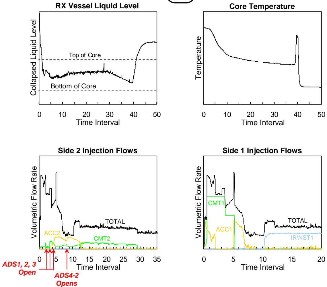
Figure 3.2 Test NRC-AP1000-05 passive safety system performance.
