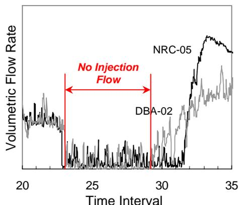
Figure 4.2 Total injection flow rate: ACCs, CMTs, and IRWST2.
