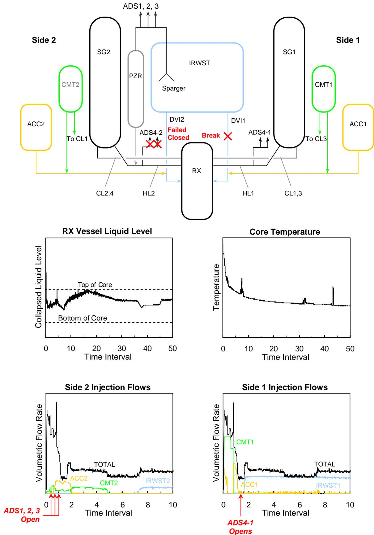
Figure 3.1 Test NRC-AP1000-03 passive safety system performance.
