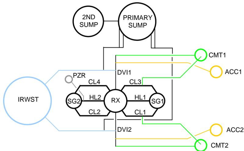
Figure 2.1 APEX-AP1000 Test Facility (Plan View)
