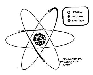
Figure 1: An atom consists of two parts: a nucleus containing positively charged protons and electrically neutral neutrons and one or more negatively charged electrons orbiting the nucleus. Protons and neutrons are nearly identical in size and weight, while each is about 2000 times heavier than an electron.
