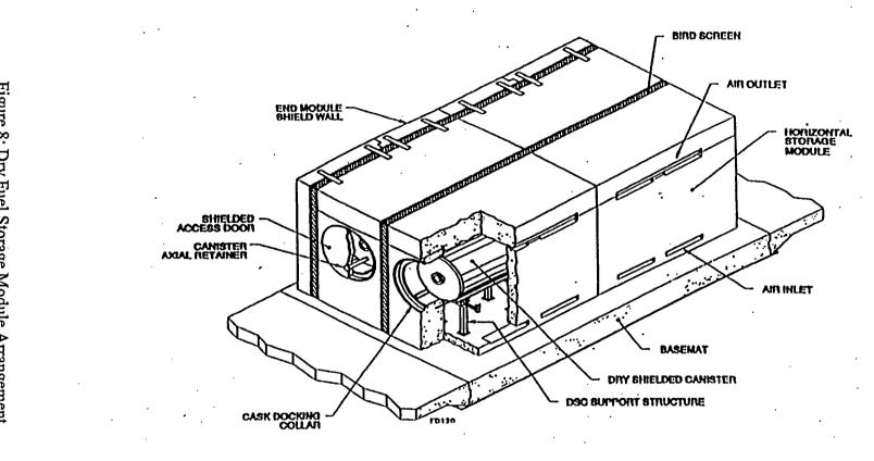
Figure 8: Dry Fuel Storage Module Arrangement
