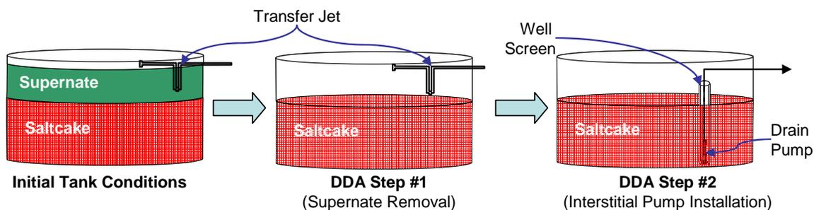
The first step in the deliquification phase (Figure 2.3, Step 1) is to remove the free supernate stored above the saltcake surface. Removal of the free supernate will generally be done using the existing tank transfer jet in each tank undergoing the DDA process. The free supernate will be transferred to another Tank Farm waste tank where it will be held for future treatment at SWPF.
