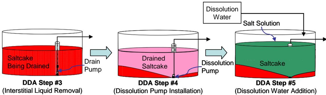
After interstitial liquid has been extracted to the point that the well recharge rate has become too slow to support the efficient removal of interstitial liquid, it is expected that approximately the bottom five feet of saltcake will remain fully saturated and approximately 50% of the interstitial liquid will have been extracted from the remainder of the saltcake, based on Tank 41 operational experience [8].
