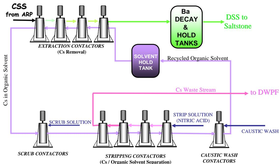
The extraction section will use the organic solvent to extract Cs (as well as some sodium and potassium) from the salt solution. The scrub section will then return the sodium and potassium to the salt solution leaving the Cs in the solvent and will neutralize any hydroxide carried over in the solvent. The strip section will return the Cs to a separate aqueous phase that will be sent to DWPF for vitrification and will allow the solvent to be reused in the process.
