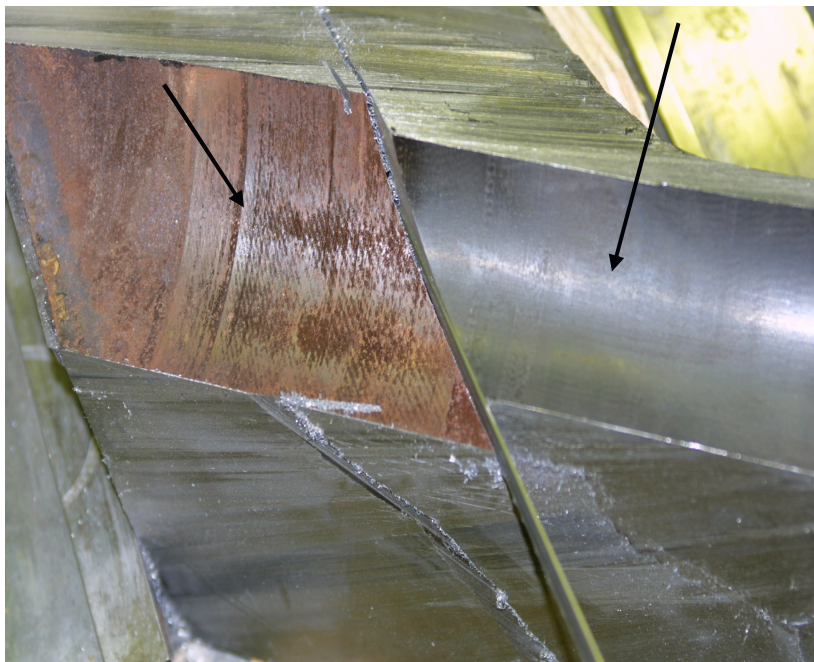
Piece B during Cutting Operation, Part of Penetration Removed
